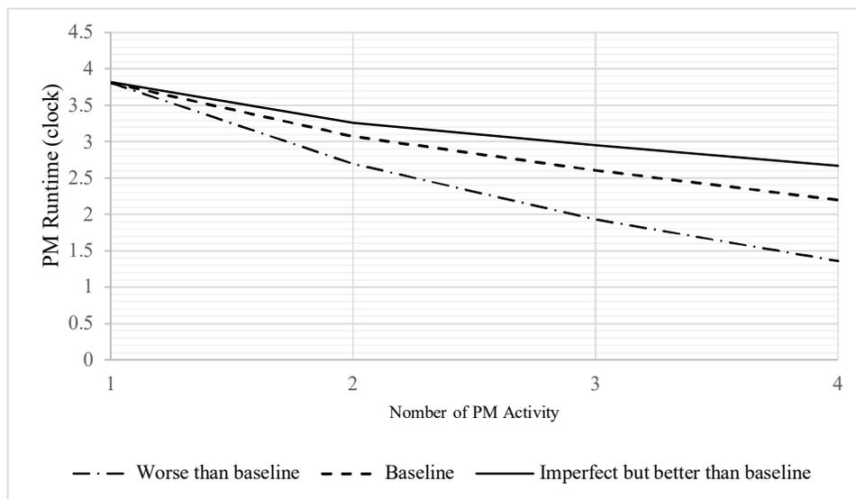
Figure 4: Execution times of PM for various effects of imperfect maintenance.
