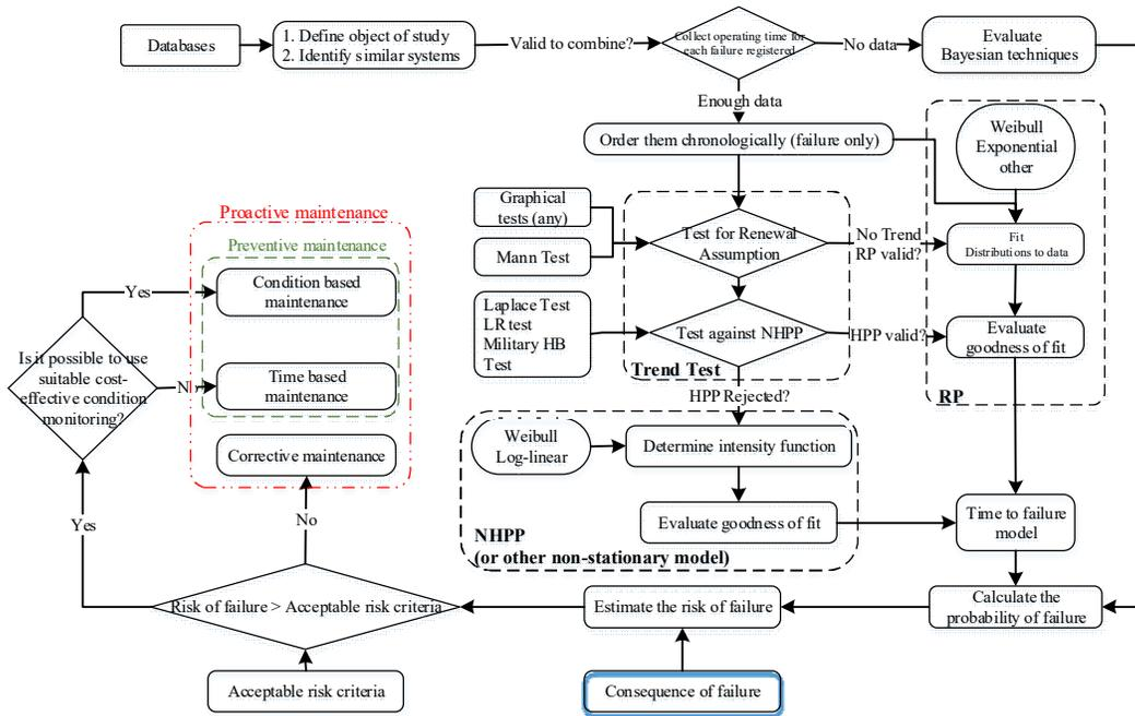
Figure 1: Methodology of reliability-based maintenance plan selection [39].
