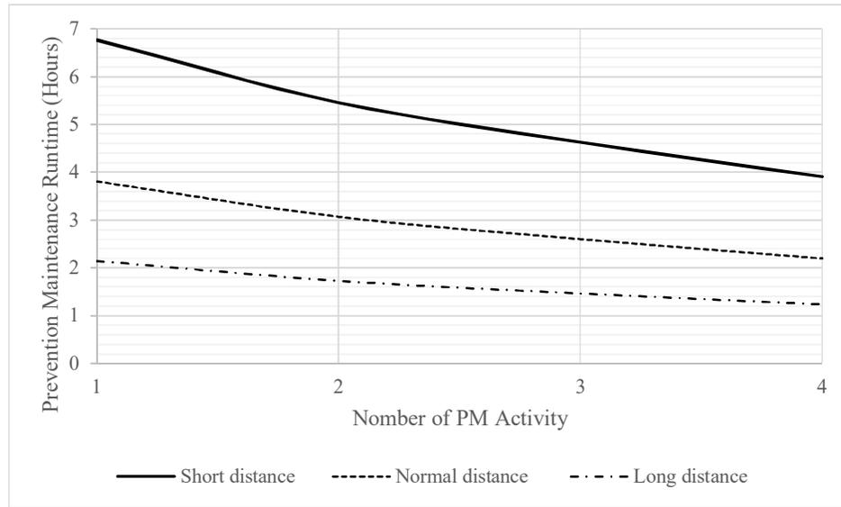
Figure 3: Preventive maintenance times in different environmental conditions.
