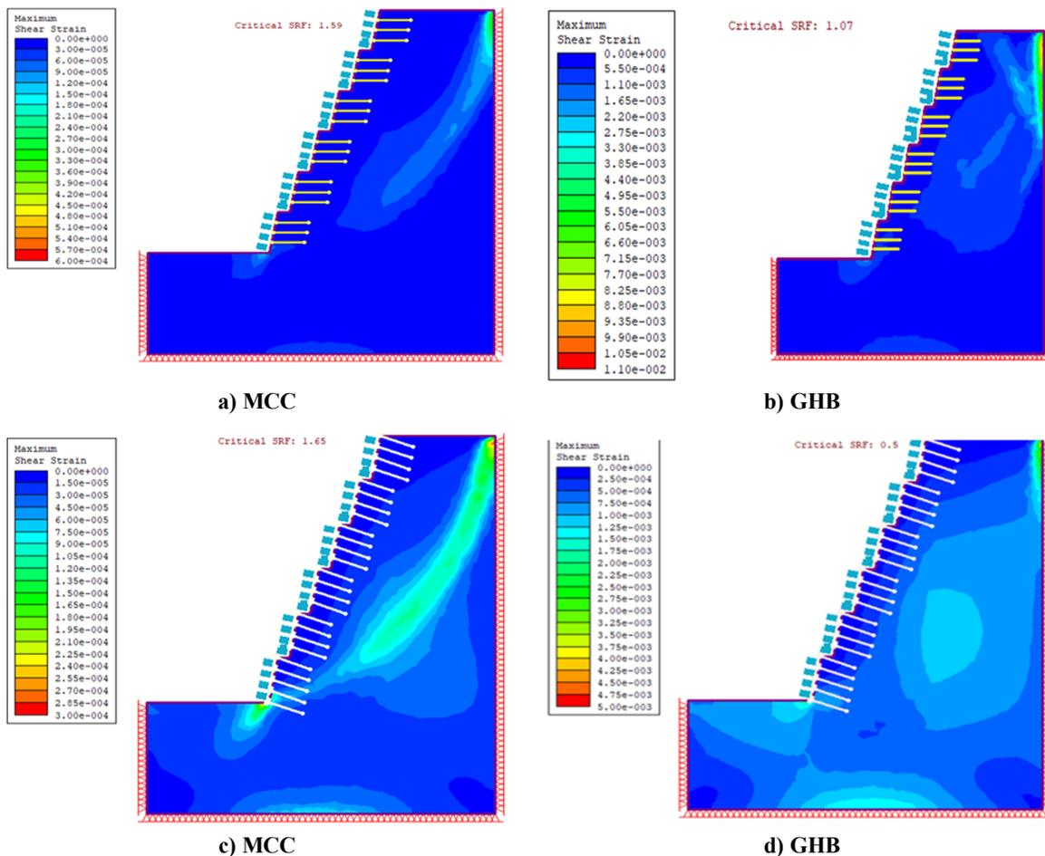
**Figure 5. a) Represents Case-I CSRF based on MCC, b) Represents Case-I CSRF based on GHB, c) Represents Case-II CSRF based on MCC, d) Represents Case-II CSRF based on GHB.**
