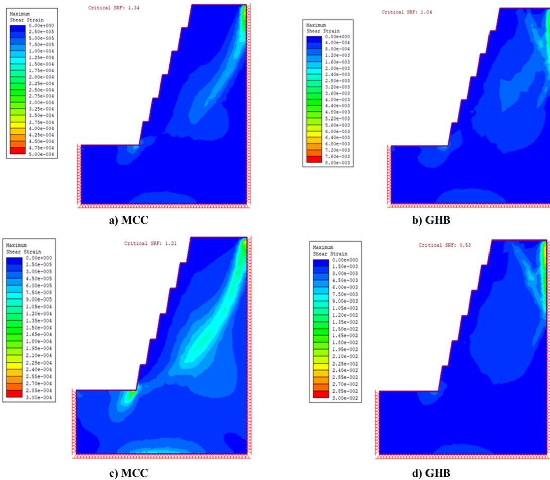
Figure 4. a) Represents Case-I CSRF based on MCC, b) Represents Case-I CSRF based on GHB, c) Represents Case-II CSRF based on MCC, d) Represents Case-II CSRF based on GHB.
