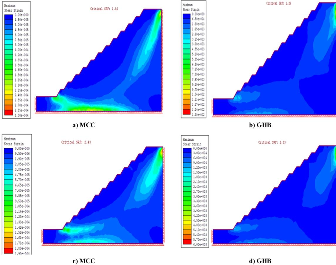
Figure 6. a) Represents Case-I CSRF based on MCC, b) Represents Case-I CSRF based on GHB, c) Represents Case-II CSRF based on MCC, d) Represents Case-II CSRF based on GHB.
