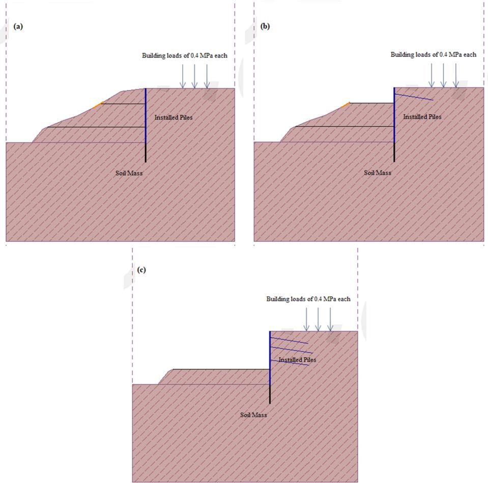
Figure 6. Steps involved in section A1-A1', (a) installation of pile, (b) and (c) installation of anchors
