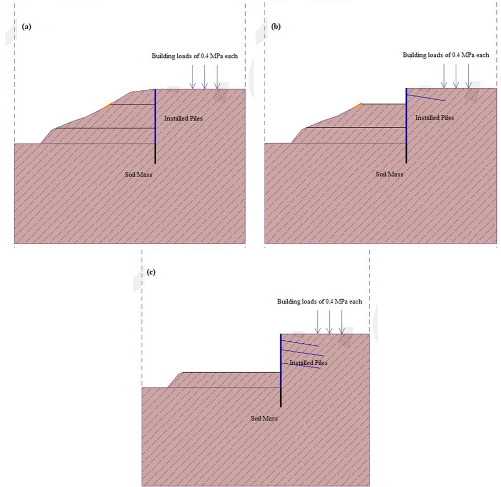
Figure 6. Steps involved in section A1-A1', (a) installation of pile, (b) and (c) installation of anchors
