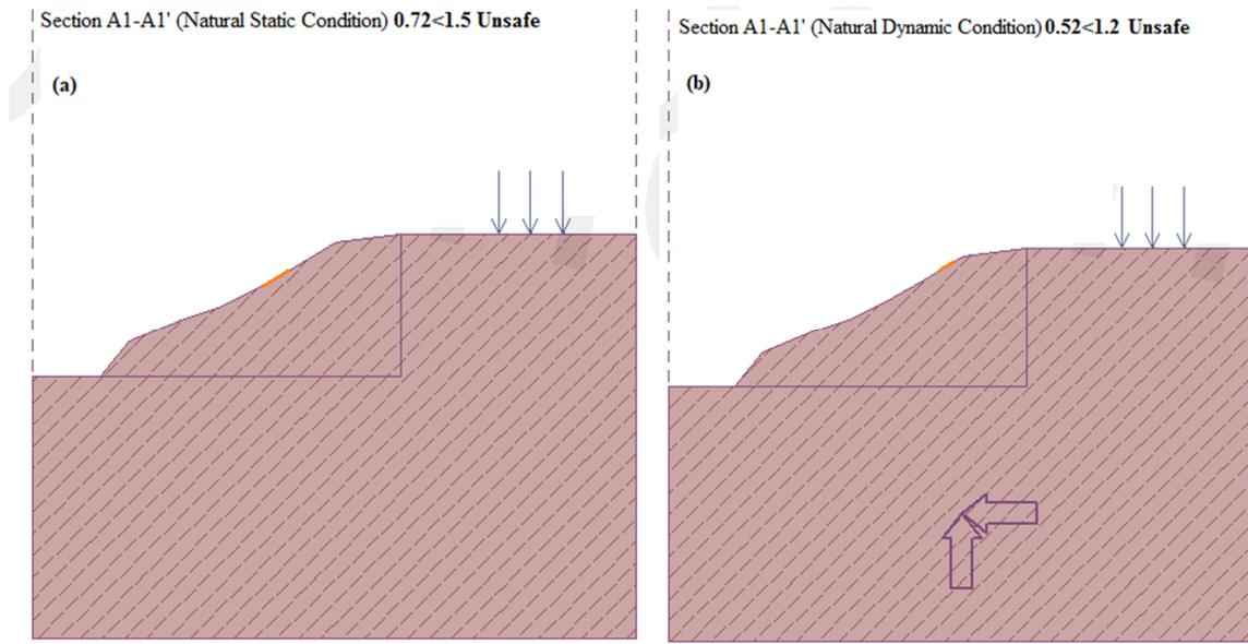
Figure 5. Section A<sub>1</sub>-A<sub>1</sub>' FOS at (a) static and (b) dynamic condition.
