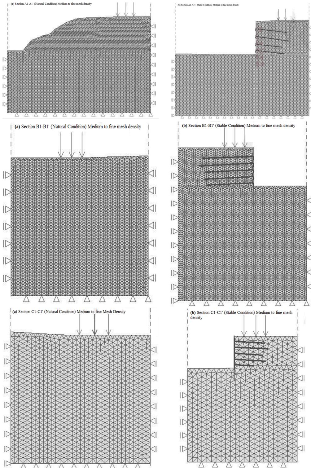
Figure 4. Finite element model for all sections from medium to fine mesh density.
