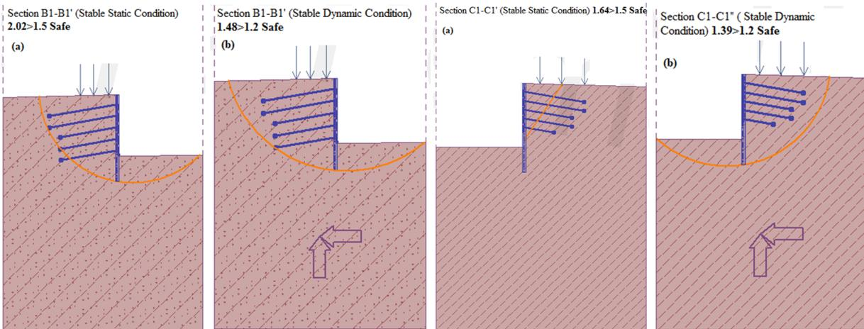
Figure 10. Stability check after remedies (a) stable static condition, (b) stable dynamic condition.
