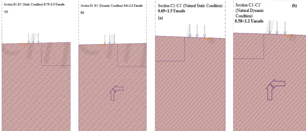
**Figure 8. Section B<sub>1</sub>-B<sub>1</sub>' and C<sub>1</sub>-C<sub>1</sub>', FOS at (a) static and (b) dynamic condition.**
