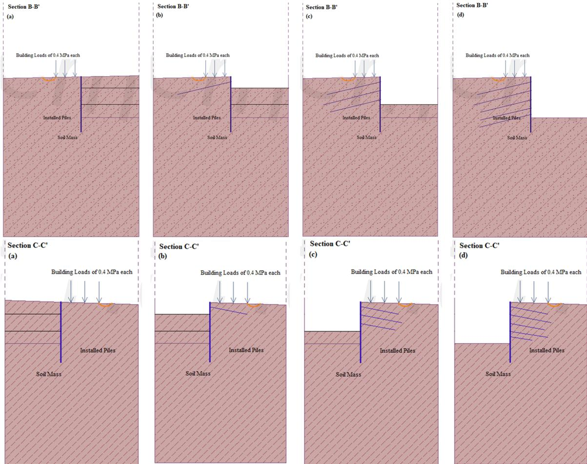
Figure 9. Steps involved in sections B<sub>1</sub>-B<sub>1</sub>' and C<sub>1</sub>-C<sub>1</sub>' - (a) installation of pile, (b), (c), and (d) installation of anchors.
