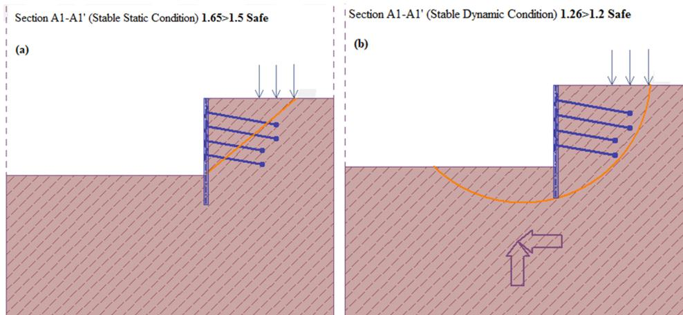
Figure 7. Stability check after remedies (a) stable static condition, (b) stable dynamic condition.
