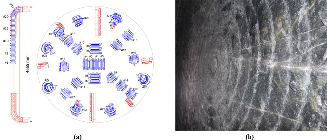
Figure 3. (a) Schematic drawing of TBM cutter-head used for boring northern lot of KWCT project; (b) Disc trajectories on tunnel face in KWCT project [7].
