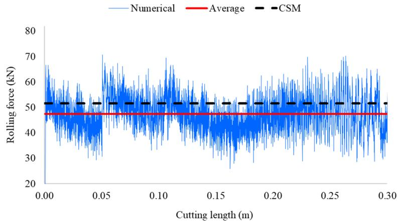
Figure 8. Variation of rolling force of disc cutter calculated using 3DEC and CSM.
