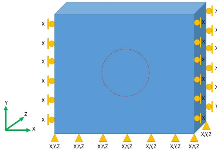
Figure 12. Boundary conditions applied to model in X, Y, Z directions.
