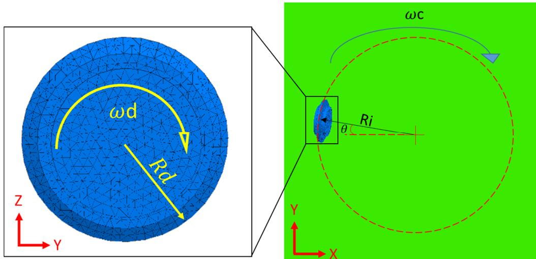
**Figure 6. Radius of rotation ( $R_d$ ) and revolution ( $R_i$ ) of disc cutter with corresponding angular velocities ( $\omega_d$ ) and ( $\omega_c$ ).**
