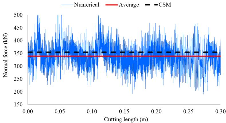
**Figure 7. Variation of normal force on disc cutter calculated using 3DEC and CSM.**
