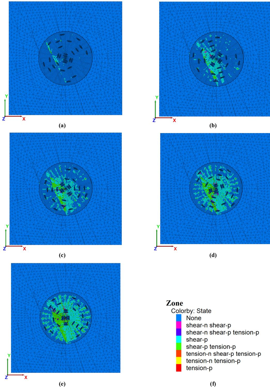
Figure 14. Development of plastic zones in unit RT-1 due to TBM boring during 10 s dynamic time: (a) 1<sup>st</sup> s.; (b) 2<sup>nd</sup> s.; (c) 4<sup>th</sup> s.; (d) 6<sup>th</sup> s.; (e) 8<sup>th</sup> s.; (f) 10<sup>th</sup> s.
