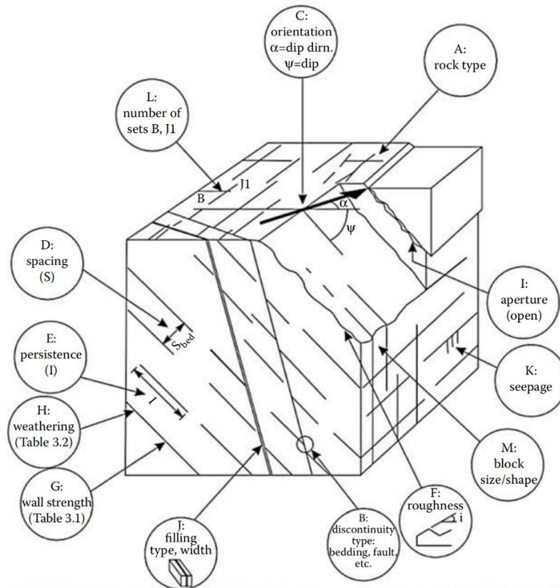
Figure 1. Characteristics of discontinuities within rock mass [8].
