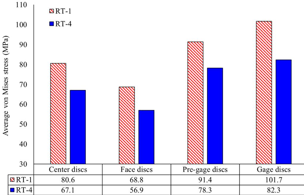
Figure 20. Average von Mises stresses for different groups of disc cutters in units RT-1 and RT4 of KWCT.
