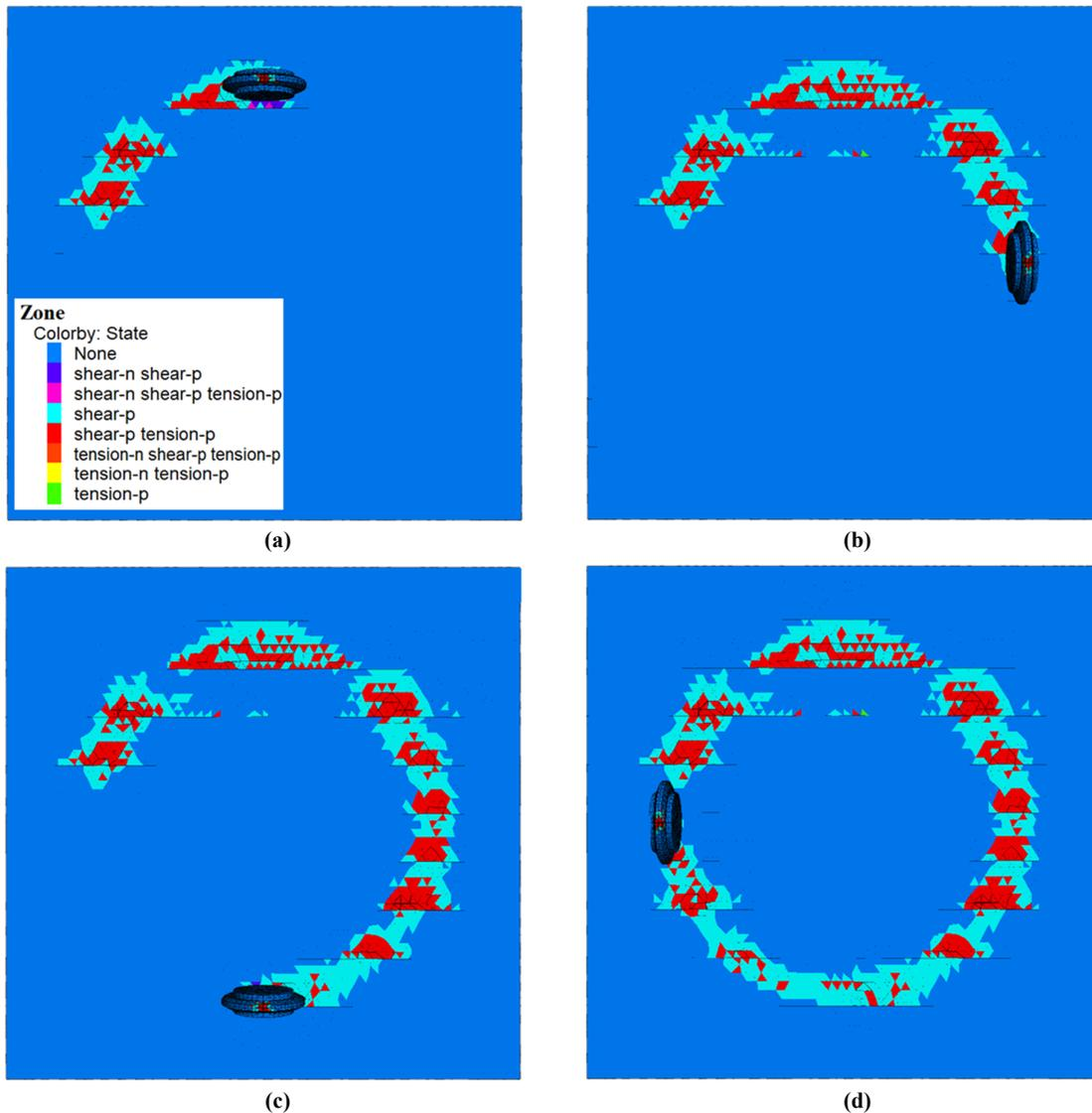
Figure 10. Extent of excavated material caused by motion of disc cutter on jointed rock mass and resulting plastic zones at different angular positions: (a) 90 degrees; (b) 180 degrees; (c) 270 degrees; (d) 360 degrees.
