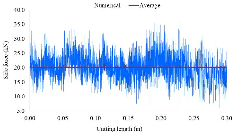
Figure 9. Estimated variation of side-force of disc cutter calculated using 3DEC.
