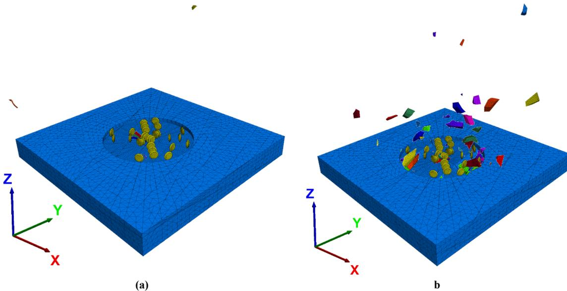
Figure 17. Separated rock blocks from surface of tunnel face due to cutter-head (disc cutters set) advancing in numerical model for geological units: (a) RT-1; (b) RT-4.
