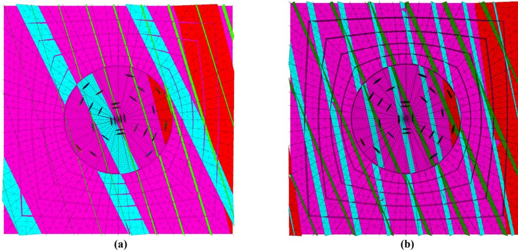
Figure 13. Joint sets for geological units: (a) RT-1; (b) RT-4.
