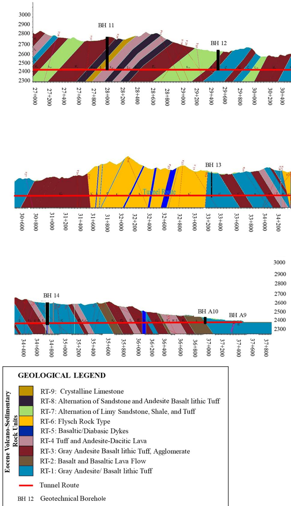
Figure 4. Geo-technical profile of completed part of north lot in KWCT project [7].
