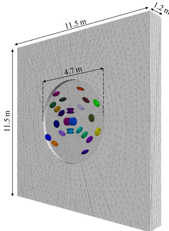
**Figure 11. Model geometry generated by 3DEC for numerical analysis of rock mass cutting by TBM cutter-head.**
