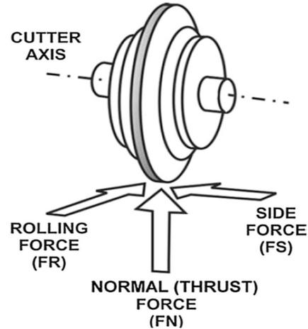
Figure 5. Forces acting on a disc cutter [47].
