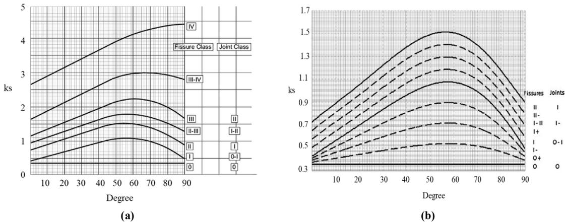
**Figure 2. (a) Calculation of fracturing factor ( $k_s$ ) based on angle between tunnel axis and plane of weakness and fracture class [9]; (b) Interpolated curves for low fracture classes (i.e. joints: 0-I, and fissures: 0-II) [10].**
