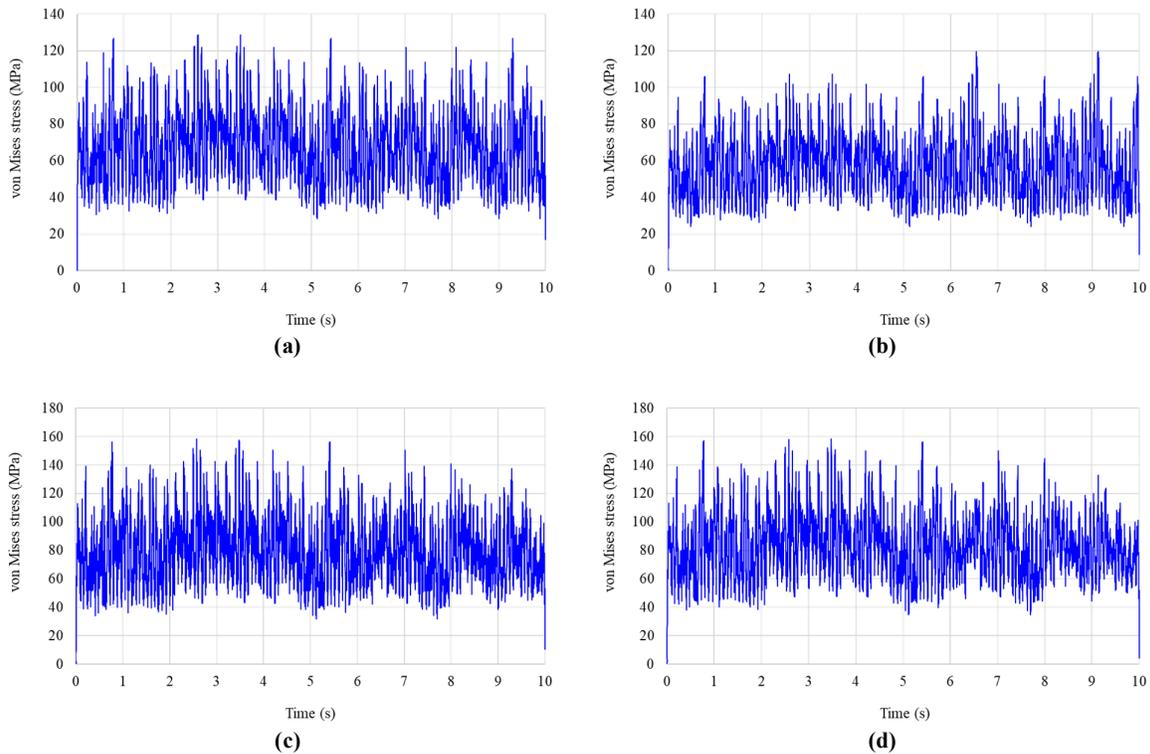
**Figure 19.** Von Mises stress oscillation graph versus to dynamic analysis time for TBM disc cutters of geological unit RT-4: (a) center group; (b) face group; (c) pre-gage group; (d) gage group.
