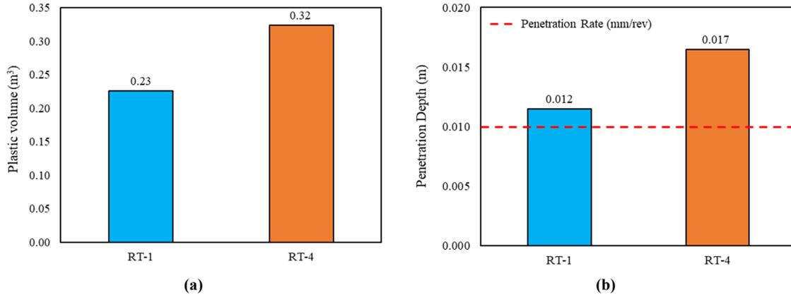
Figure 16. Numerical results: (a) Volume of plastic zone in numerical model for two selected geological units; (b) Penetration depth affected by plastic zones and nominal penetration rate.
