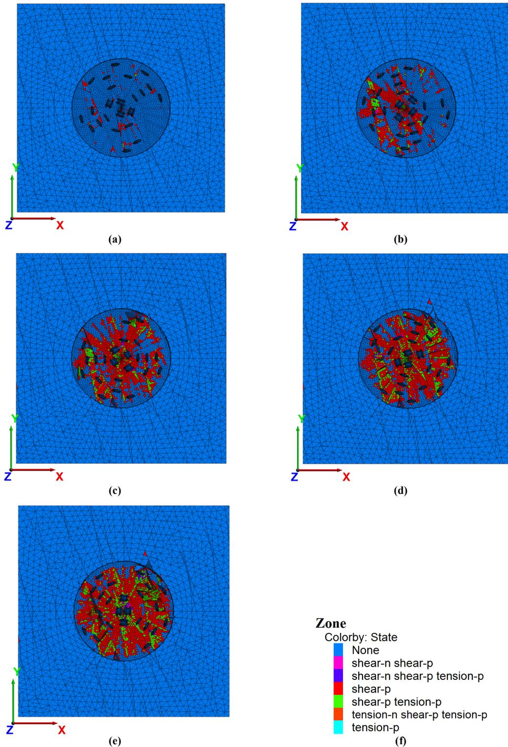
Figure 15. Development of plastic zones in unit RT-4 due to TBM boring during 10 second dynamic time: (a) 1<sup>st</sup> s.; (b) 2<sup>nd</sup> s.; (c) 4<sup>th</sup> s.; (d) 6<sup>th</sup> s.; (e) 8<sup>th</sup> s.; (f) 10<sup>th</sup> s.
