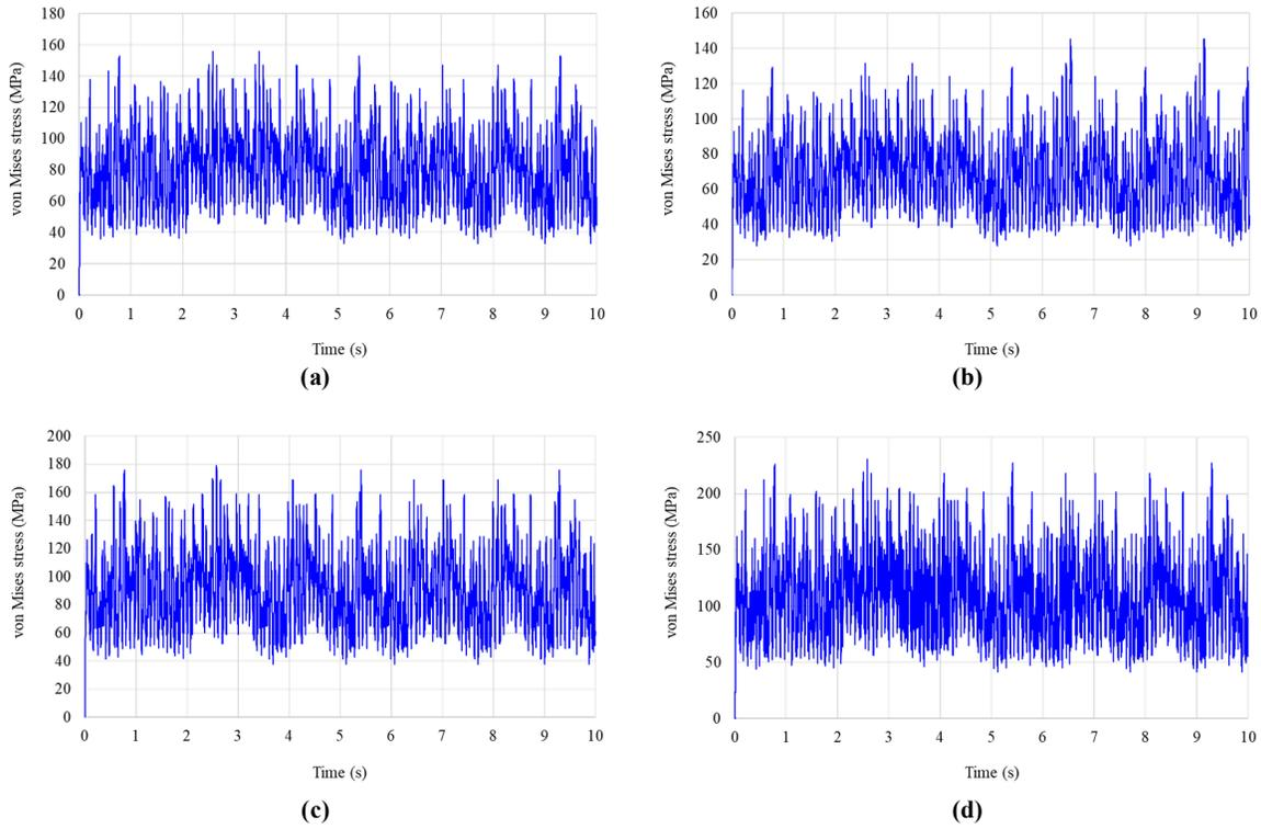
**Figure 18.** Von Mises stress oscillation graph versus to dynamic analysis time for TBM disc cutters of the geological unit RT-1: (a) center group; (b) face group; (c) pre-gage group; (d) gage group.
