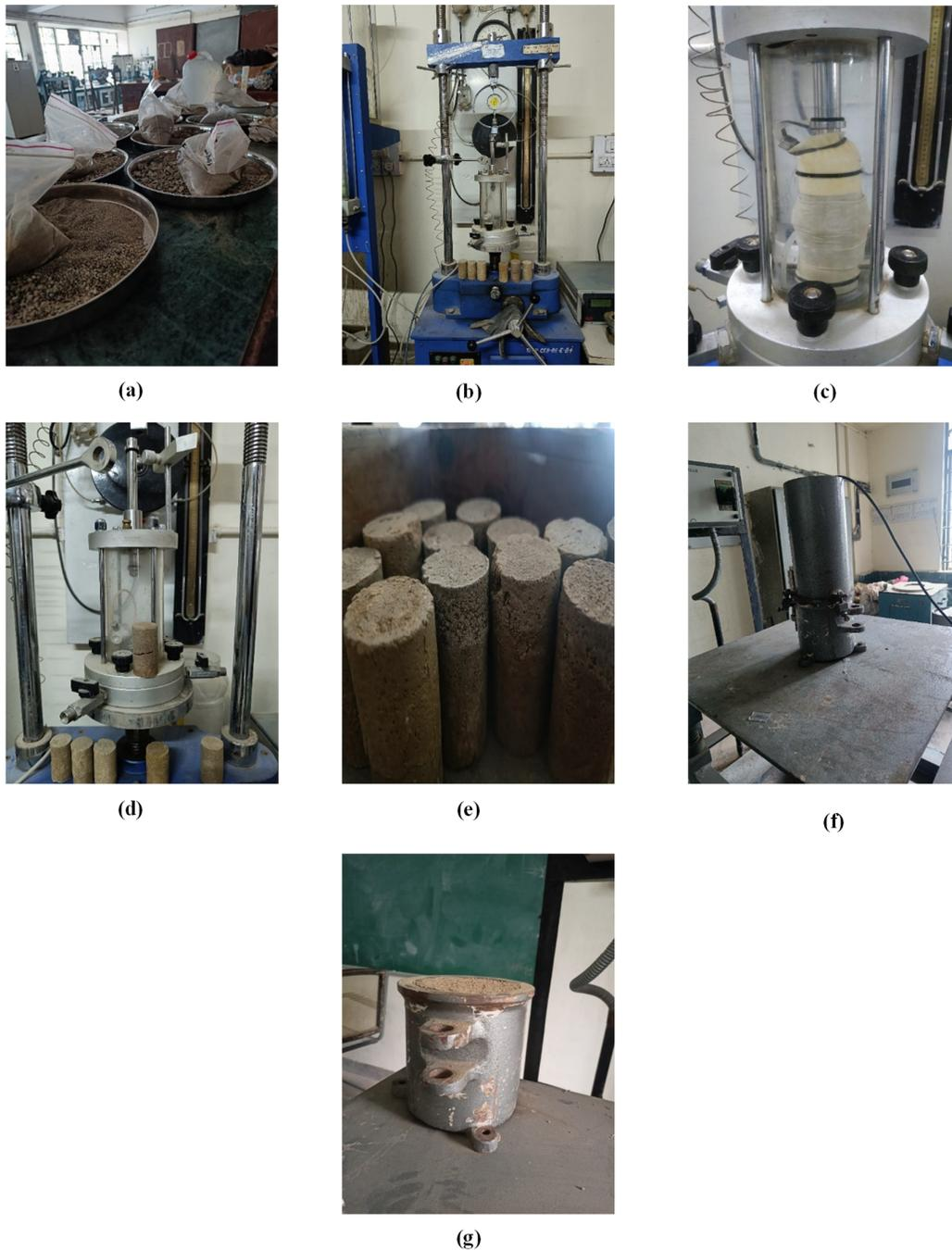
Figure 3. (a) Soil sample. (b), (c), (d) and (e) triaxial testing setup. (f) and (g) relative density test.
