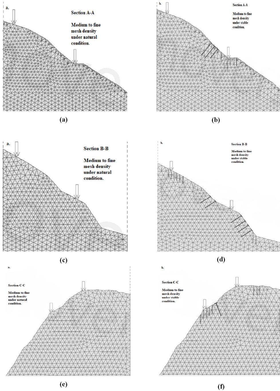
Figure 4. Finite element model for all sections from medium to fine mesh density.
