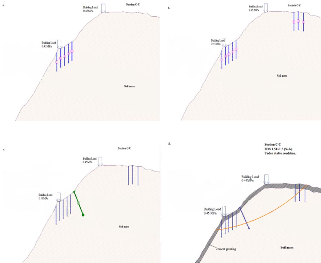
**Figure 8. Steps involved in section C-C, (a) and (b) installation of piles. (c) Installation of anchors. (d) Stability check after grouting and all remedies.**
