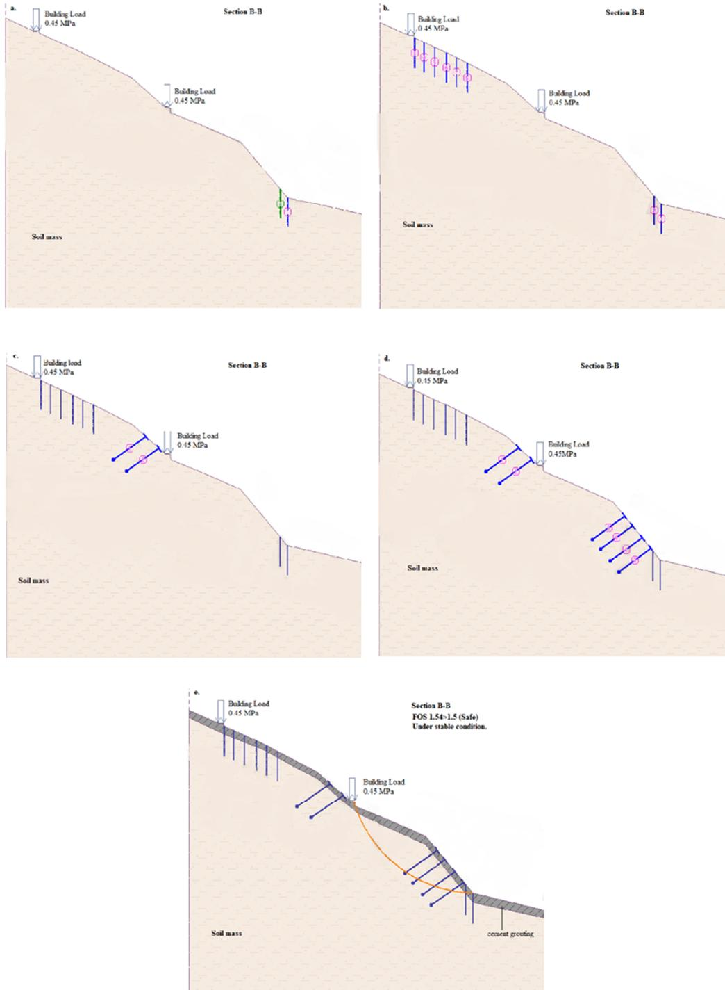
Figure 7. Steps involved in section B-B, (a) and (b) installation of piles. (c) and (d) installation of anchors. (e) stability checks after all remedies.
