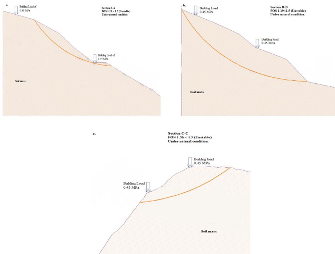
Figure 5. a) Stability check of Section A-A. b) Stability check of Section B-B. c) Stability check of Section C-C under natural condition.
