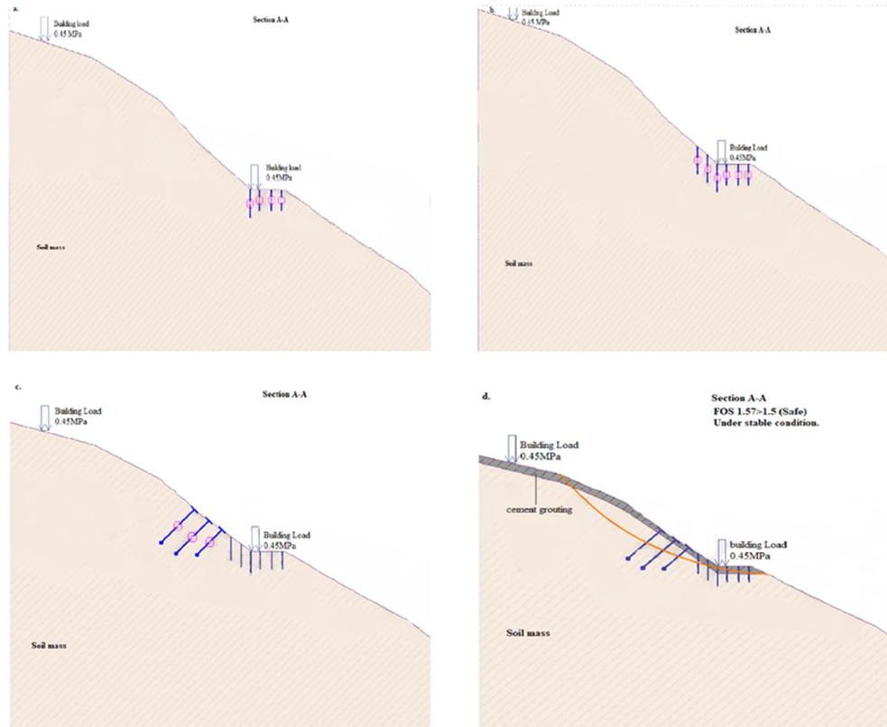
**Figure 6.** Steps involved in section A-A, (a) and (b) installation of piles. (c) Installation of anchors. (d) Stability checks after all remedies.
