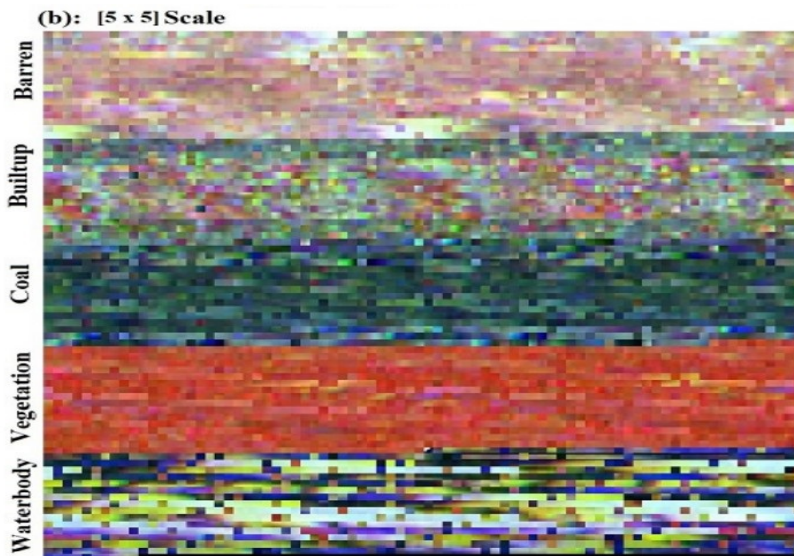
Figure 5. [5 × 5] scale sizes dataset with five class viz. barren land, built-up area, active coal mine, vegetation, and water body.
