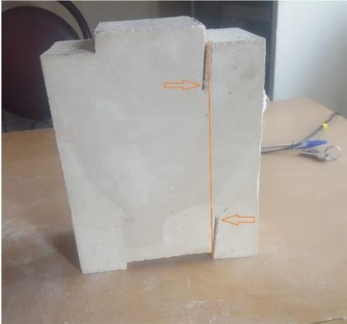
Figure 29. Sample containing a non-standard notch.
