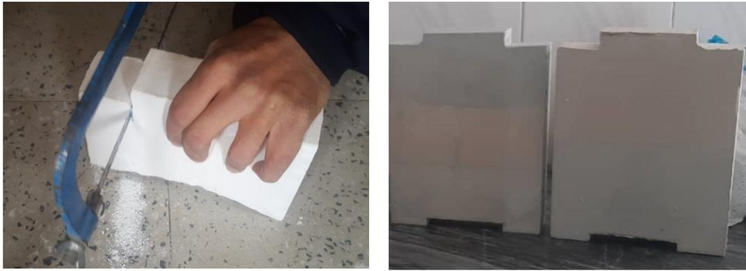
Figure 34. Use of a hand saw in making a sample with non-persistent notches.
