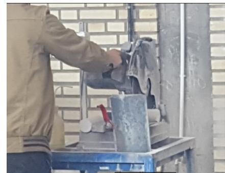
Figure 31. Using an electric saw in making a sample with non-persistent notches.
