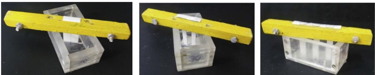
Figure 22. Making method of a sample containing non-continuous joints [22].
