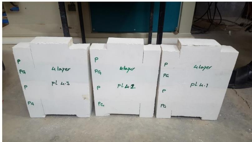
Figure 35. Samples of four layers with different notch lengths.
