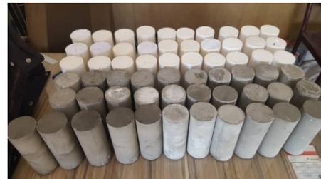
Figure 25. Cylindrical samples prepared from plaster and reinforced plaster for the uniaxial compression tests.
