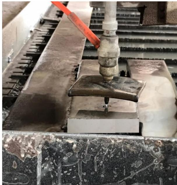
Figure 30. Using a water jet to create a joint.
