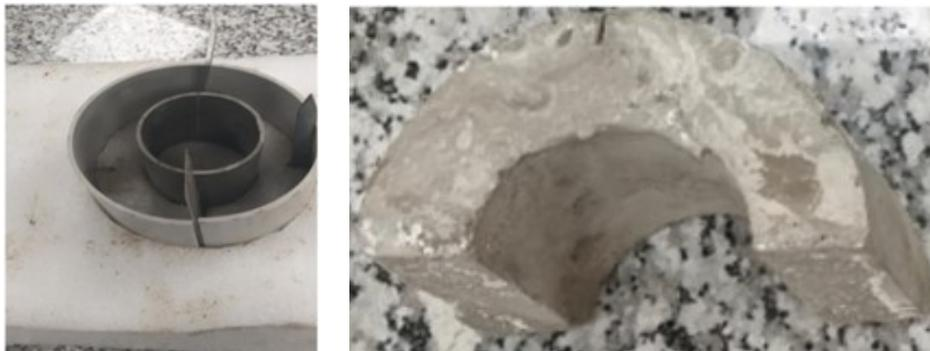
**Figure 17.** Mold used to make a semi-ring sample containing an edge joint [17].
