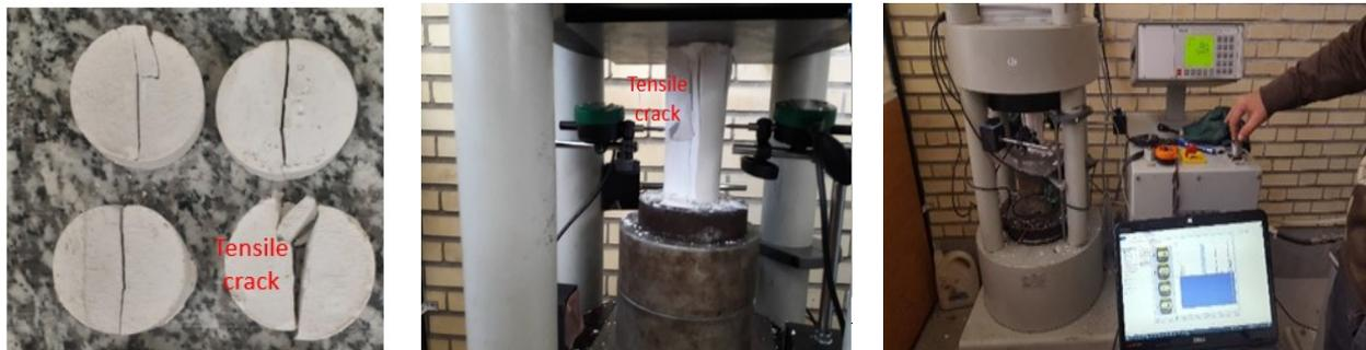
Figure 26. Conducting uniaxial compressive test and Brazilian tension.
