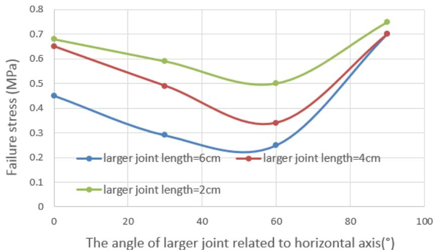
Figure 10. Effects of joint length and joint inclination angle on strength of the modelled specimen.
