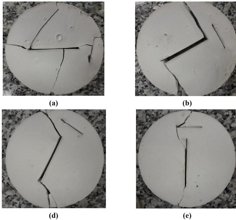
Figure 9. Mechanism of failure process in the rock-like material specimens containing two non-persistent joints with large and small sizes; the large joint inclination angle changes as a) 0, b) 30, c) 60, d) 90 degrees, respectively.
