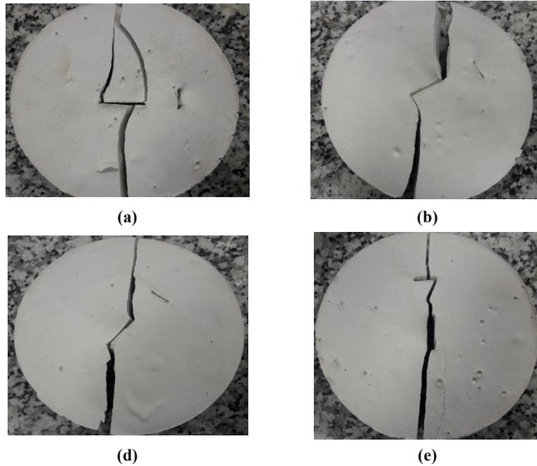
**Figure 7. Failure mechanisms of rock-like material specimens with two non-persistent joints when the inclination angle of large crack is a) 0, b) 30, c) 60, d) 90.**
