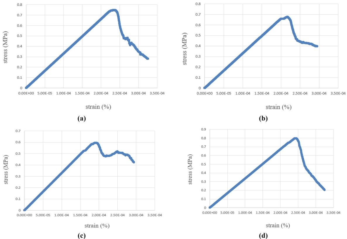
Figure 16. Stress versus strain for four models with different large joint angles of a) 0, b) 30, c) 60, and d) 90.
