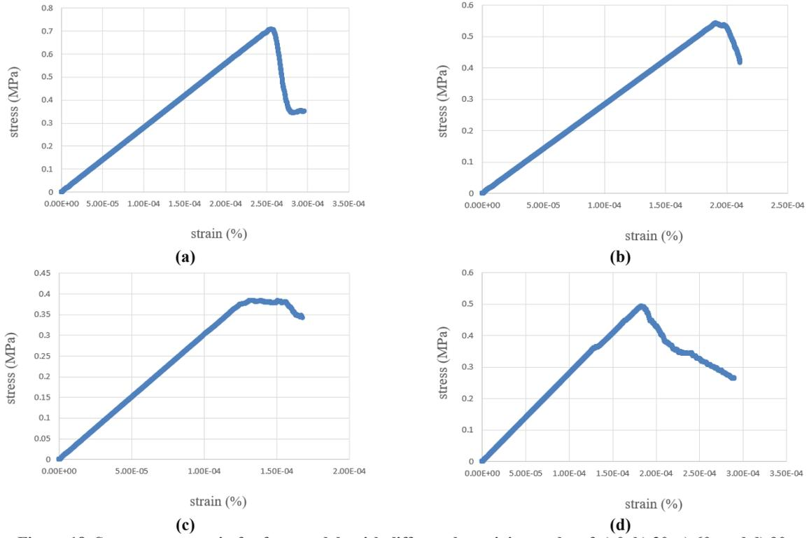
Figure 18. Stress versus strain for four models with different large joint angles of a) 0, b) 30, c) 60, and d) 90.
