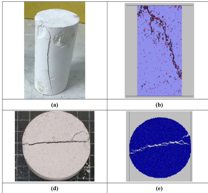
Figure 11. a) Experimental compression test, b) numerical compression test, c) experimental Brazilian test, and d) numerical Brazilian test.
