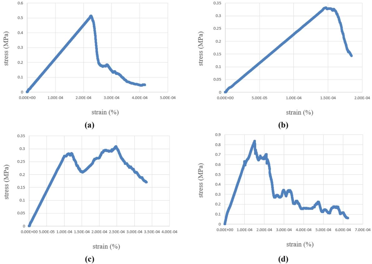
**Figure 20. Stress versus strain for four models with different large joint angles of a) 0, b) 30, c) 60, and d) 90.**
