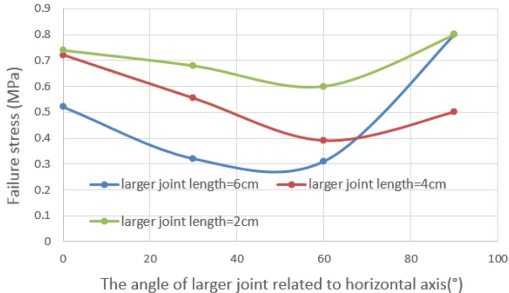
Figure 21. Effect of joint angle on strength of models.
