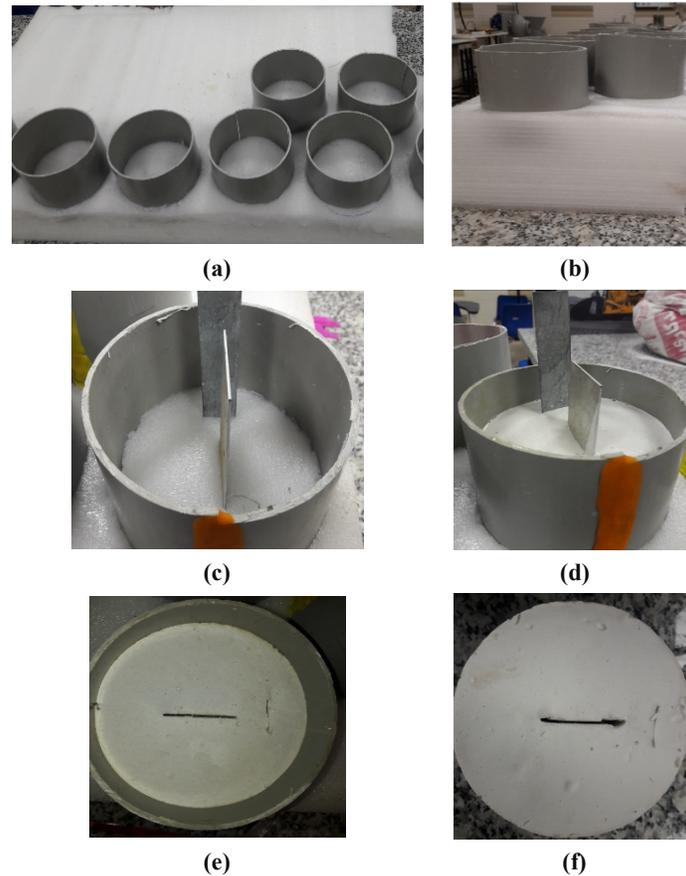
**Figure 1. a) Frame with diameter of 10 cm and thickness of 40 cm. b) Frame with diameter of 10 cm and thickness of 40 cm. c) Shim with dimension of 100 mm × 1 mm × 60 mm inside the plastic fiber. e) Plaster slurry inside the mold e) Aluminum sheet is removed from the mold. f) Sample consisting of T-shaped non-persistent joint.**
