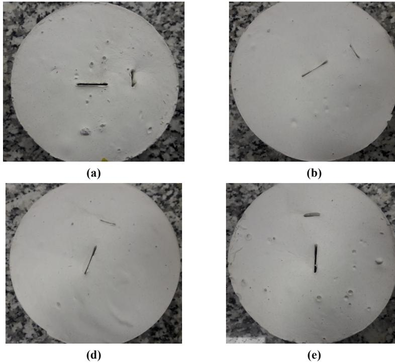
Figure 3. T-shaped joint with large joint angle of a) 0, b) 30, c) 60, d) 90; large joint length was 2 cm.
