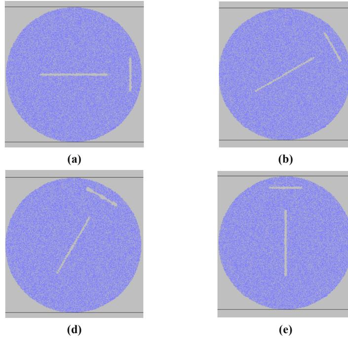
Figure 14. Two T-shaped joints with large joint angle of a) 0, b) 30, c) 60, d) 90, e) 120, and f) 150.
