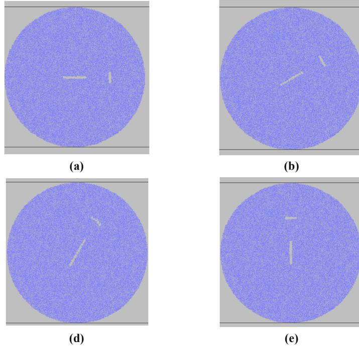
Figure 12. T-shaped joint with large joint angle of a) 0, b) 30, c) 60, d) 90, e) 120, and f) 150.
