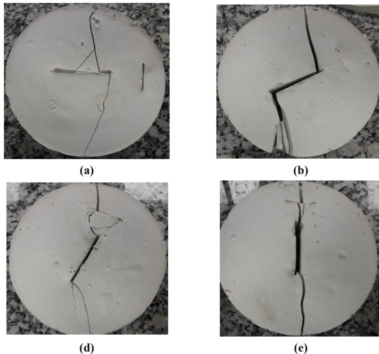
**Figure 8. Failure pattern of specimens containing two non-persistent joint with large joint angle of a) 0, b) 30, c) 60, d) 90.**
