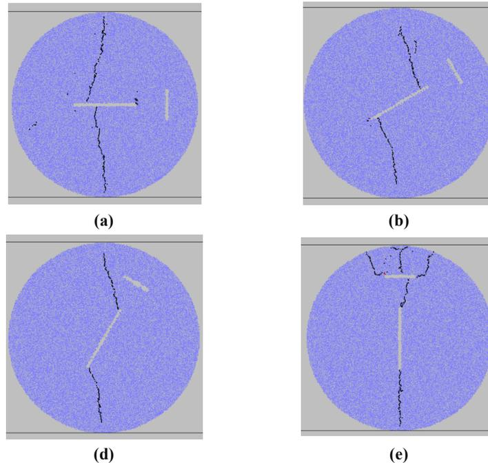
**Figure 17. Failure pattern of specimens containing three non-persistent joint with large joint angle of a) 0, b) 30, c) 60, d) 90, e) 120, and f) 150.**
