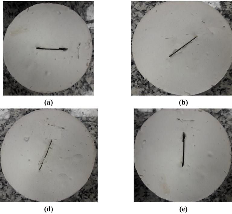
Figure 4. T-shaped joint with large joint angle of a) 0, b) 30, c) 60, d) 90; large joint length was 4 cm.
