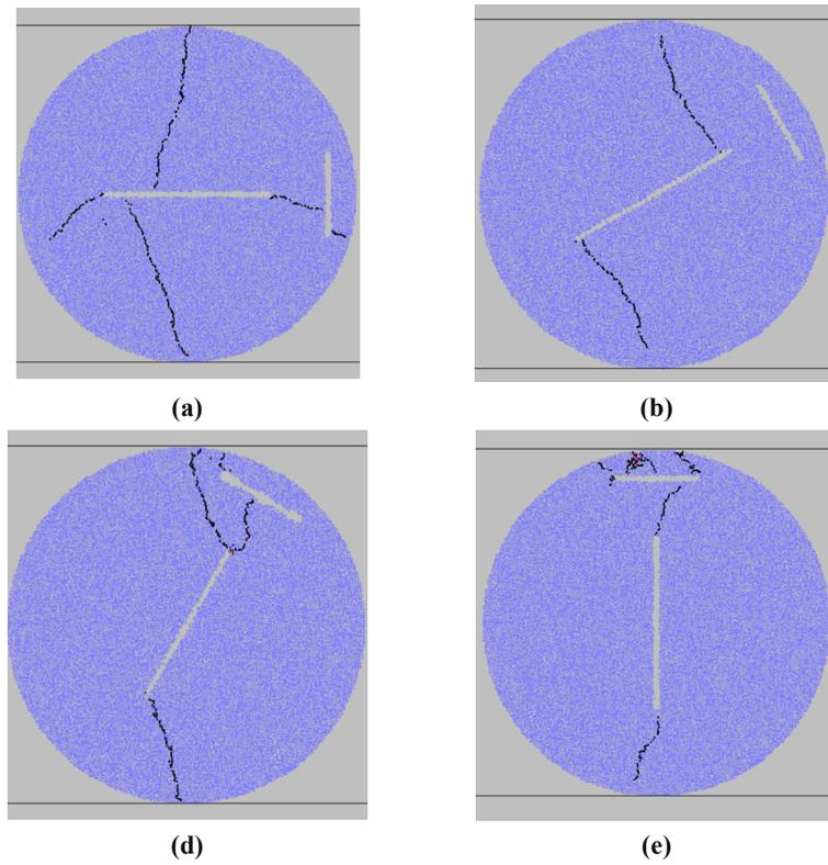
Figure 19. Failure pattern of specimens containing two non-persistent joint with large joint angle of a) 0, b) 30, c) 60, d) 90, e) 120, and f) 150
