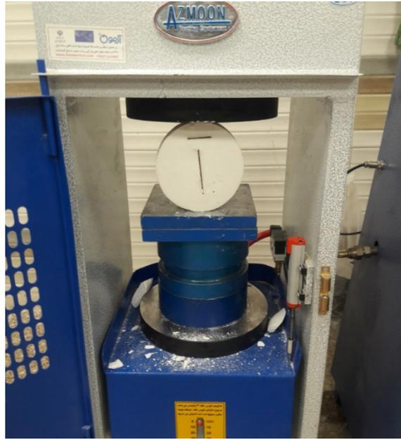
Figure 6. Specimens are placed between plates of the loading machine.
