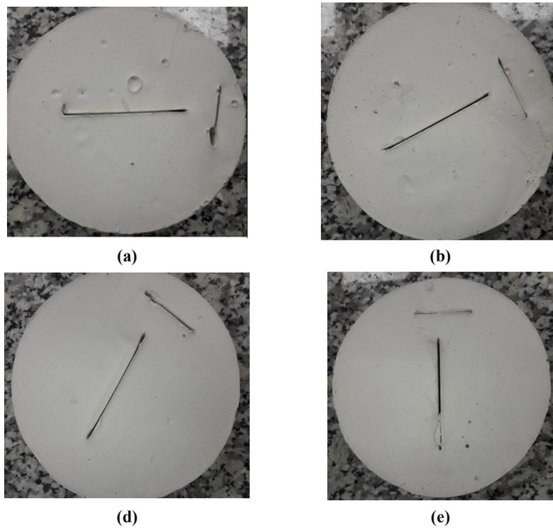
Figure 5. T-shaped joint with large joint angle of a) 0, b) 30, c) 60, d) 90; large joint length was 6 cm.
