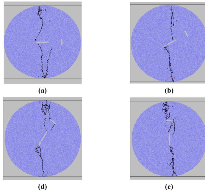
Figure 15. Failure pattern of specimens containing three non-persistent joint with large joint angle of a) 0, b) 30, c) 60, d) 90, e) 120, and f) 150.
