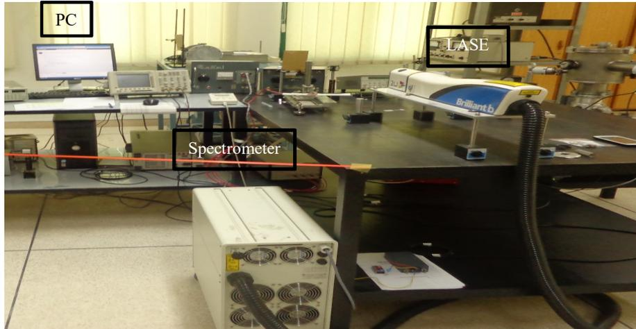
Figure 3. Physical diagram of LIBS setup used for rock analysis.
