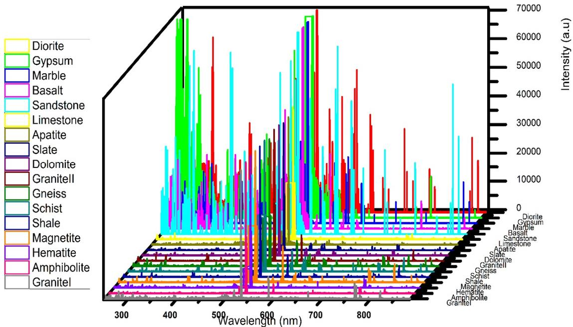
Figure 4. Optical emission spectra of rock samples in the range 250-870 nm.
