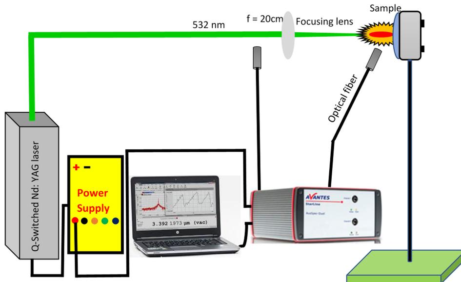
Figure 2. Schematic diagram of LIBS setup used for rock analysis.
