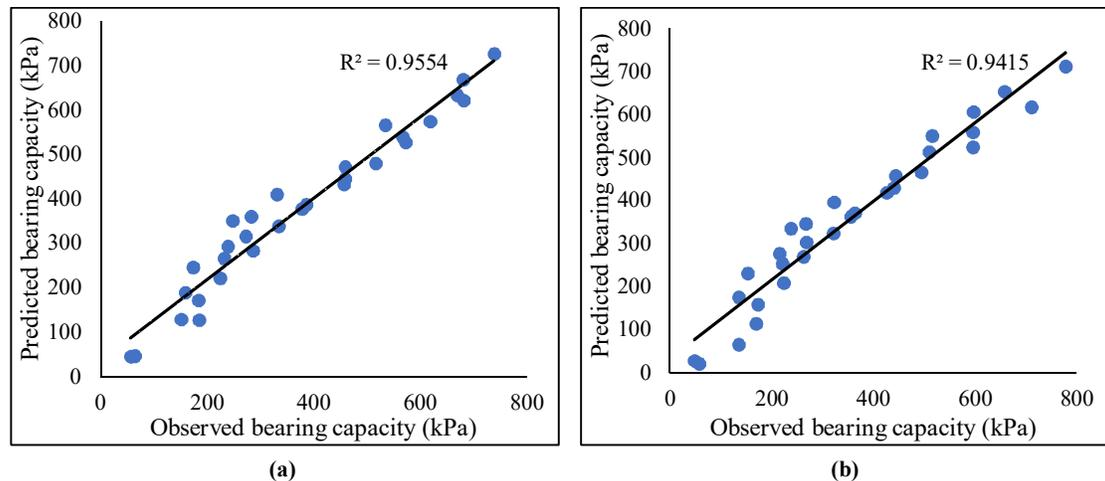
**Figure 8. Variation of observed and predicted bearing capacity (a) square footing (b) circular footing.**
