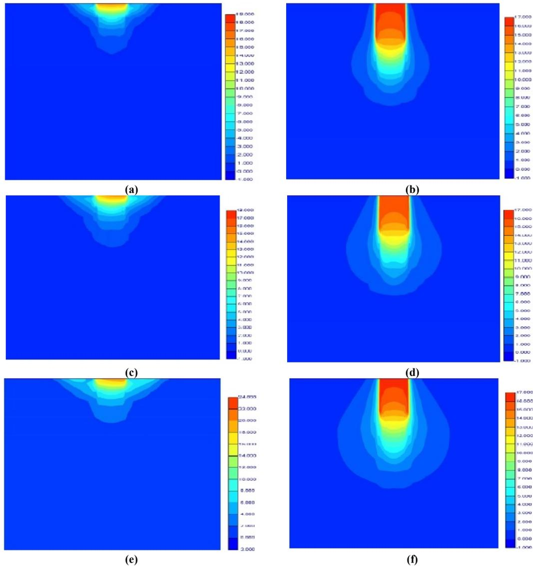
**Figure 10. Failure pattern for unskirted ( $h/B = 0$ ) and skirted ( $h/B = 2$ ) circular footing with different friction angle (a, b)  $36^\circ$  (c, d)  $40^\circ$  (e, f)  $42^\circ$ .**
