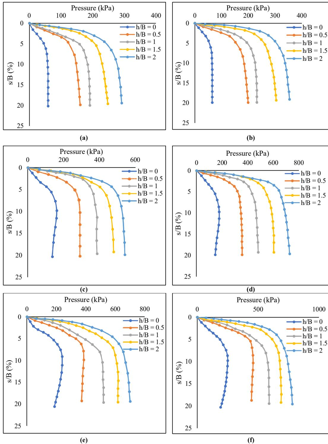
**Figure 3. Pressure-settlement plots for square footings (a, c, e) partially rough (b, d, f) rough interface.**
