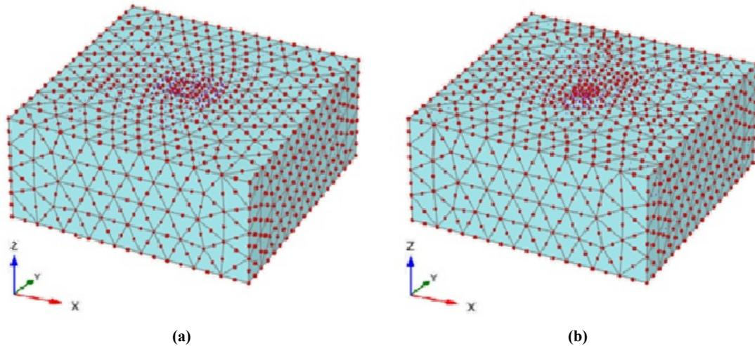
Figure 2. Generated mesh for numerical models (a) Square (b) Circular.
