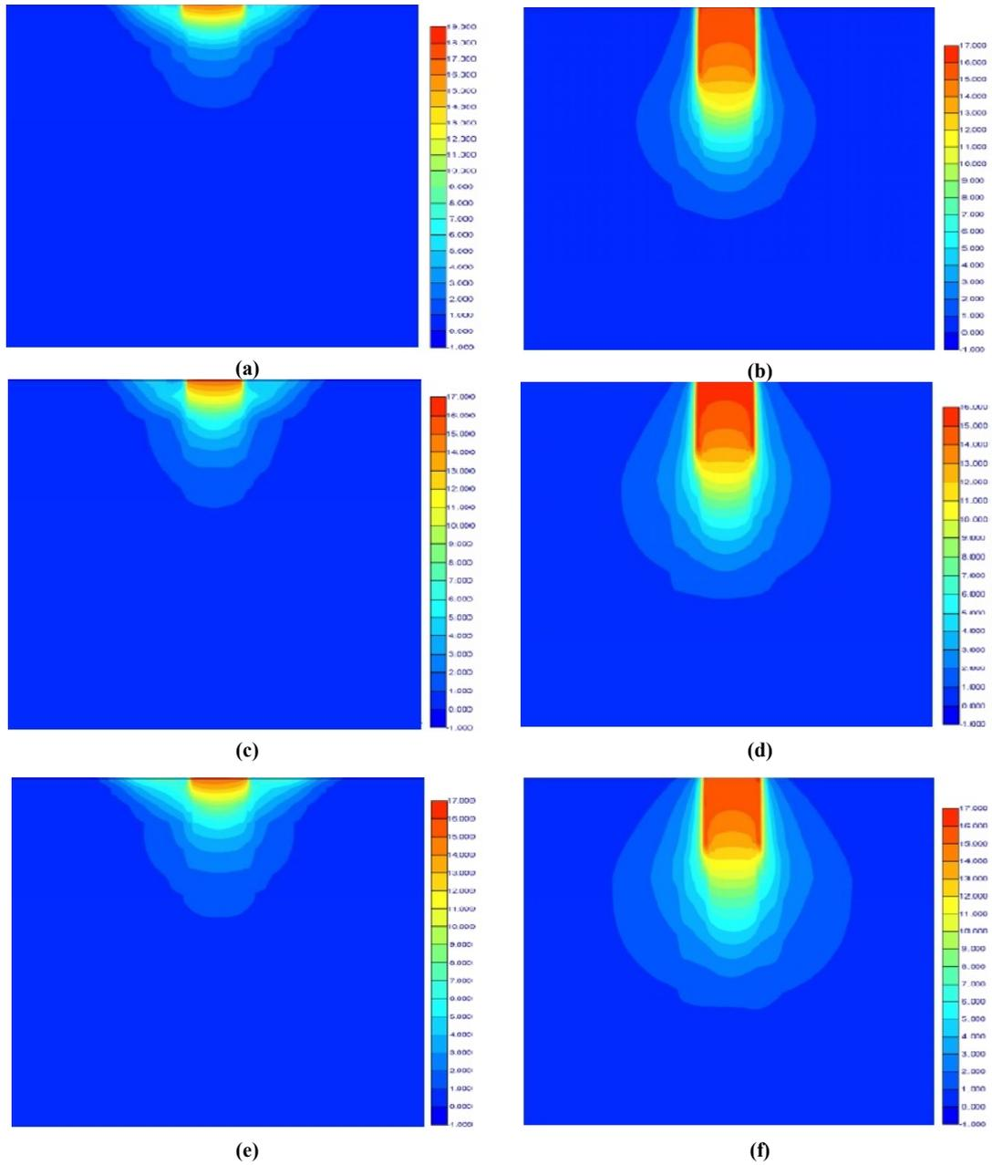
**Figure 9. Failure pattern for unskirted ( $h/B = 0$ ) and skirted ( $h/B = 2$ ) square footing with different friction angle (a, b)  $36^\circ$  (c, d)  $40^\circ$  (e, f)  $42^\circ$ .**
