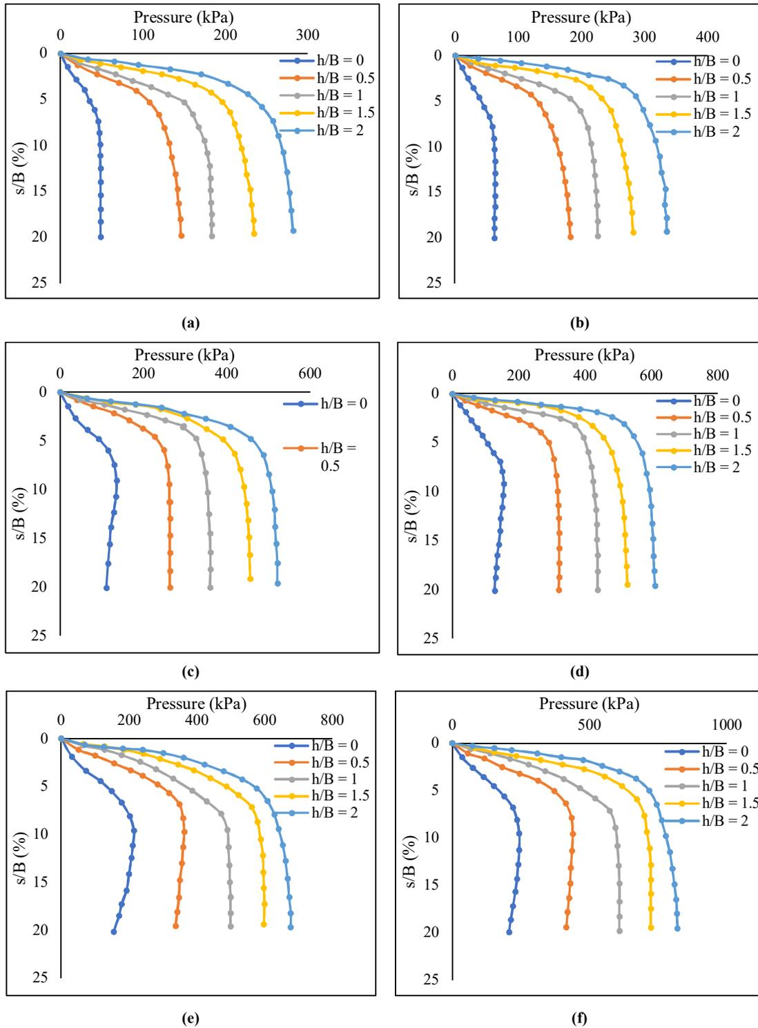
Figure 4. Pressure-settlement plots for circular footing (a, c, e) partially rough (b, d, f) rough interface.
