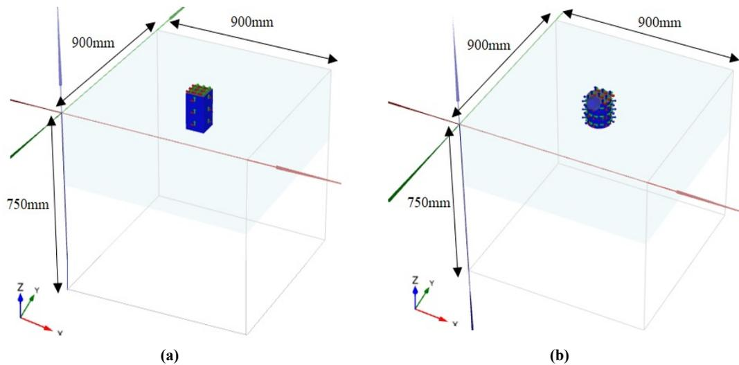
Figure 1. Numerical models of footings with skirt (a) Square (b) Circular.
