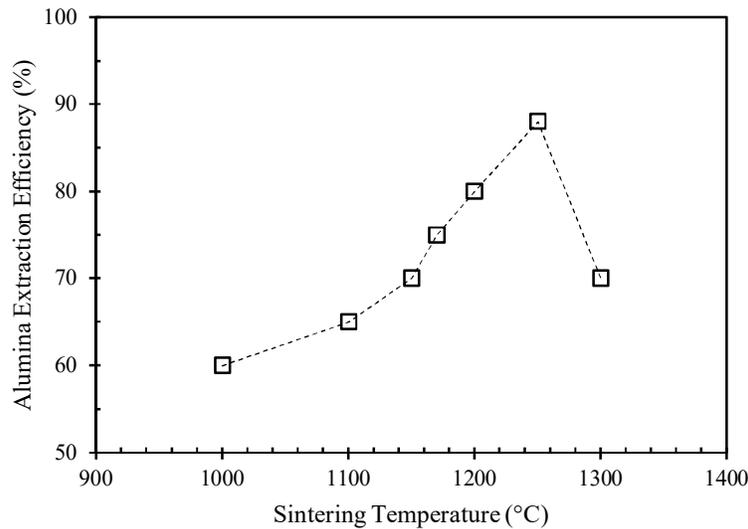
Figure 3. Effect of sintering temperature on alumina extraction efficiency (N/A = 0.9, C/S = 1.2, Sintering time = 80 min, leaching temperature = 80 °C, leaching time = 15 min).
