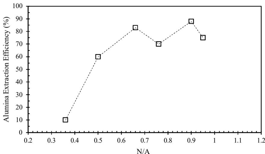
Figure 6. Effect of N/A on alumina extraction efficiency.
