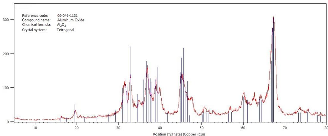
**Figure 8. XRD patterns of produced alumina powder.**
