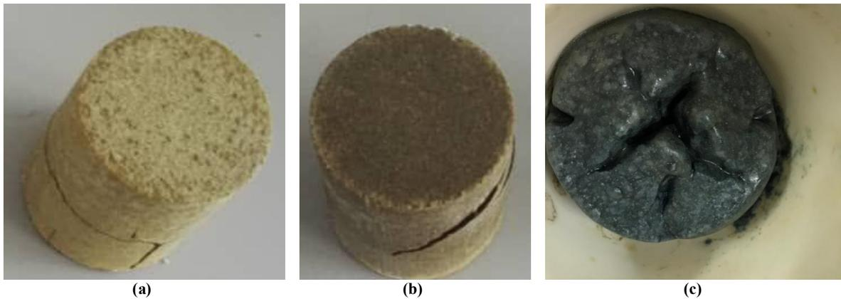
Figure 2. Images of molded cylinder sintered in different temperatures, a) 800, b) 1250, and c) 1300 °C.
