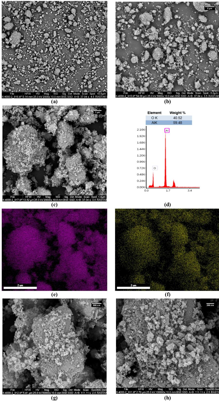
Figure 9. SEM Images of produced alumina powder, a,b,c,g and h are in 2000x, 5000x, 20000x, 50000x and 100000x magnification, d, e and f are map elemental EDS analysis, Al and O overlay plots for the c area.
