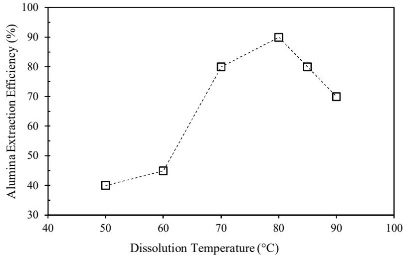
**Figure 7. Effect of dissolution temperature on alumina extraction efficiency.**
