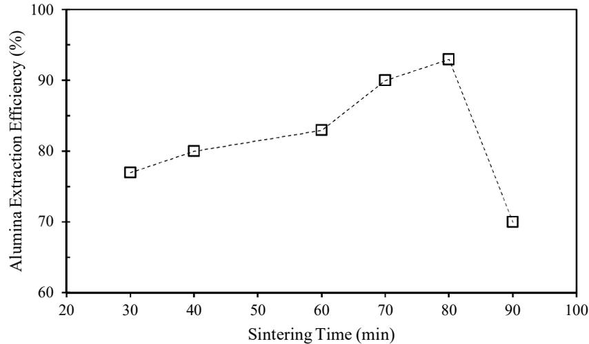
**Figure 4. Effect of sintering time on alumina extraction efficiency.**
