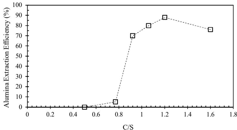
**Figure 5. Effect of C/S on alumina extraction efficiency.** (N/A = 0.9, sintering temperature = 1250 °C, sintering time = 80 min, leaching temperature = 80 °C, leaching time = 15 min).
