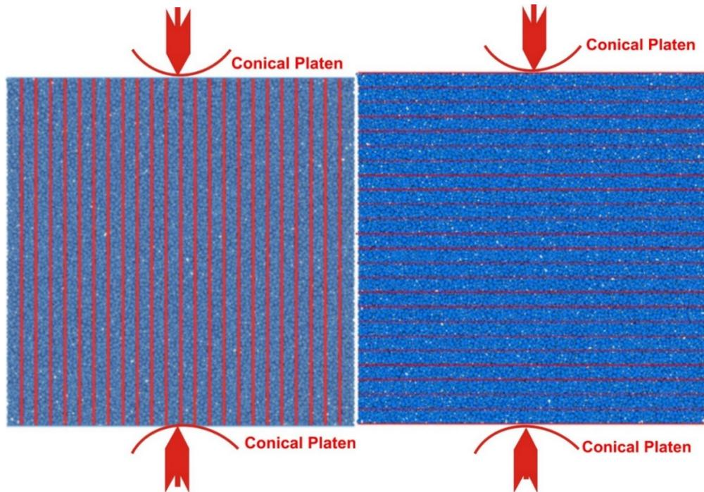
Figure 11. Orientation of lamination parallel and perpendicular to loading rate in PFC.
