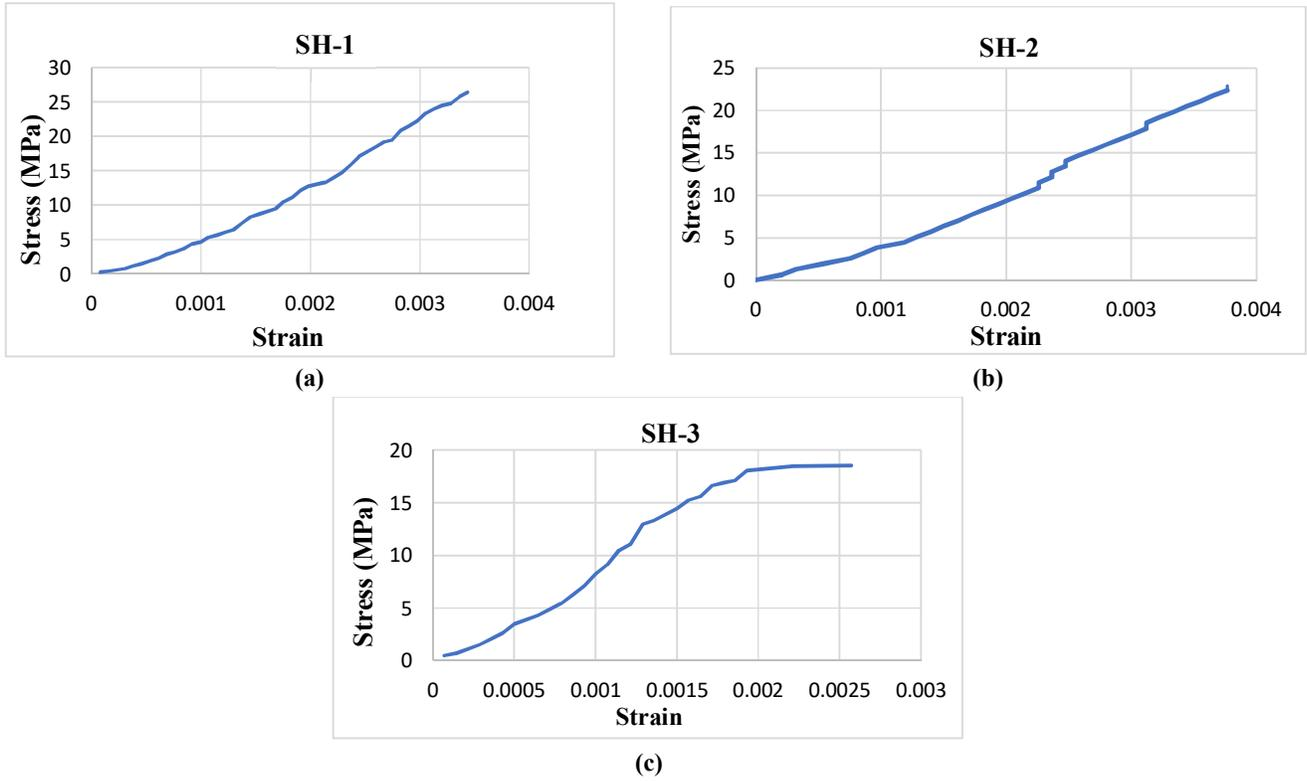
Figure 3. UCS test loading perpendicular to lamination.
