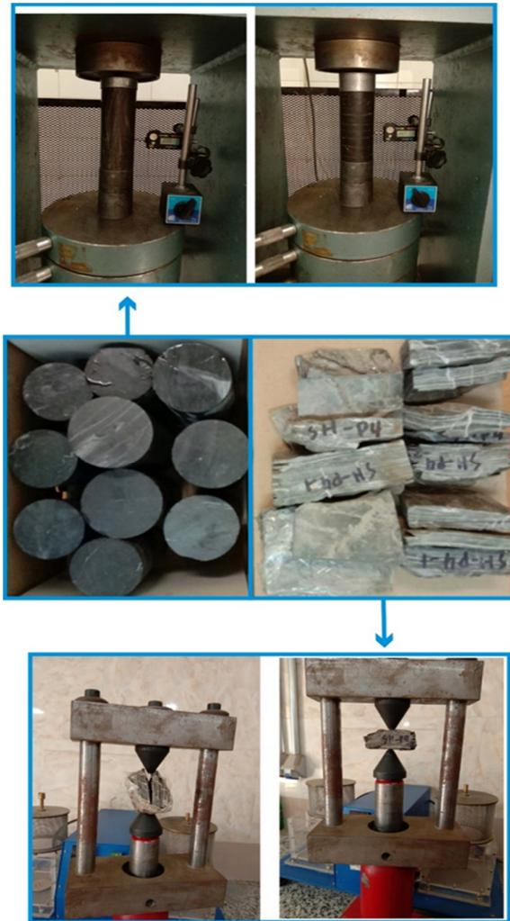
Figure 2. Prepared shale specimens for point load test and uniaxial compressive strength test.
