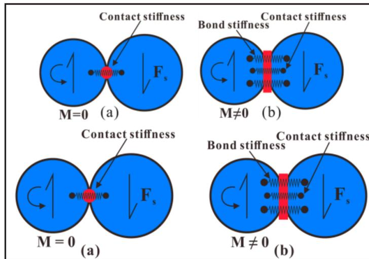
Figure 9. a). Contact bond model b). Parallel bond model [30].
