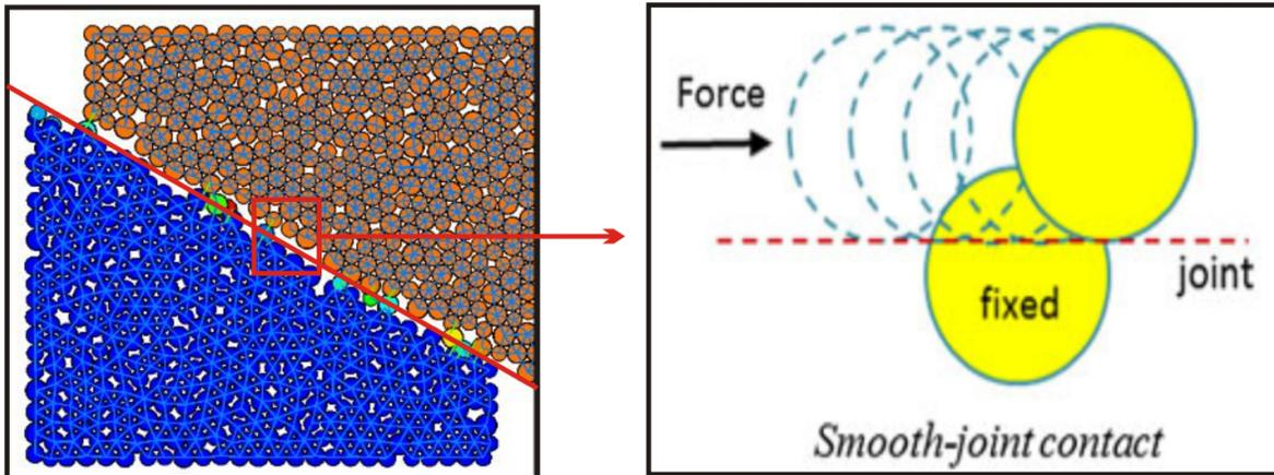
Figure 8. Detailed behavior of smooth joint model [29].
