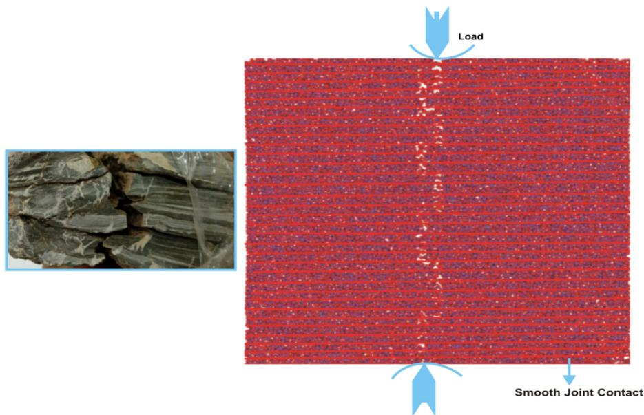
**Figure 15. SJM in point load test with the lamination direction perpendicular to loading.**
