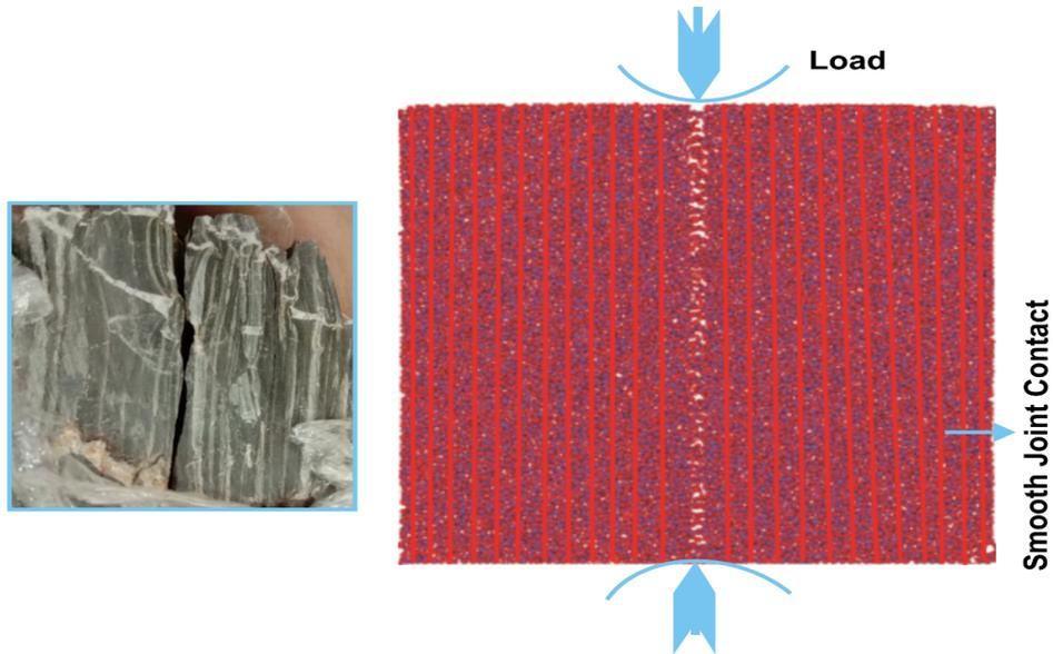
Figure 16. SJM in point load test with the lamination direction parallel to loading.
