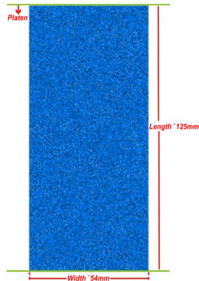
Figure 12. Model geometry of uniaxial compressive strength test in PFC.
