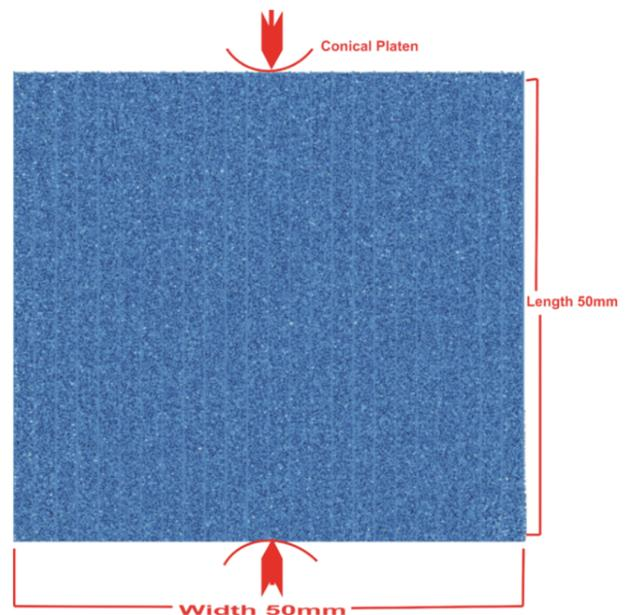
**Figure 10. Model geometry of point load test in PFC.**
