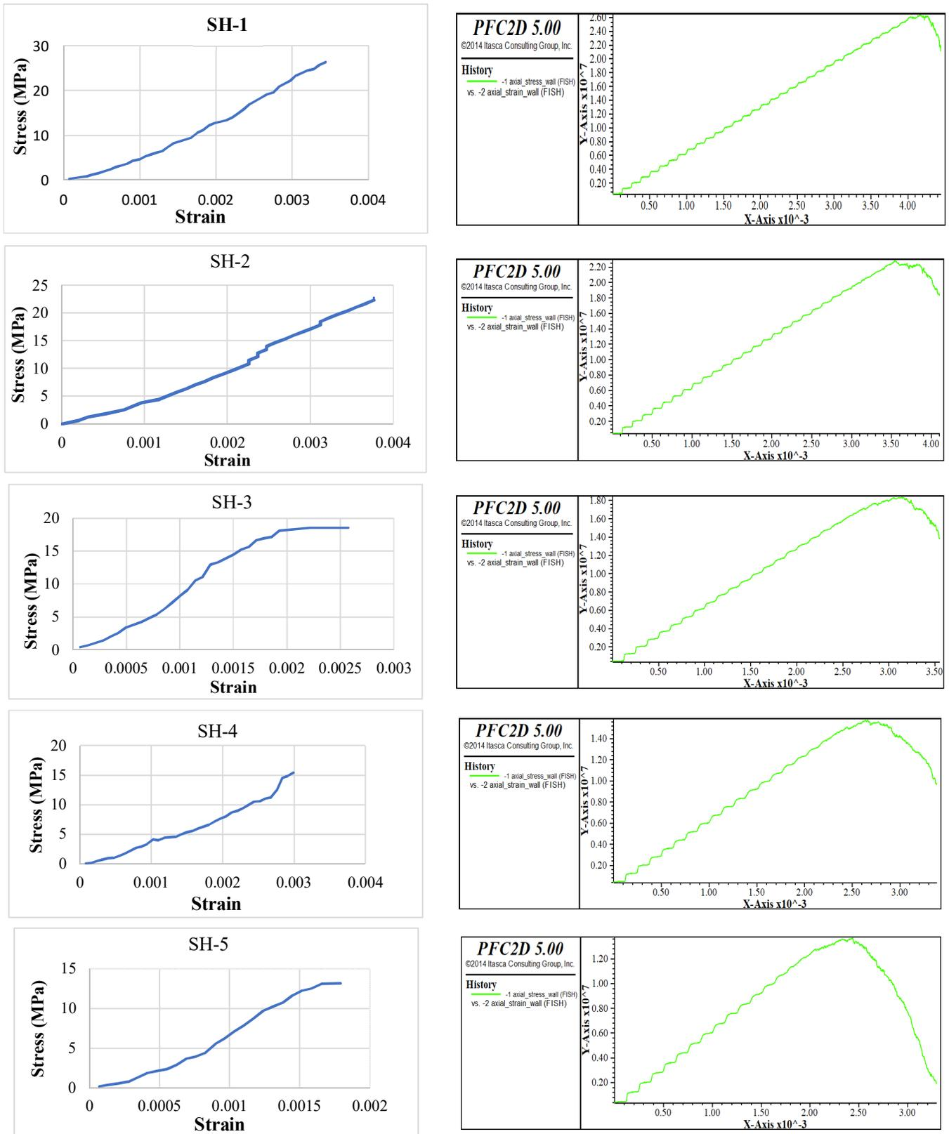
Figure 18. Validation of macro-parameters (UCS tests) with micro-parameters (PFC).
