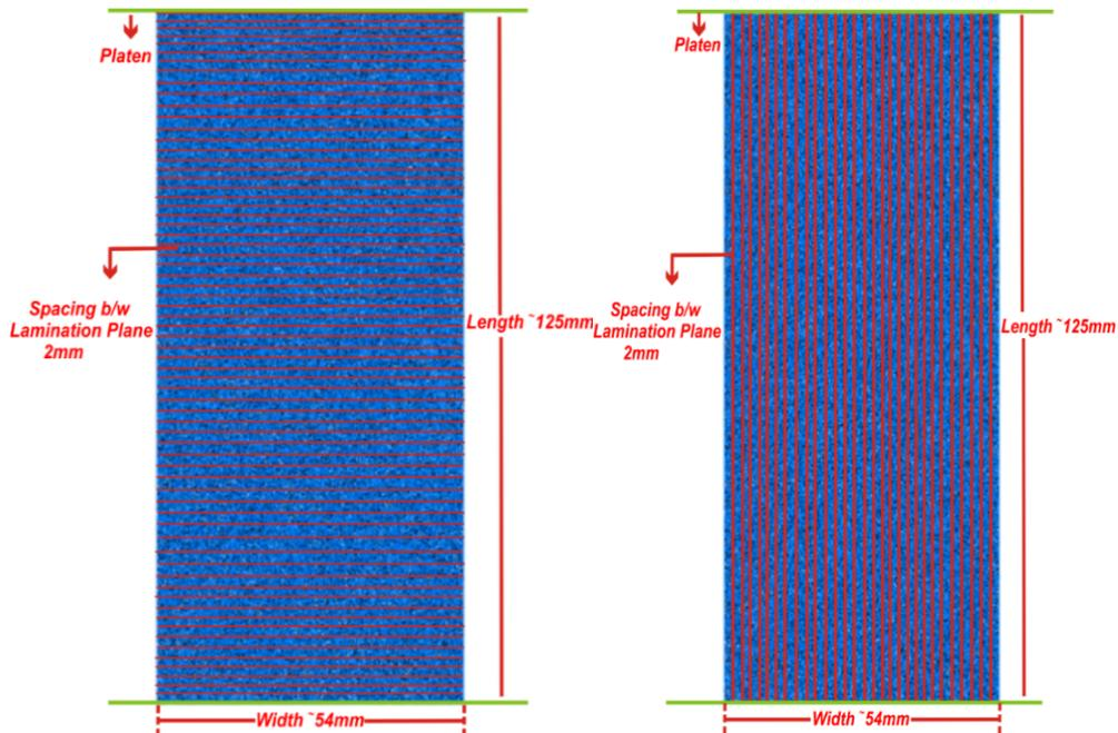
Figure 13. Orientations of lamination perpendicular and parallel to loading in PFC.
