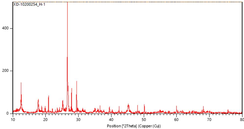
Figure 5. X-ray diffractogram of laminated shale sample.
