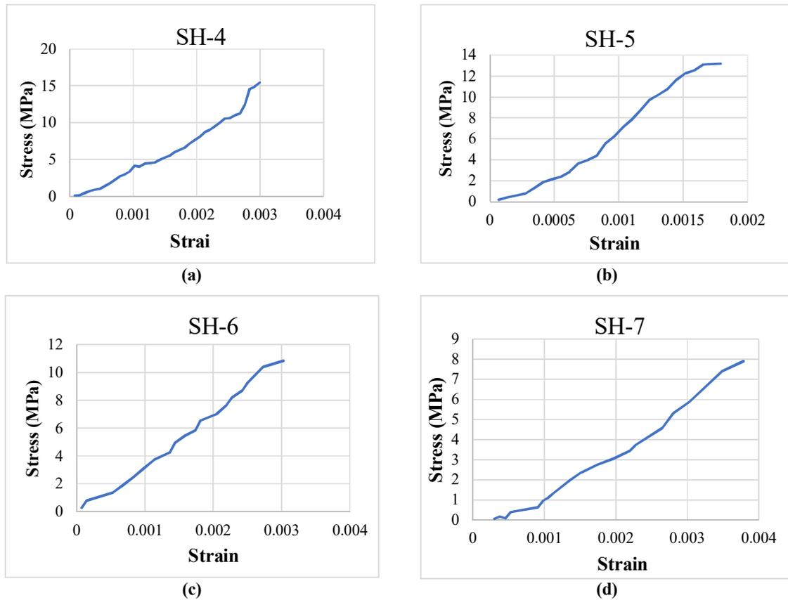
Figure 4. UCS tests loading parallel to lamination.
