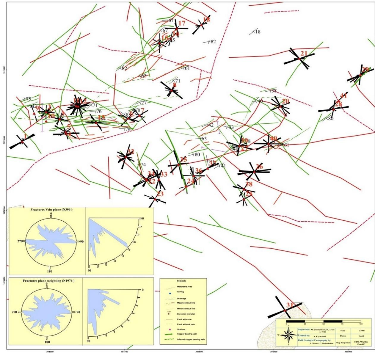
Figure 3. Map of mineralized and non-mineralized fractures of the Gazkhizan area with their residual diagrams in each geological station.
