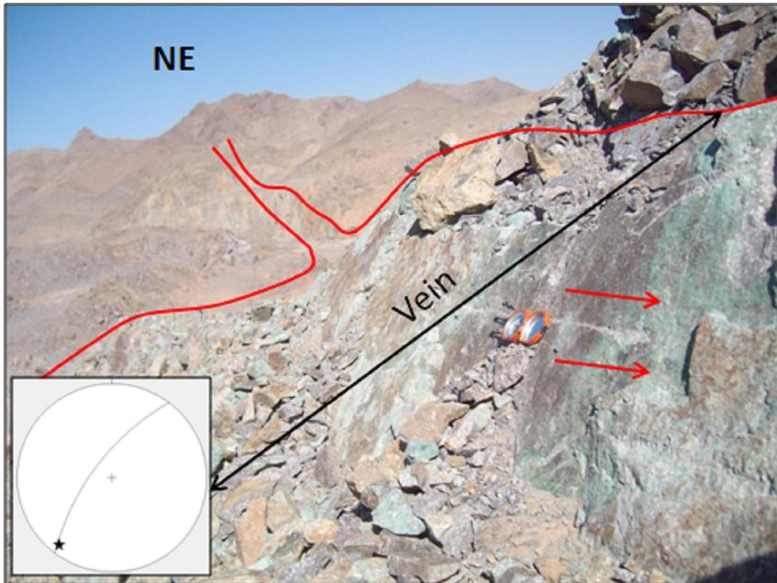
Figure 7. Left-slip faults along the R fractures along which copper ores are placed.
