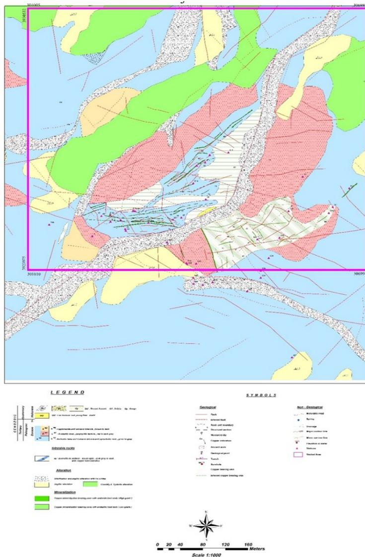
Figure 2. Geological-structural map of the Gazkhizan mineral area with the condition of fractures and its mineralized veins.
