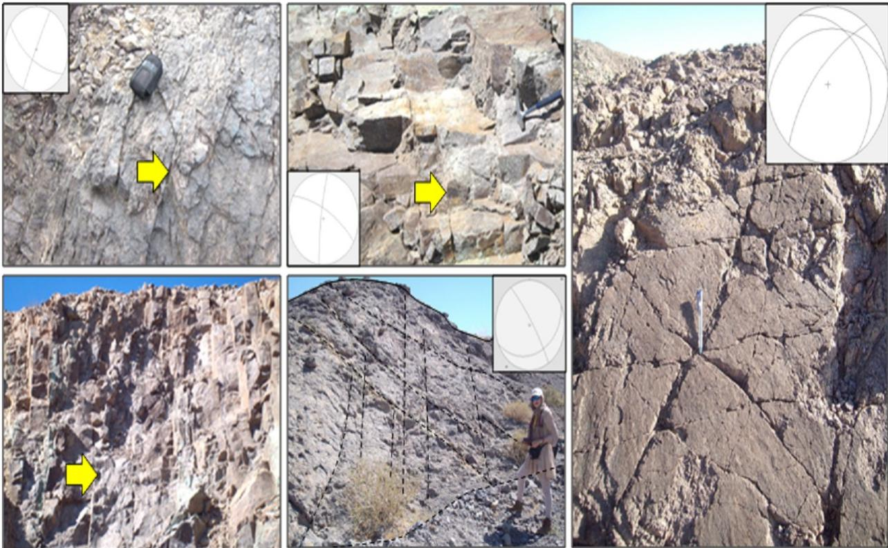
Figure 6. View of the joints of the Gazkhizan area. The status of their plates can be seen in stereographic diagrams.
