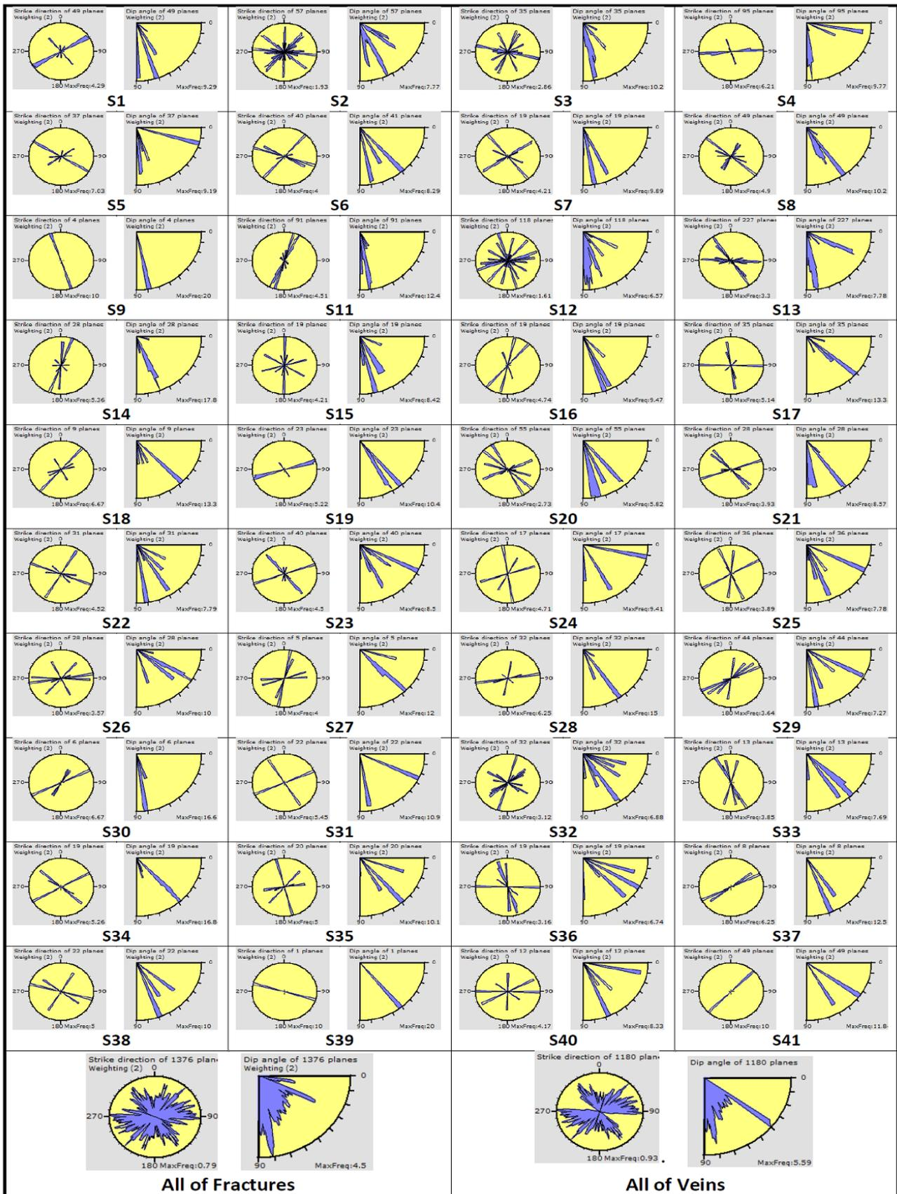
Figure 4. Diagrams of the directional rose and the slope value of fractures in the Gazkhizan region by geological stations and general data of fractures and types of mineralized fractures.
