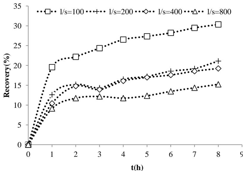
Figure 1. Effect of l/s ratio on the gold thiosulfate complexes recovery by activated carbon. Gold concentration= 2mg/l, pH=10 and T=25°C
