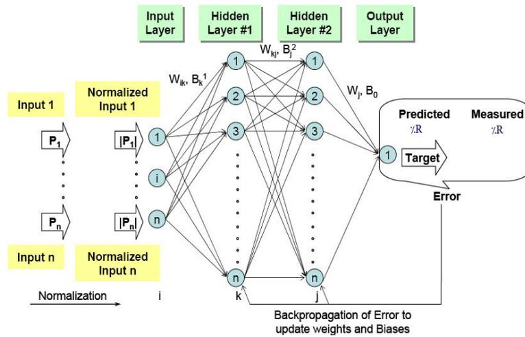
Figure 8. A neural network with feed forward back propagation algorithm
