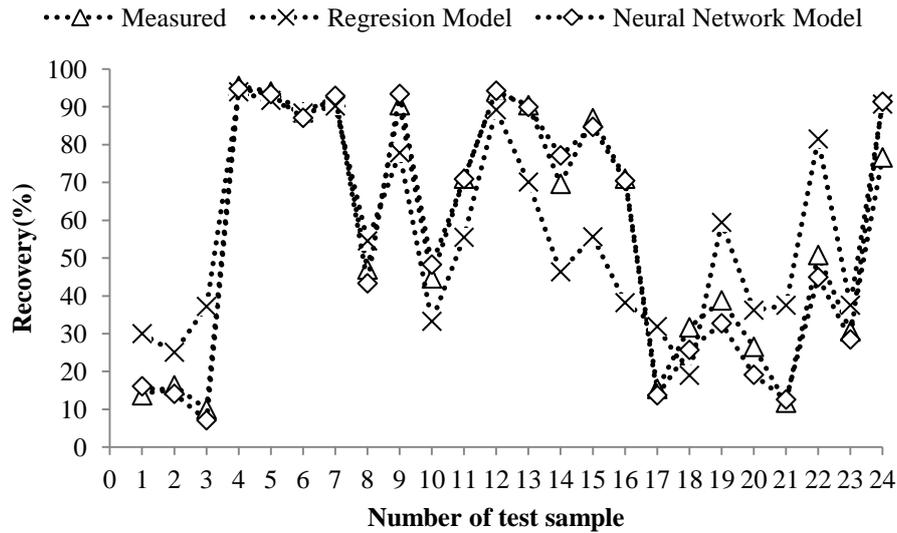
Figure 15. Comparison between measured and predicted recovery of gold on activated carbon for different type of pattern
