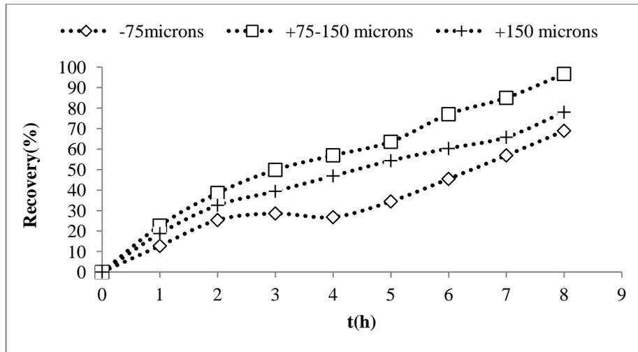
Figure 6. Effect of sizes of activated carbon. gold concentration= 2mg/l, T=45°C, l/s=100 and pH=10.5
