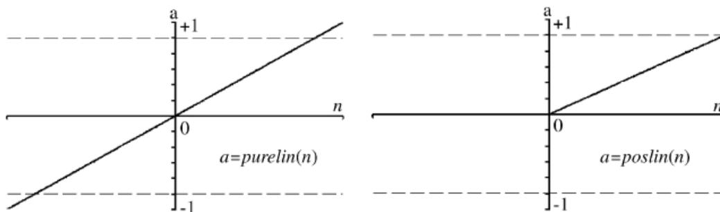
Figure 10. Linear transfer functions
