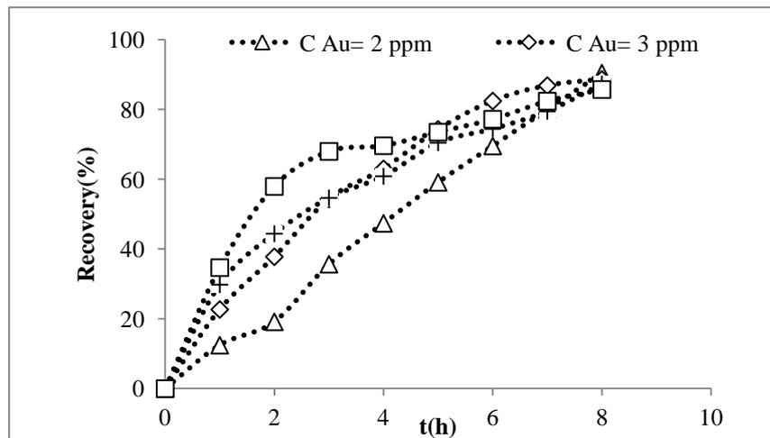
Figure 5. Effect of initial gold concentration. T=45°C, l/s=100 and pH=10.5
