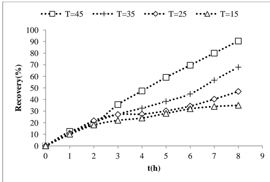
Figure 2. Temperature effect on the gold thiosulfate complex recovery by activated carbon. Gold concentration= 2 mg/l, pH=10 and l/s=100
