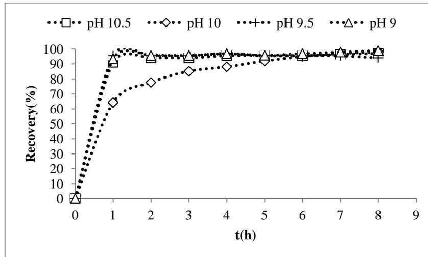
Figure 4. PH effect on the gold thiosulfate complex recovery by activated carbon. Gold concentration= 1.0 mg/l, T=25°C and l/s= 50
