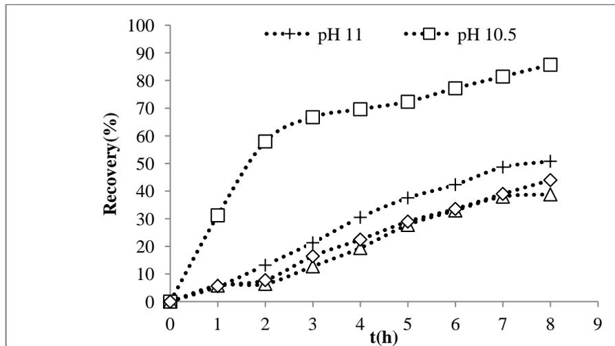
Figure 3. PH effect on the gold thiosulfate complex recovery by activated carbon. Gold concentration= 5mg/l, T=45°C and l/s=100
