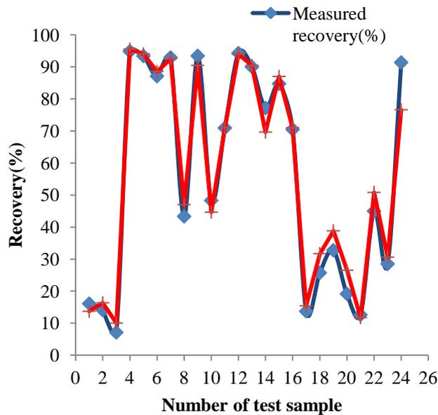
Figure 12. Comparison between measured and predicted recovery of gold on activated carbon for different type of pattern
