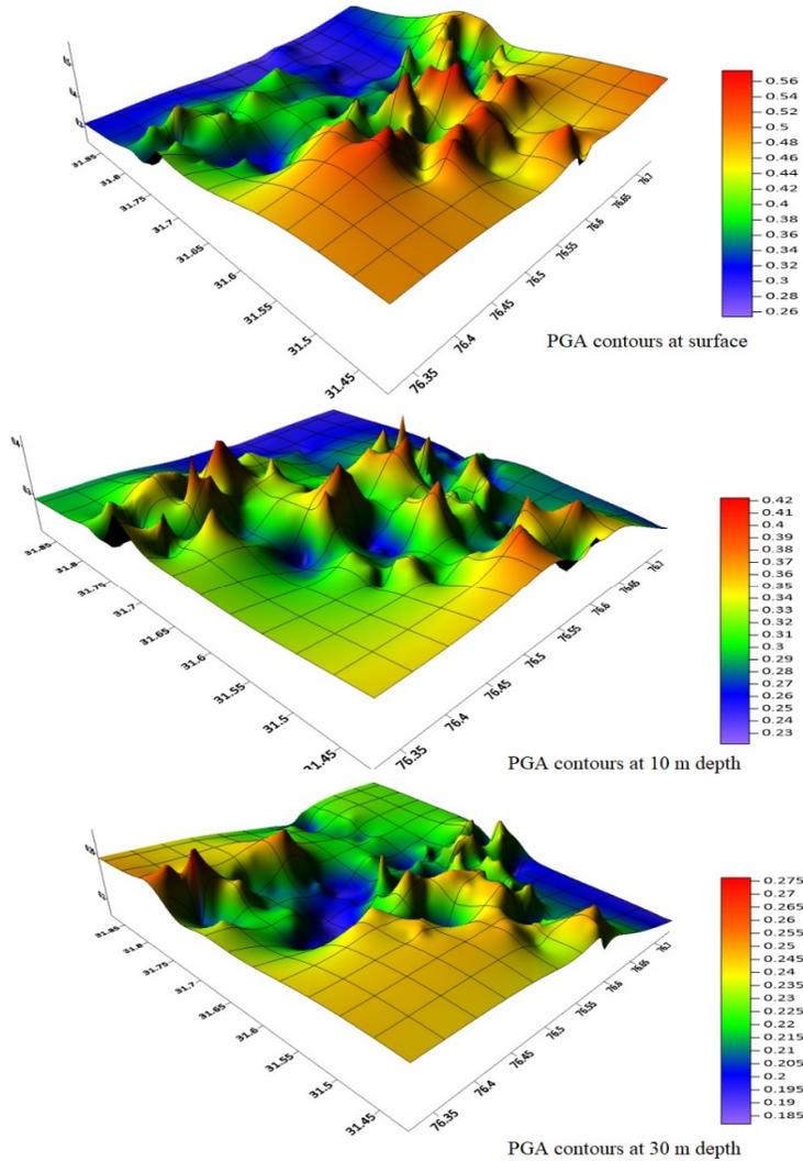
Figure 9. 3D PGA contours at surface, 10 m, and 30 m depth for El Centro earthquake.
