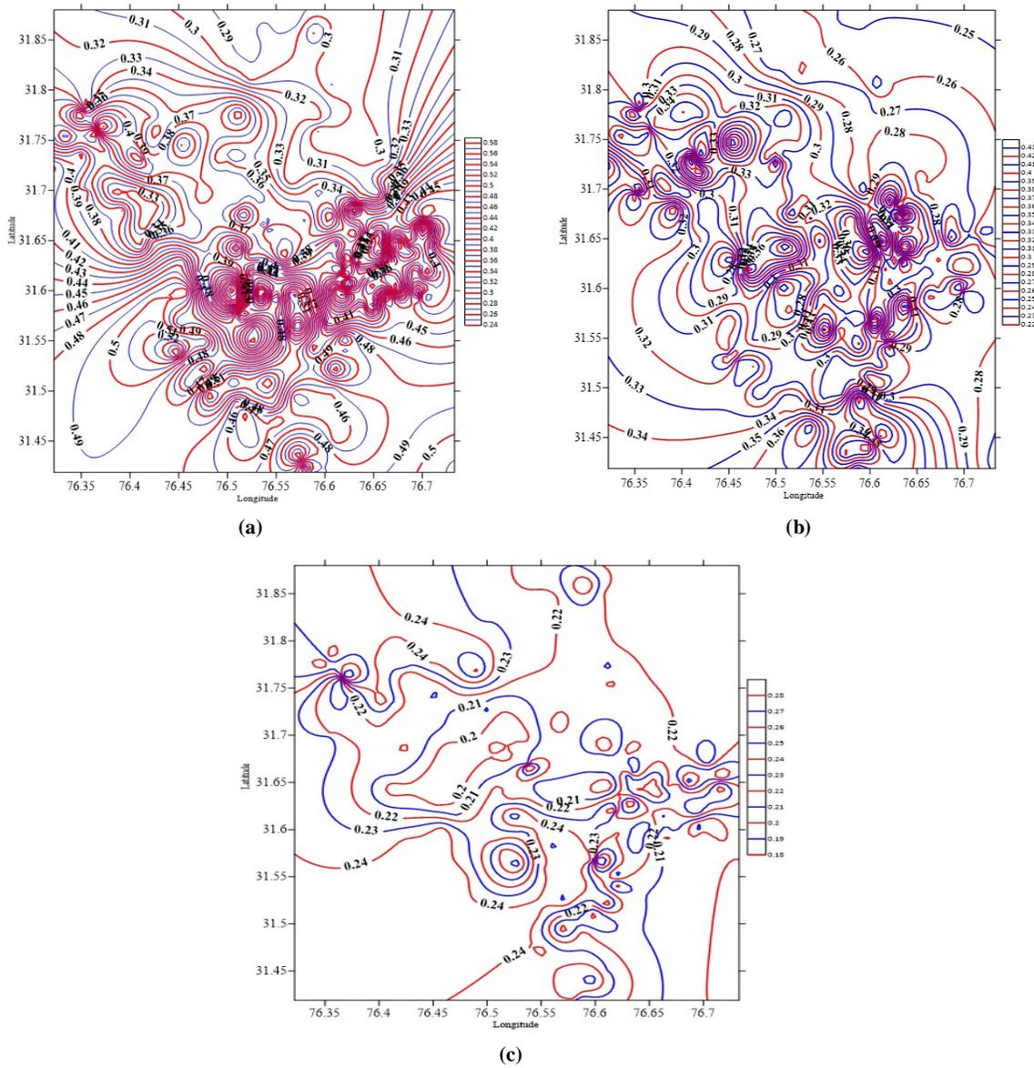
Figure 8. PGA contours for El Centro earthquake: (a) at surface, (b) 10 m depth, and (c) 30 m depth.
