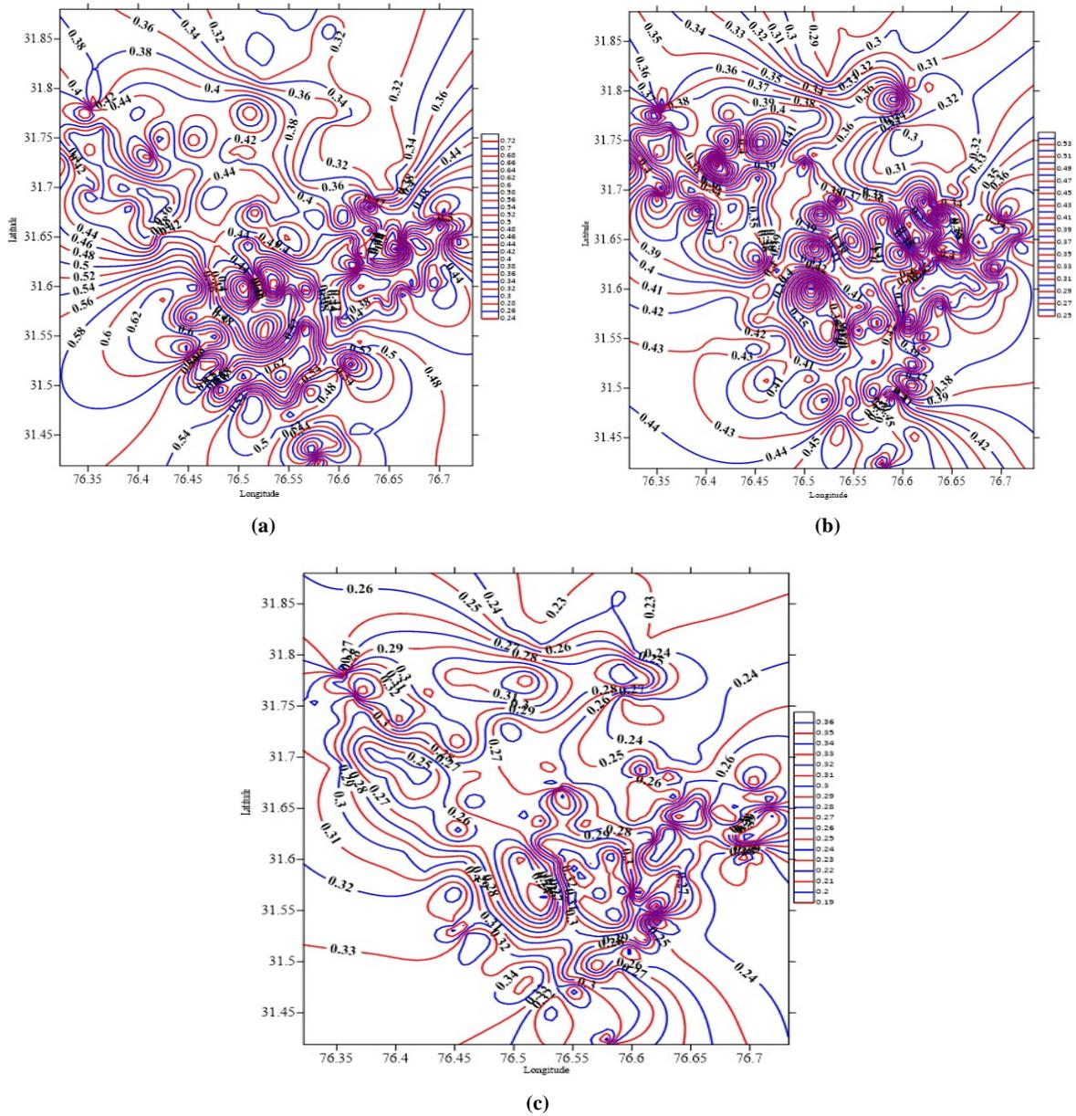
Figure 12. PGA contours for Petrolia earthquake: (a) at surface, (b) 10 m depth, and (c) 30 m depth.
