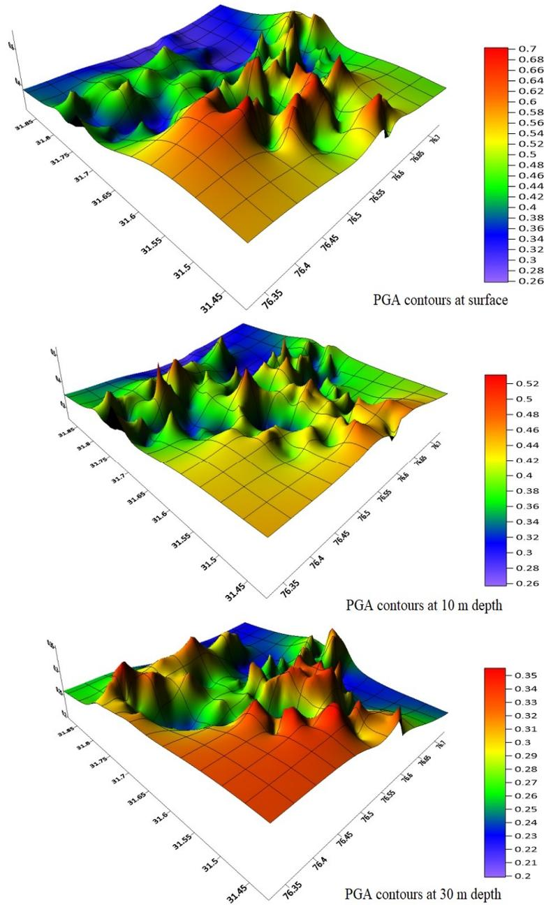
**Figure 13. 3D PGA contours at surface, 10 m, and 30 m depth for Petrolia earthquake.**
