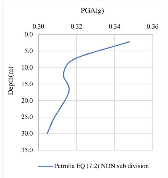
Figure 7 (c). Typical profile of borehole No. 34 (Nadaun).
