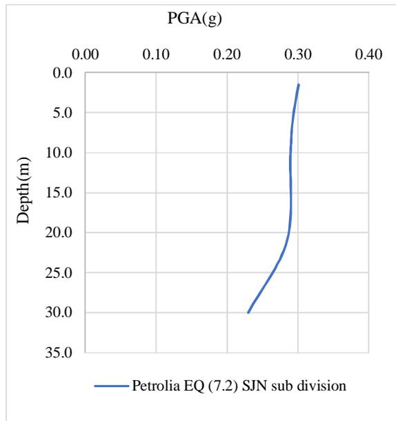
Figure 7 (d). Typical profile of borehole No. 10 (Sujanpur).
