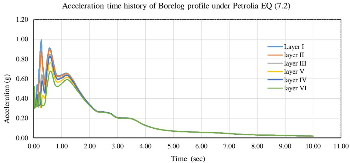
**Figure 6. Typical acceleration time history of typical borehole (No. 34) profile of Nadaun sub-division.**
