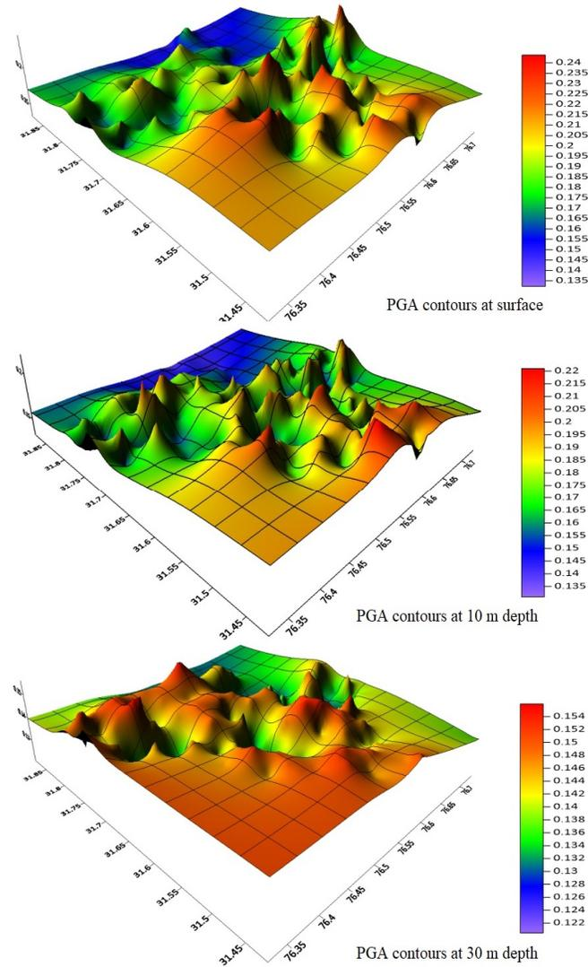
Figure 11. 3D PGA contours at surface, 10 m, and 30 m depth for Loma Prieta earthquake.
