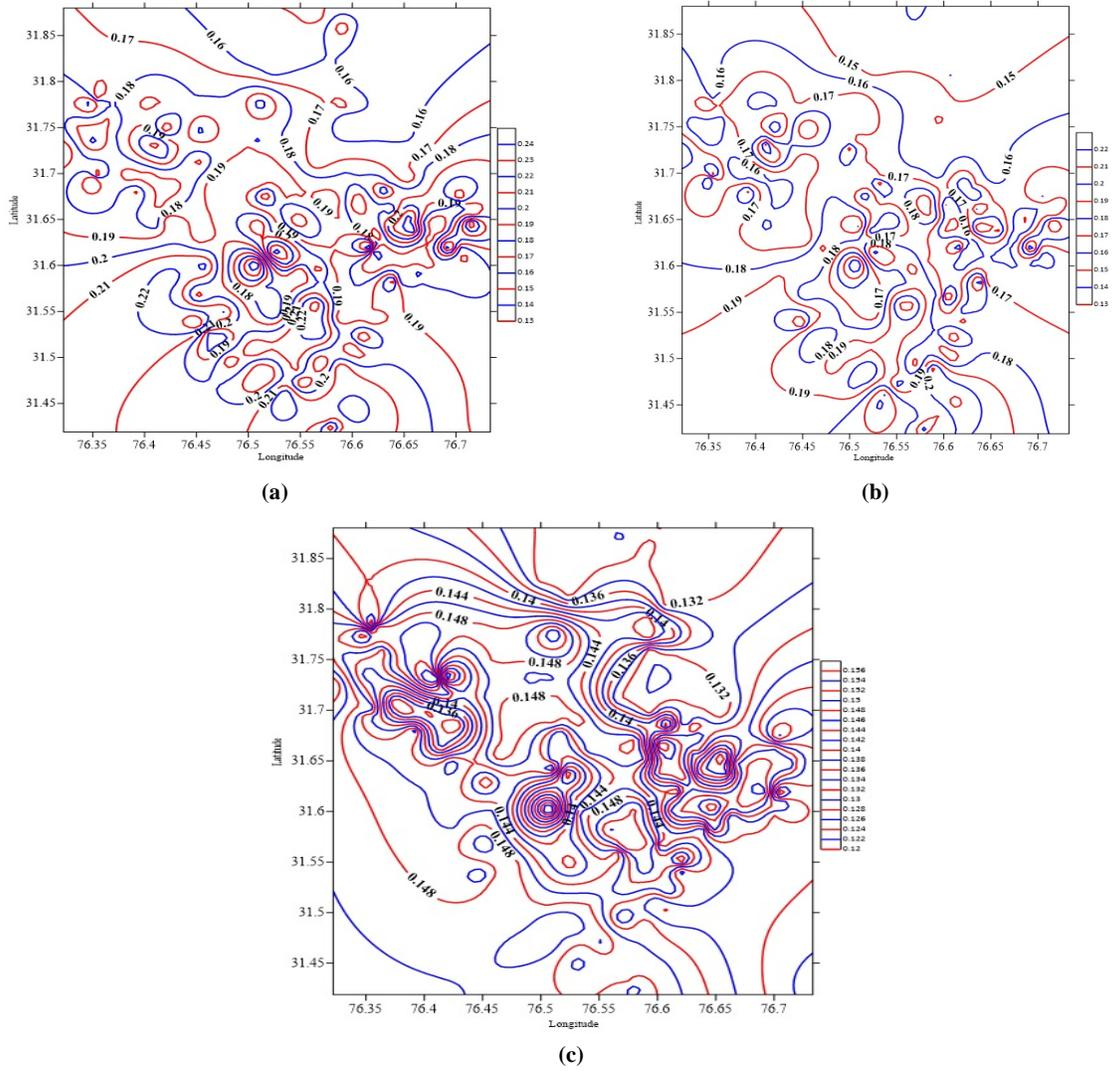
Figure 10. PGA contours for Loma Prieta earthquake: (a) at surface, (b) 10 m depth, and (c) 30 m depth.
