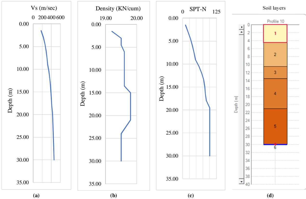
**Figure 2. Typical variation of input parameters in borehole 34 of Nadaun sub-division (a) shear wave velocity (b) density (c) SPT-N values (d) soil layers and water table level.**
