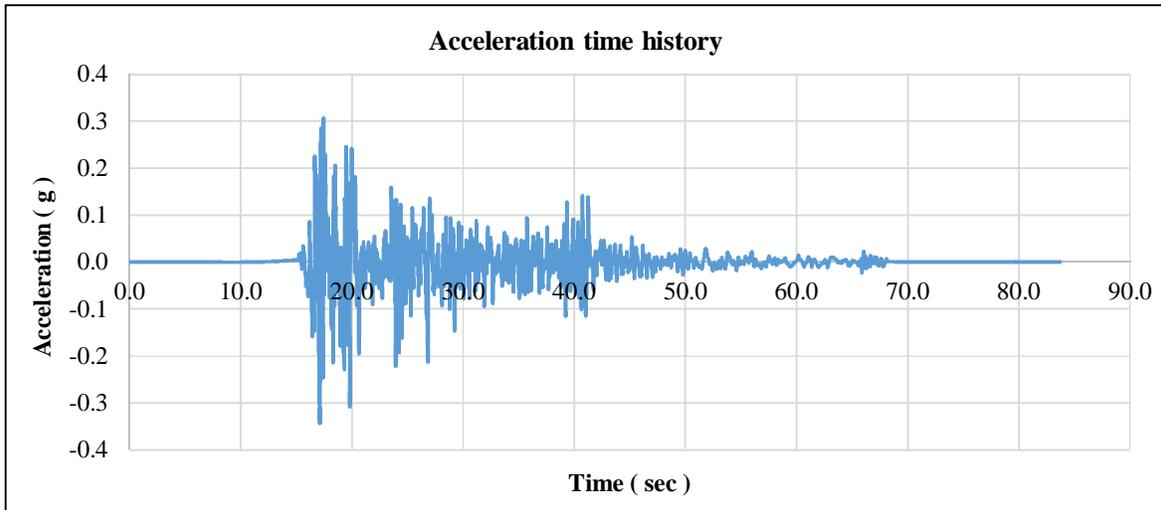
Figure 3. El Centro earthquake–input acceleration time history.
