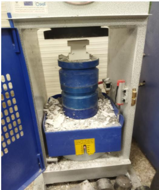
**Figure 3. Uniaxial loading frame.**
