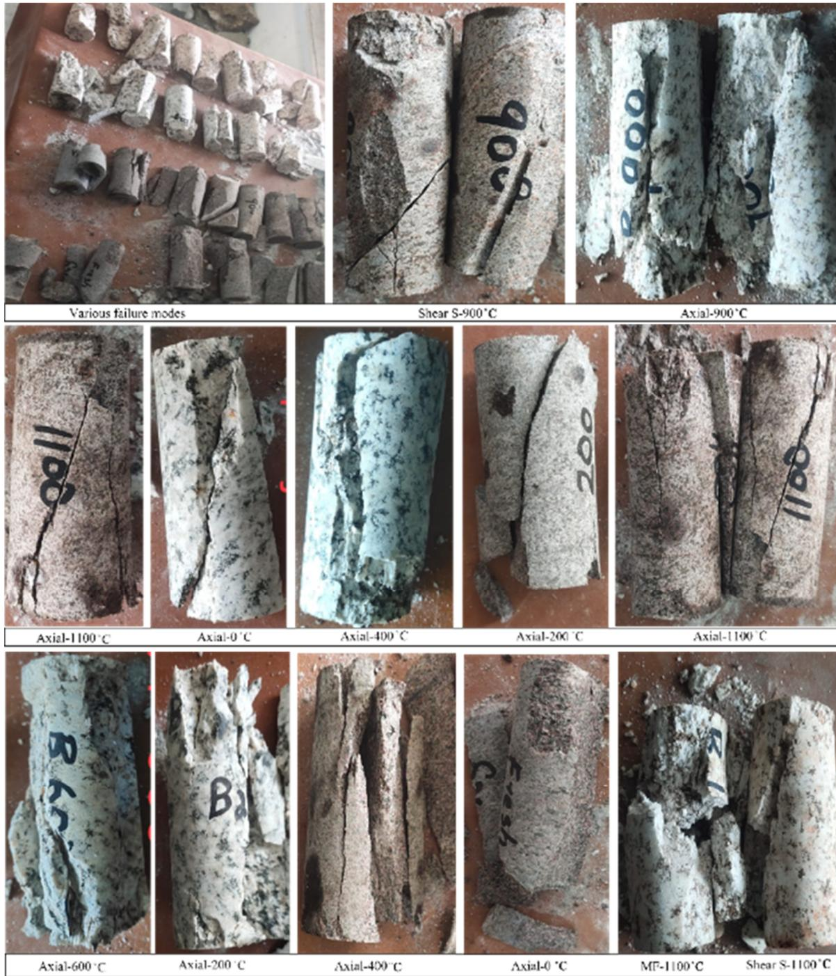
Figure 12. Failure modes of granite observed under uniaxial compression at different temperatures.
