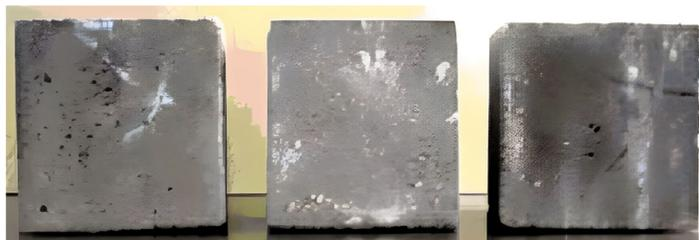
**Figure 2.** Rubberised copper slag based geo-polymer mortar.
