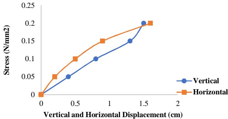
Figure 7. Stress vs.  $\Delta V$  and  $\Delta H$  values for slope with LDPE geo-composite facing, spacing 200 mm (10 mm).
