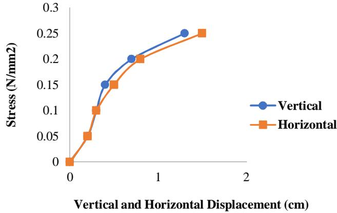
Figure 15. Stress vs  $\Delta V$  and  $\Delta H$  values for slope with LDPE geo-composite facing, spacing 200 mm (12 mm).
