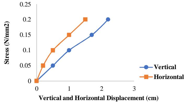
Figure 11. Stress vs  $\Delta V$  and  $\Delta H$  values for slope with diamond-shaped aluminium wire mesh, spacing 200 mm (10 mm).
