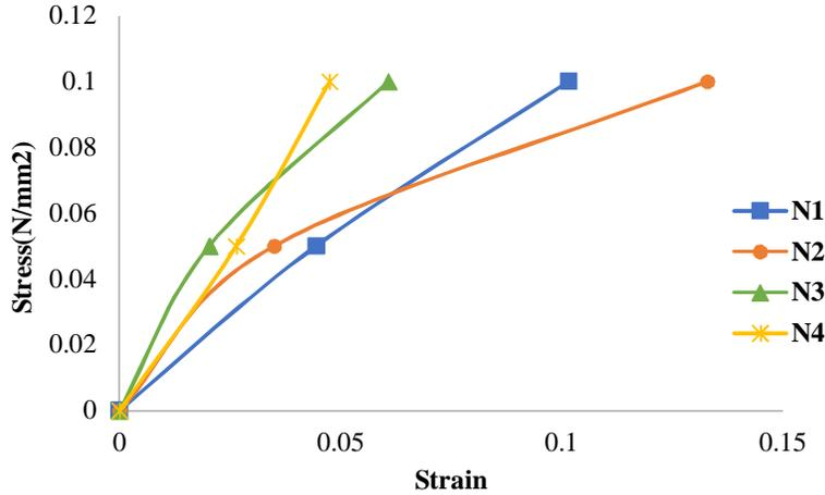
Figure 4. Stress vs. strain values for slope without facing, spacing 200 mm (10 mm).
