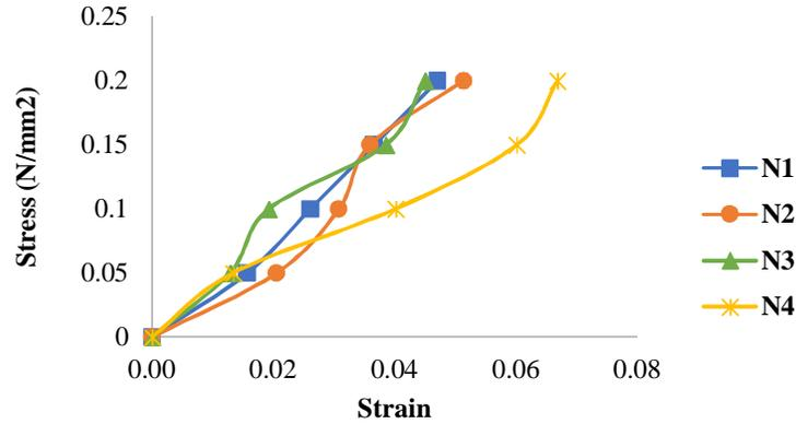
Figure 10. Stress vs strain values for slope with diamond-shaped aluminium wire mesh, spacing 200 mm (10 mm).
