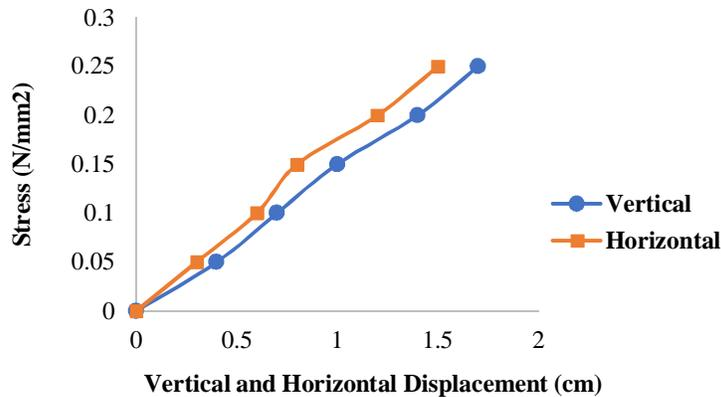
Figure 17. Stress vs  $\Delta V$  and  $\Delta H$  values for slope with galvanized iron facing, spacing 200 mm (12 mm).
