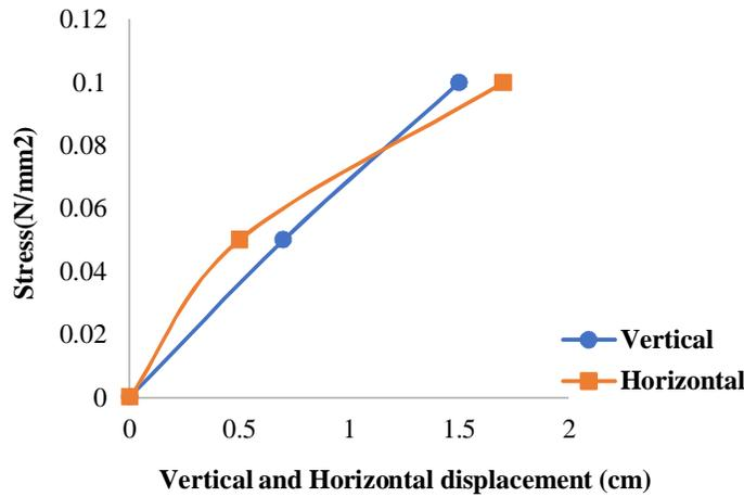
Figure 5. Stress vs.  $\Delta V$  and  $\Delta H$  values for slope without facing, spacing 200mm (10mm).
