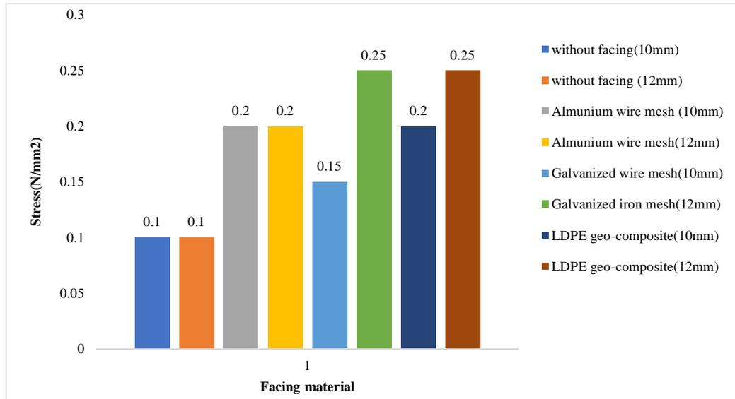
Figure 20. Comparison of facing materials with 10 mm and 12 mm diameter nails.
