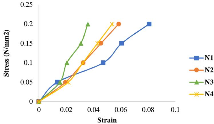
Figure 6. Stress vs. strain values for slope with LDPE geo-composite facing, spacing 200 mm (10 mm).
