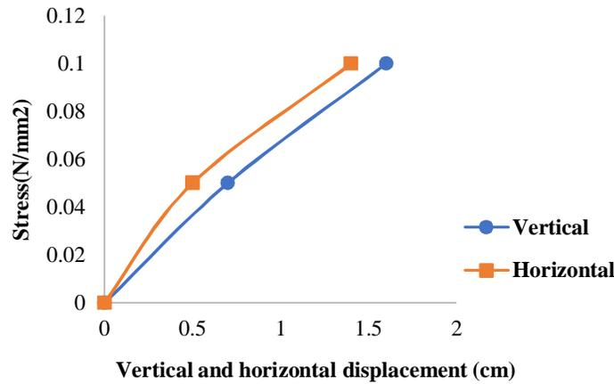
Figure 13. Stress vs  $\Delta V$  and  $\Delta H$  values for slope without facing, spacing 200 mm (12 mm).
