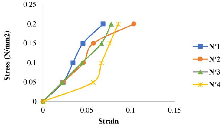
Figure 18. Stress vs strain values for slope with diamond-shaped aluminium wire mesh, spacing 200 mm (12 mm).
