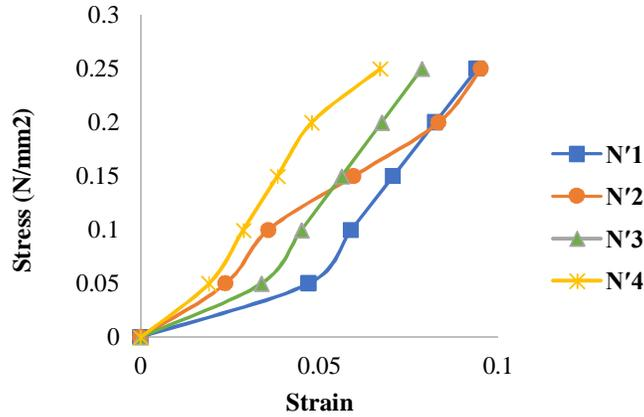
Figure 14. Stress vs strain values for slope with LDPE geo-composite facing, spacing 200 mm (12 mm).
