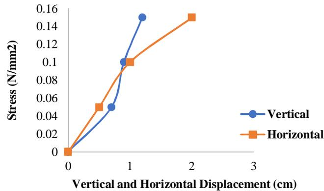
Figure 9. Stress vs  $\Delta V$  and  $\Delta H$  values for slope with galvanized iron facing, spacing 200 mm (10 mm).
