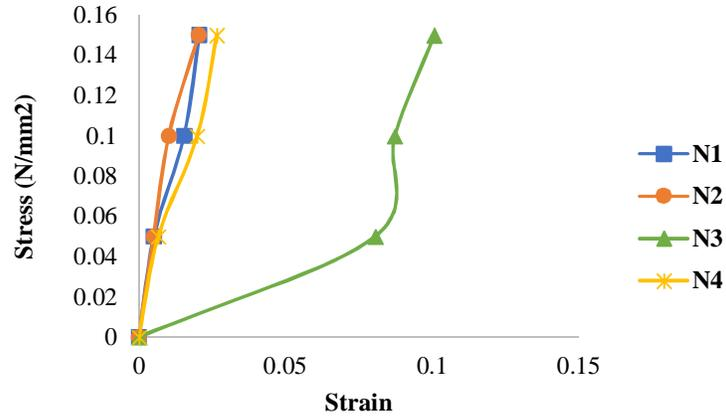
Figure 8. Stress vs strain values for slope with galvanized iron facing, spacing 200 mm (10 mm).
