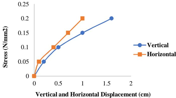
Figure 19. Stress vs  $\Delta V$  and  $\Delta H$  values for slope with diamond-shaped aluminium wire mesh, spacing 200 mm (12 mm).
