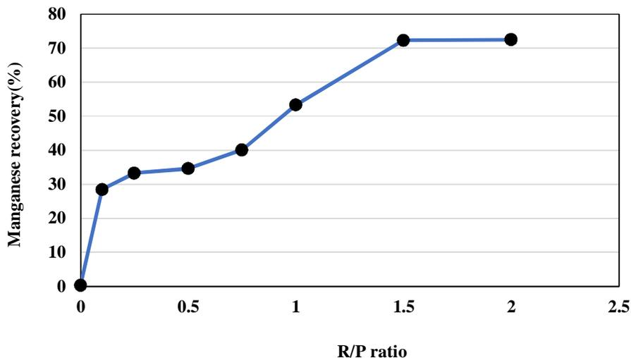
Figure 5. Effect of R/P on manganese recovery from pyrolusite in the sulfuric acid of 1.5 M, 70 °C, and 4 h.
