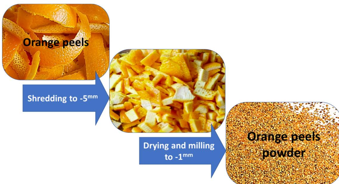
Figure 1. Orange peel powder (as reductant) preparation.
