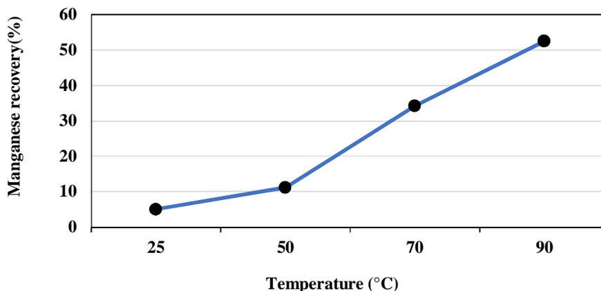
Figure 4. Effect of temperature on manganese recovery from pyrolusite in the sulfuric acid concentration of 1.5 M, R/P of 0.5 (w/w), and 4 h.
