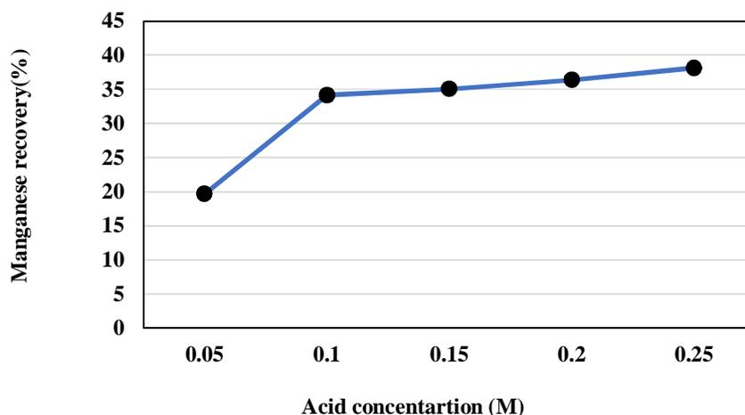
Figure 3. Effect of sulfuric acid concentration on manganese recovery from pyrolusite in 70 °C, R/P of 0.5 (w/w), and 4 h.
