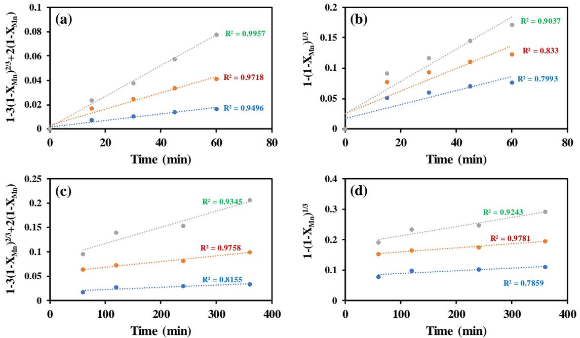
Figure 7. Kinetic data plot based on the shrinking core model at three temperatures of 50 °C (blue line), 70 °C (red line), and 90 °C (green line) in the range of 0 to 60 min (a) diffusion through the product layer, (b) chemical reaction, and the range of 60 to 360 min (c) diffusion through the product layer, (d) chemical reaction.
