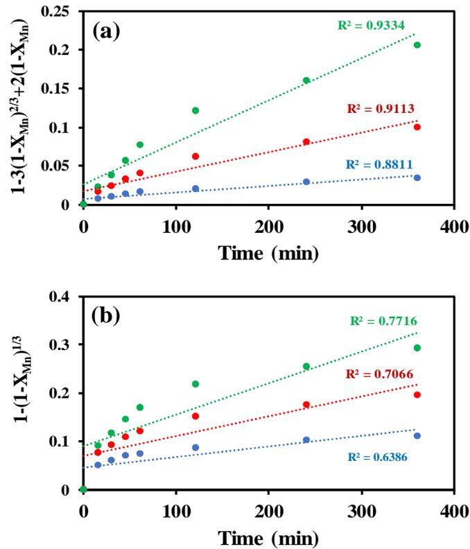
**Figure 6.** Kinetic data plot based on the shrinking core model at three temperatures of 50 °C (blue line), 70 °C (red line) and 90 °C (green line) (a) diffusion through the product layer, (b) chemical reaction.
