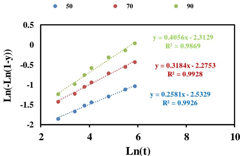
**Figure 8.** Plotting kinetic data based on the Avrami model at three temperatures of 50 °C (blue line), 70 °C (red line), and 90 °C (green line).
