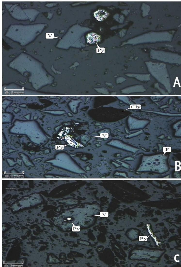
Figure 3. Polarized light microscope images of Tabas coal samples: A) PE, B) B<sub>4</sub>C<sub>1</sub>, C) B<sub>4</sub>B<sub>2</sub>. Py: Pyrite, Cly: Clay Minerals, F: Fusinite, V: Vitritinite.
