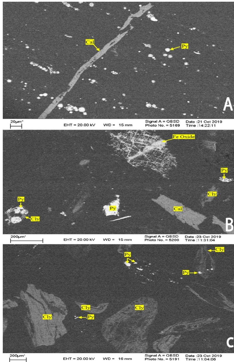
**Figure 2. Scanning electron microscope (SEM) images of Tabas coal samples: A) PE, B) B<sub>4</sub>C<sub>1</sub>, C) B<sub>4</sub>B<sub>2</sub>, Py: Pyrite, Cal: Calcite, Fe-oxide: Iron oxide minerals, Cly: Clay Minerals.**
