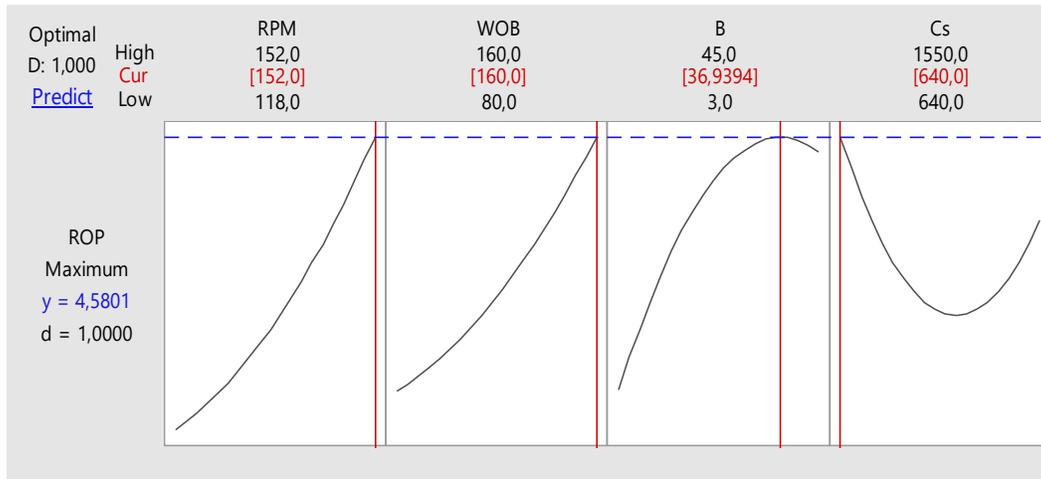
Figure 10. Response optimization plot for penetration rate in rotary drilling.
