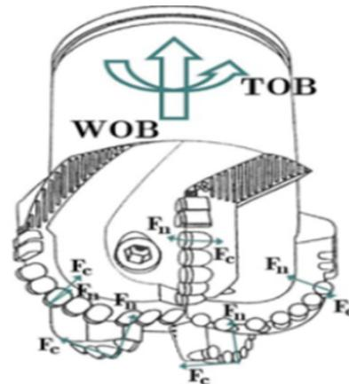
Figure 2. PDC drill tool and forces on tool [14].
