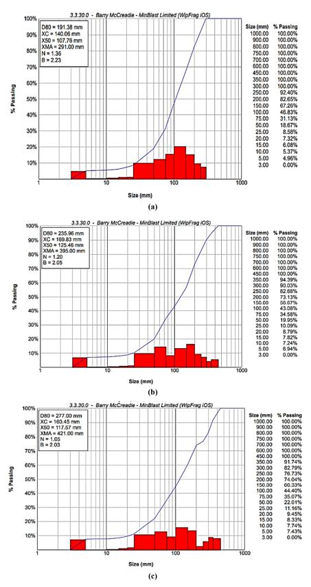
Figure 3. Fragmentation analysis result with size distribution rate.
