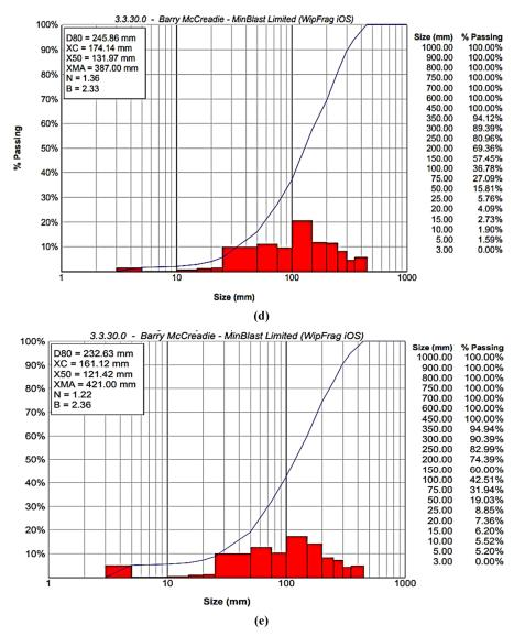
Continuous of Figure 3. Fragmentation analysis result with size distribution rate.
