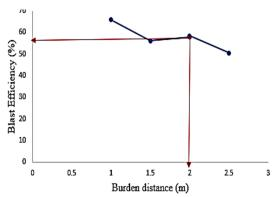
Figure 4. Relationship between blast efficiency and burden distance.
