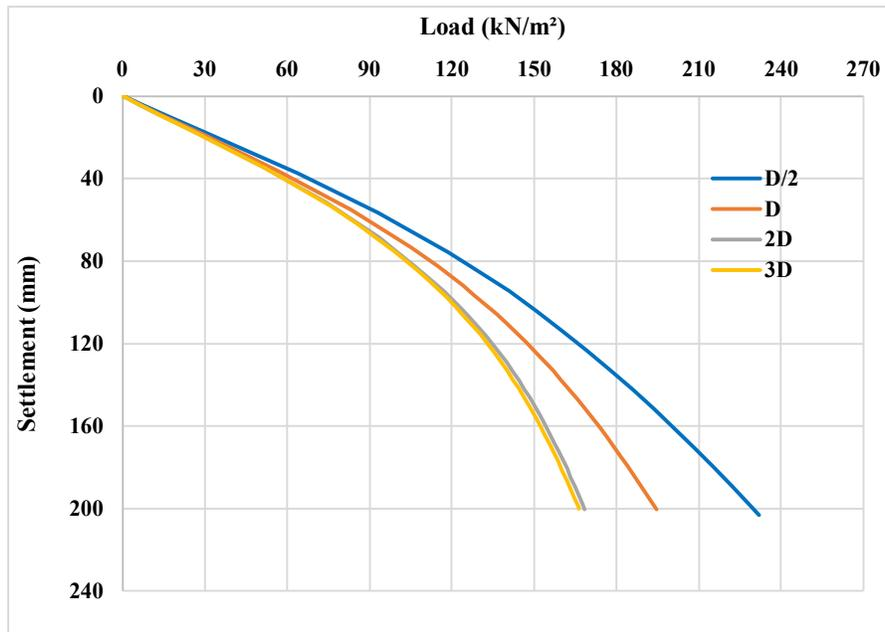
Figure 13. Comparative load settlement plot.
