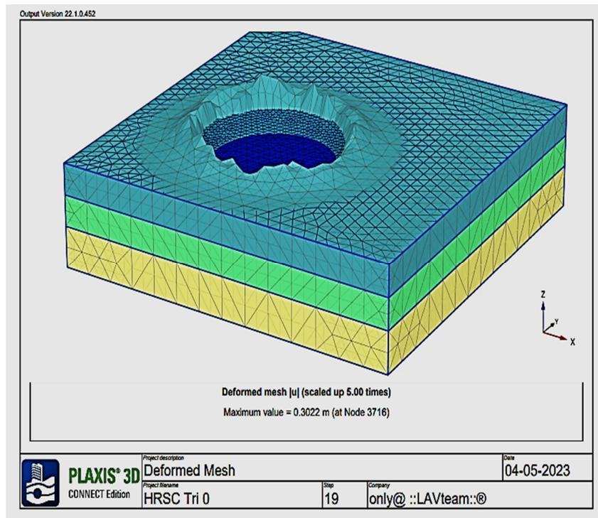
Figure 2. Deformed mesh of raft footing on layered soil.
