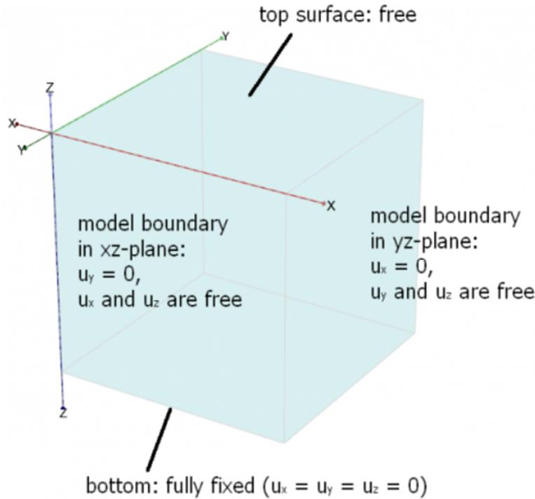
**Figure 1b. Boundary conditions of the model.**
