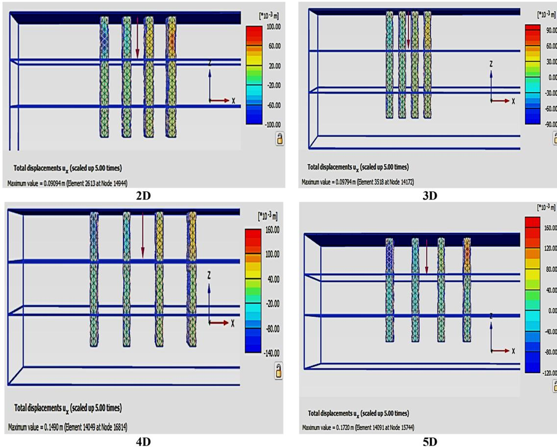
Figure 10. Displacement contours of stone columns in square arrangement with spacing ranging 2D to 5D.
