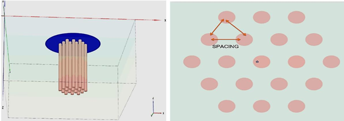
Figure 5. Stone columns arranged triangularly.
