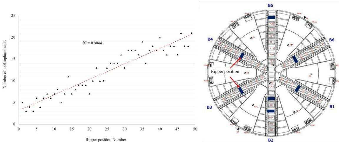
Figure 11. Relation between cutter position and cutter consumption for rippers in 6500 m of Tehran metro line 7.
