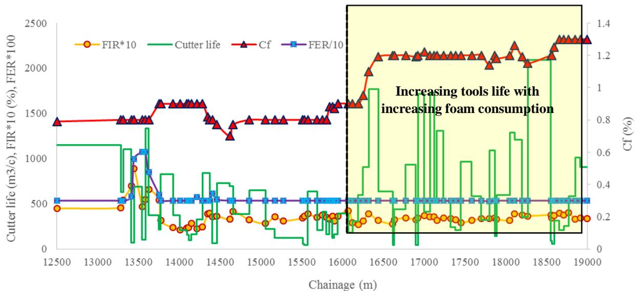
Figure 26. Variation of tool life and conditioning parameters in Tehran metro line 7.
