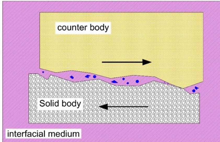
Figure 1. Components of a tribological system [3].
