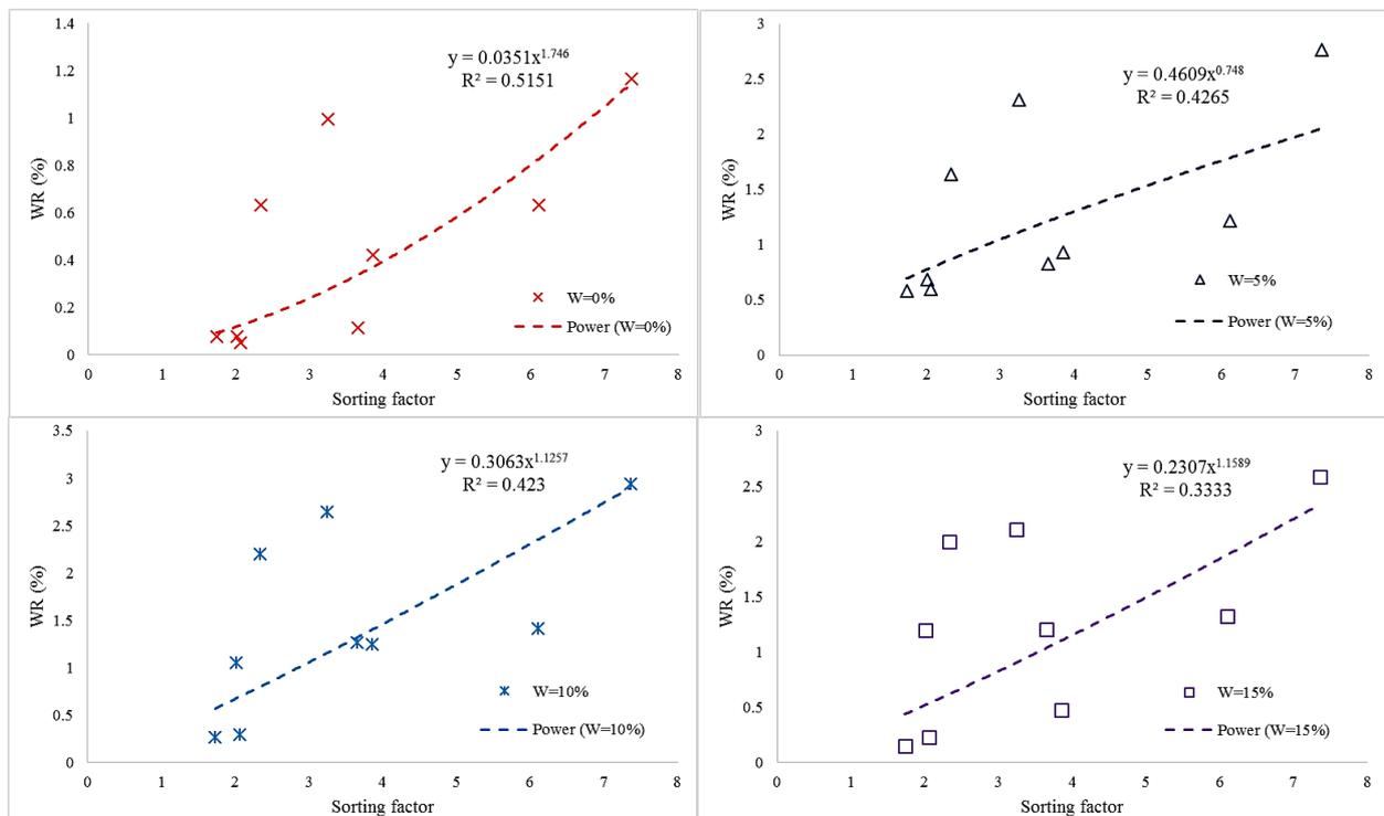
Figure 19. Effect of soil sorting on the wear at 0, 5, 10, and 15% moisture.
