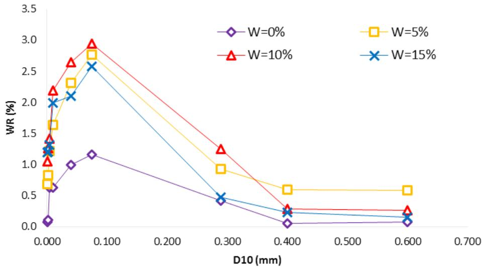
Figure 12. Correlation of D<sub>10</sub> and WR.
