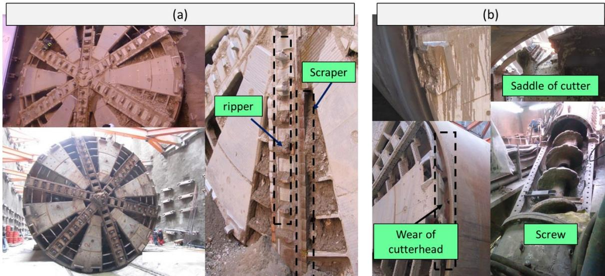
Figure 2. Types of wear: a) Worn rippers and scrapers, b) Wear of screw, saddle of cutters and cutterhead.
