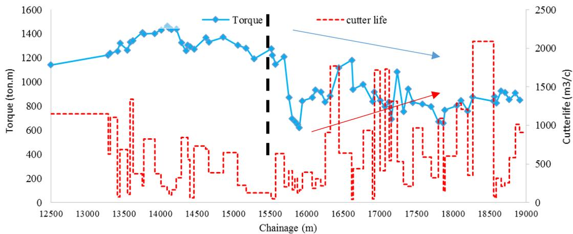
Figure 23. Variation of torque and cutter life in 6500 m of Tehran metro line 7.
