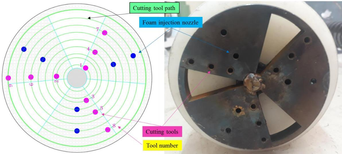
Figure 7. Cutting tools arrangement of SSAT device.
