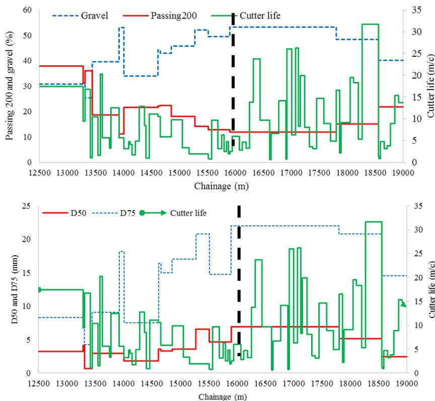
**Figure 20. Variation of grading and cutter life for Tehran metro line 7, a) distribution of gravel and passing 200, b) distribution of  $D_{50}$  and  $D_{75}$ .**
