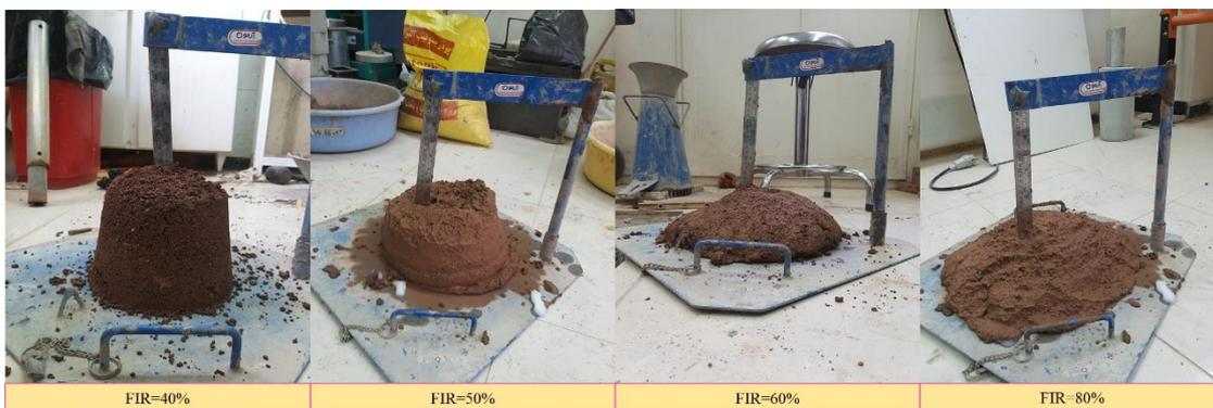
**Figure 24. Slump of materials at different FIR values.**
