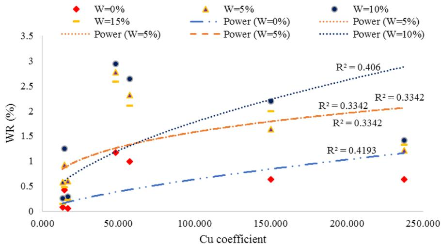
Figure 17. Relationship between the  $C_u$  and wear.
