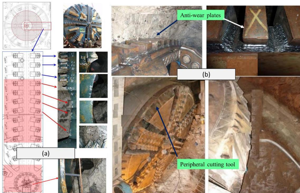
**Figure 3. Wear in Iran's tunneling projects: a) Isfahan cutterhead central tools wear, b) Shiraz cutterhead environmental tools wear [5, 6].**
