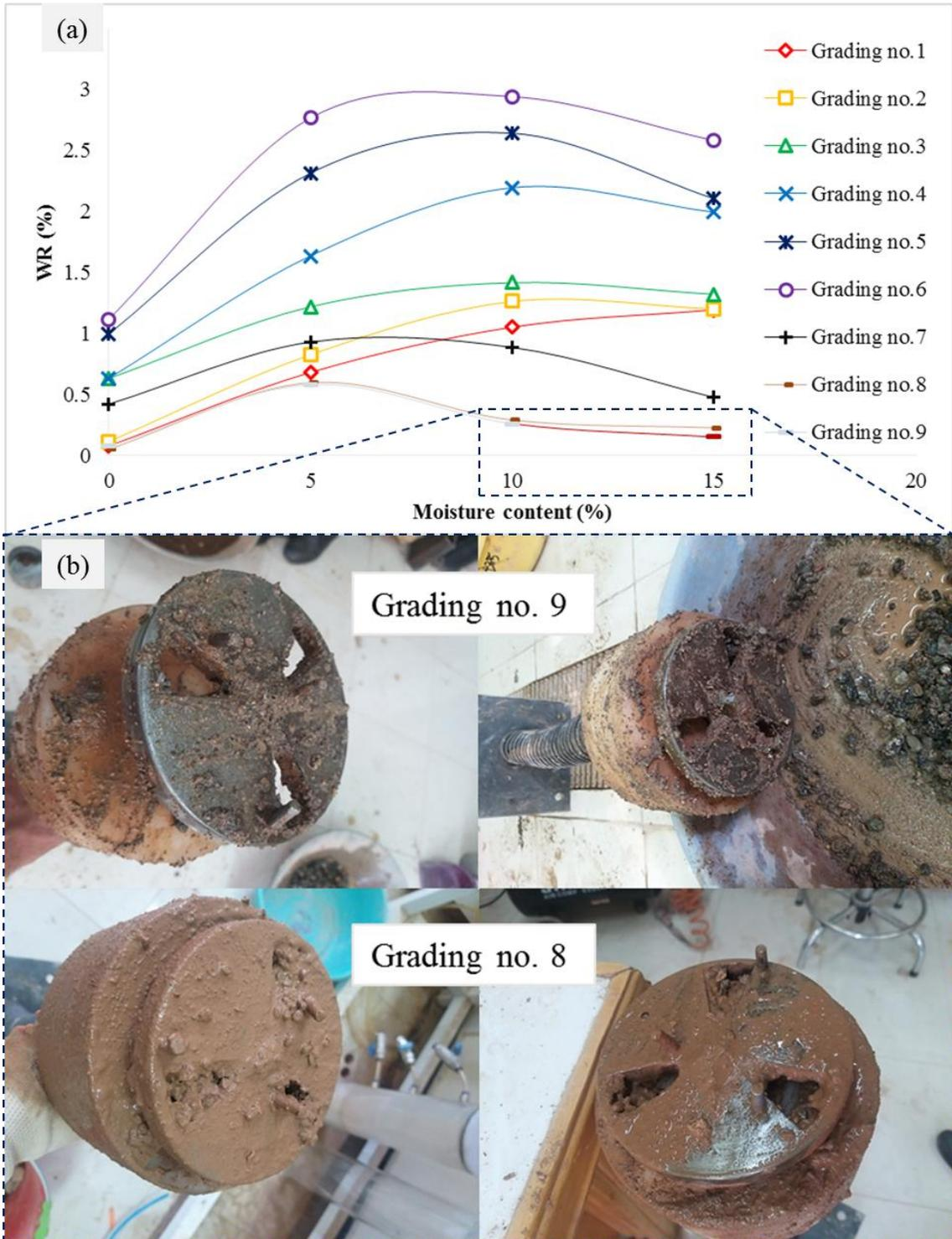
Figure 21. (a) Relationship between the moisture content values and wear and (b) propeller and cutting tools in grading No. 8 and 9: left) 15% moisture content and right) 10% moisture content.
