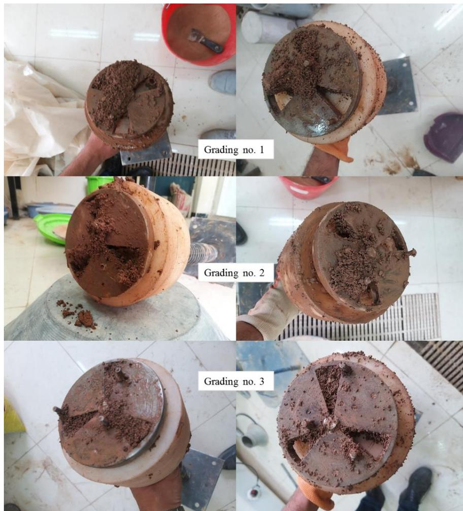
Figure 13. Clogging of propeller for grading No. 1 to 3: left) 15% moisture content and right) 10% moisture content.
