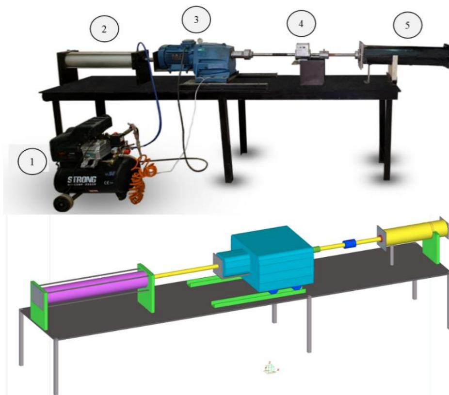
**Figure 5. SSAT testing device: 1) air compressor, 2) pneumatic jack, 3) motor and gearbox, 4) torque-meter sensor, 5) excavation chamber**
