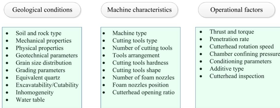
**Figure 4. Effective factors on wear of cutting tools in EPB tunneling [8].**
