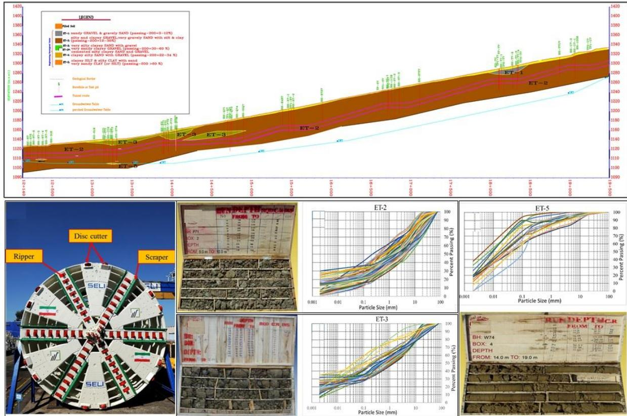
Figure 9. Additional specifications of Tehran metro line 7: a) geo-technical profile, b) picture of the EPB-TBM, and c) picture of soil samples (Left) and grain size distribution curves (Right).
