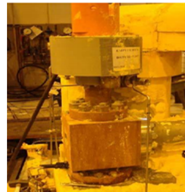
Figure 6. Sand production test device based on applying lateral stresses [28].
