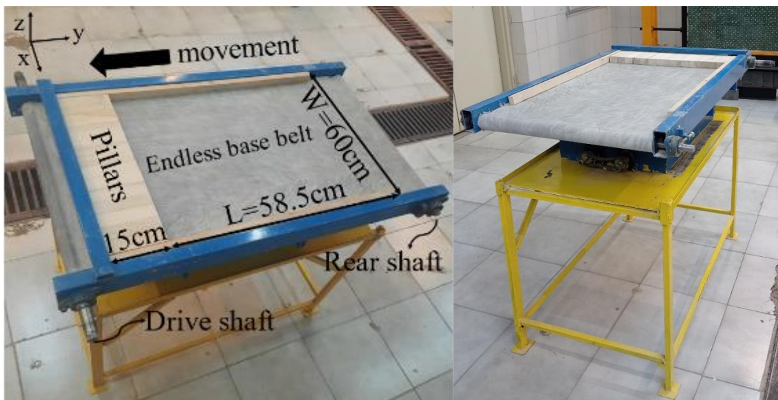
Figure 2. Base friction table used for physical modeling of the caving process
