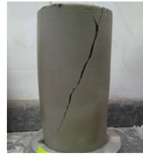
Figure 9. 2-hour specimen for the mix design number 1 after performing the uniaxial test.
