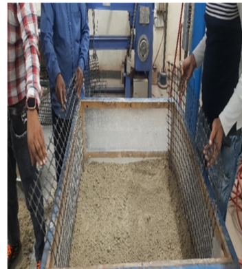
Figure 13. Filling of tailing over spread loop reinforcement in model tank
