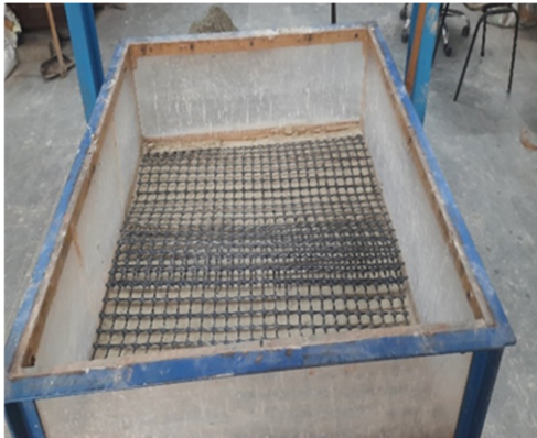
Figure10. tailing and reinforcement in the model tank
