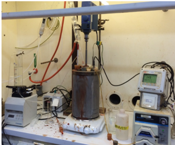
Figure 2. Atmospheric leaching test setup.
