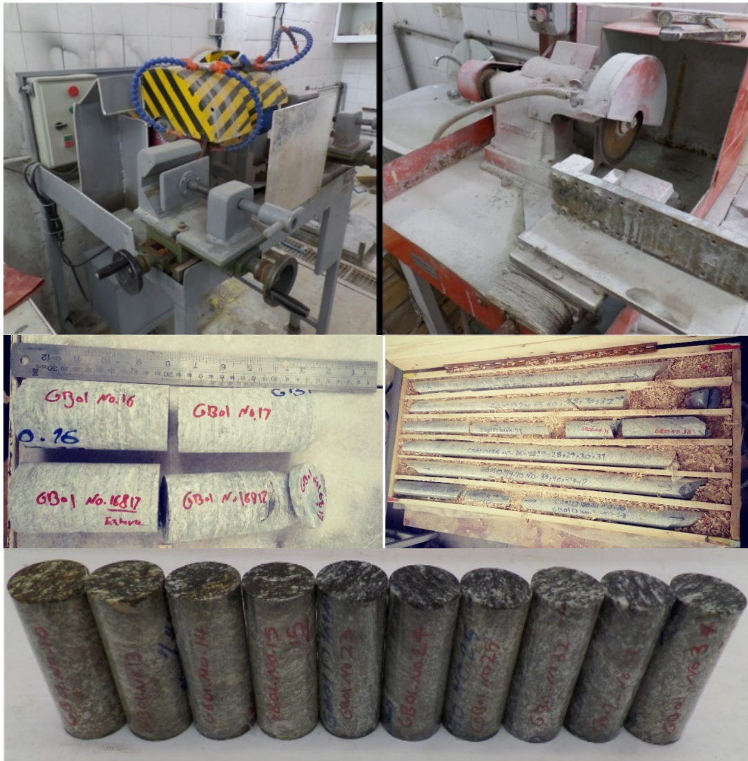
Figure 7. Transferred cores to the laboratory for preparation and testing.
