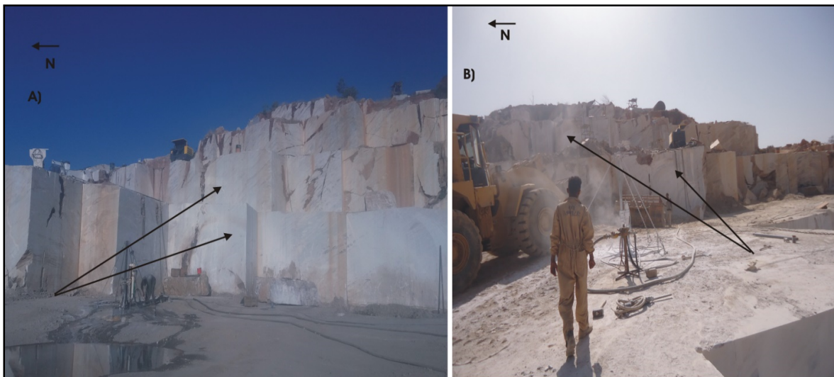
Figure 4. A) The first arrow indicates massive marble on the 3 rd and 4 th benches; B) The second arrow indicates closely spaced, jointed marble on the 1 st and 2 nd benches, and highly weathered.
