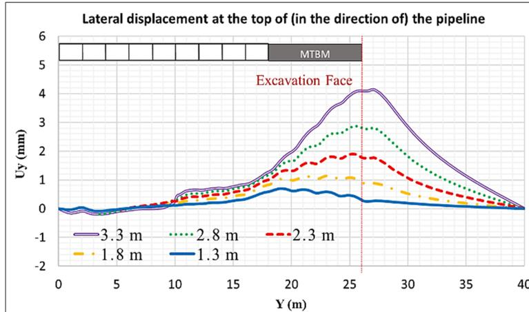
Figure 7. Longitudinal diagram of lateral deformation ( $u_y$ ) in the 26 m advance of the shield
