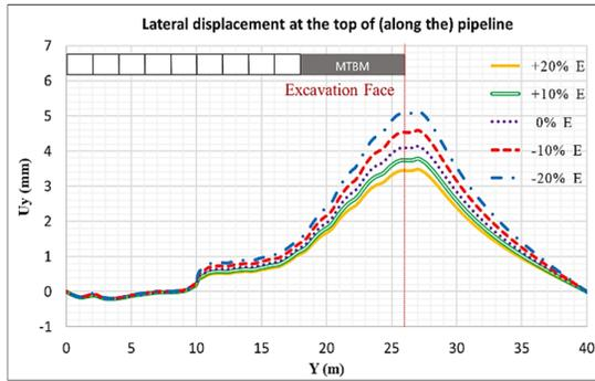
Figure 14. Lateral displacement ( $u_y$ ) in the 26m advancement of the shield
