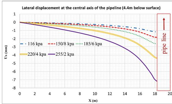
**Figure 12. Traverse diagram of lateral deformation ( $U_x$ ) in the 26 m advance of the shield**
