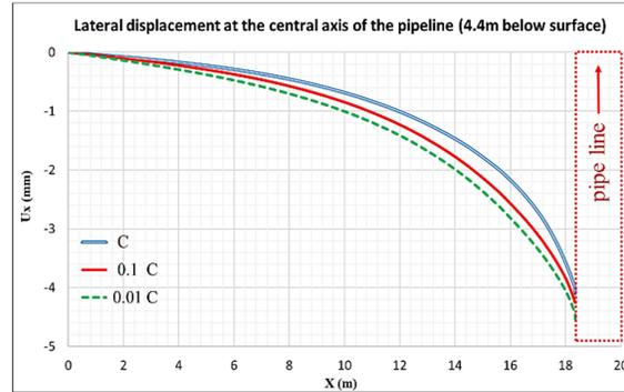
Figure 15. Traverse diagram of lateral deformation ( $U_x$ ) in the 26 m advancement of the shield
