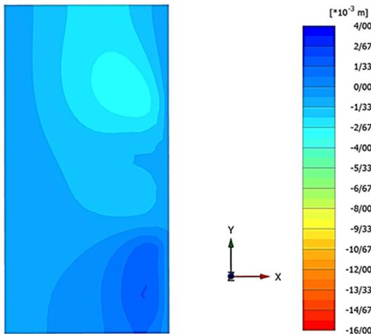
**Figure 13. Lateral displacement contour ( $U_x$ ) in the 26 m advance of the shield and ground surface**
