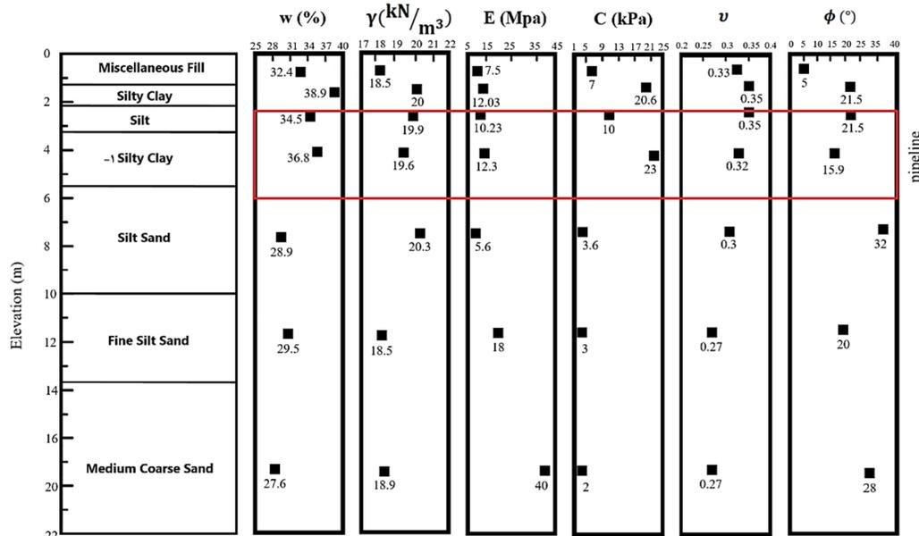
Note: w = Water content,  $\gamma$  = Soil Unit Weight, E = Elastic modulus, C = Cohesion,  $\nu$  = Poisson ratio,  $\phi$  = friction angle
