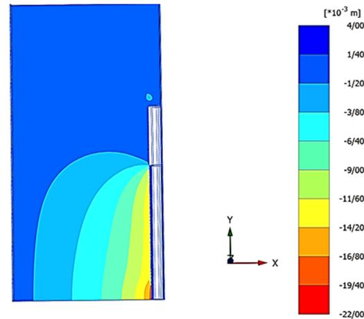
Figure 10. Longitudinal section of displacement ( $u_x$ ) at a depth of 4.4 m and injection pressure of 150 kPa
