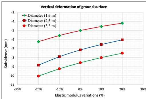
Figure 17. Simultaneous effect of diameter and Elastic modulus on ground subsidence
