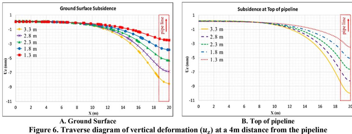
According to the observations, as the diameter of the pipe increases, the lateral displacement along the ground surface also increases. This is due to the rise in grout injection pressure and the enhanced friction and interaction between the jacked pipe and the soil, resulting in a higher displacement rate. The most significant displacement of 4.1 mm occurs at the lateral part of the pipeline, specifically in the largest diameter of 3.3 m.
