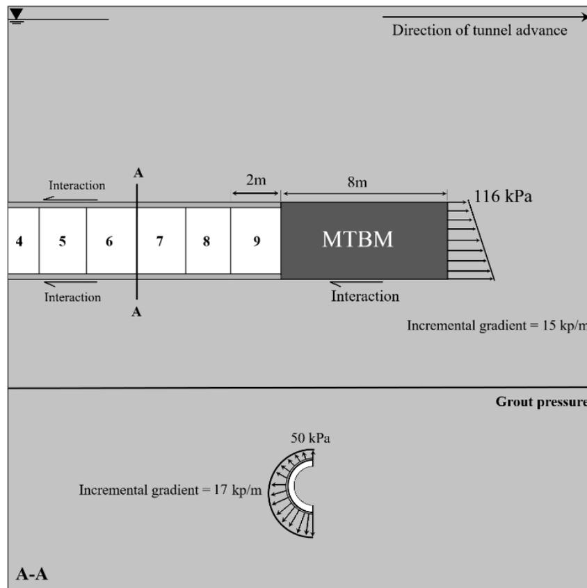
Figure 3. The details of the numerical model (Face pressure, Grout pressure)
