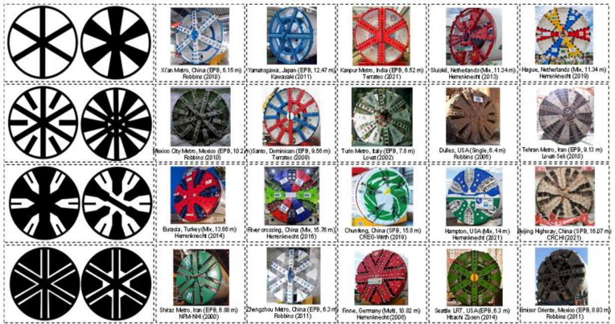
Figure A1. Different cutterhead configurations based on database for soft ground conditions
