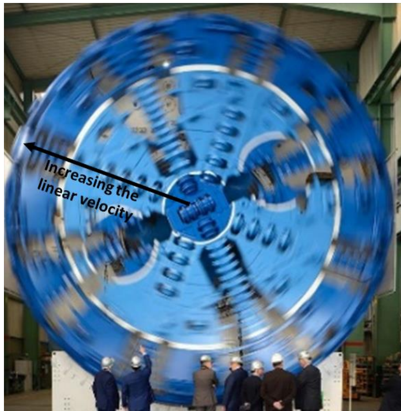
Figure 14. Schematic representation of linear velocity on cutterhead face.
