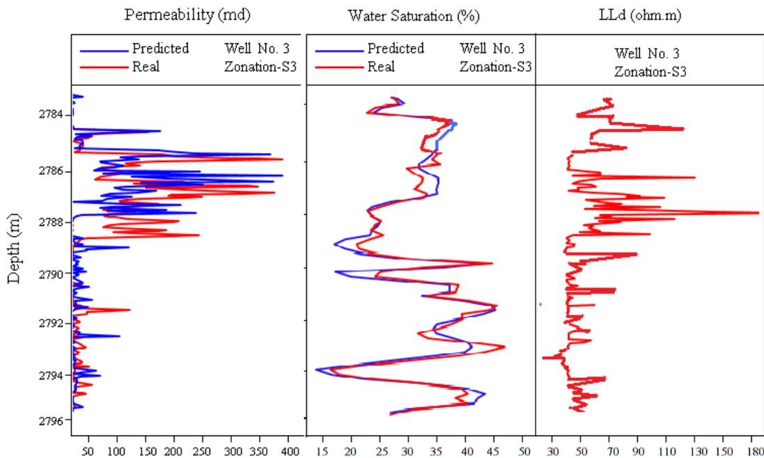
Figure 3. Results obtained from prediction of permeability and water saturation in well No.3.
