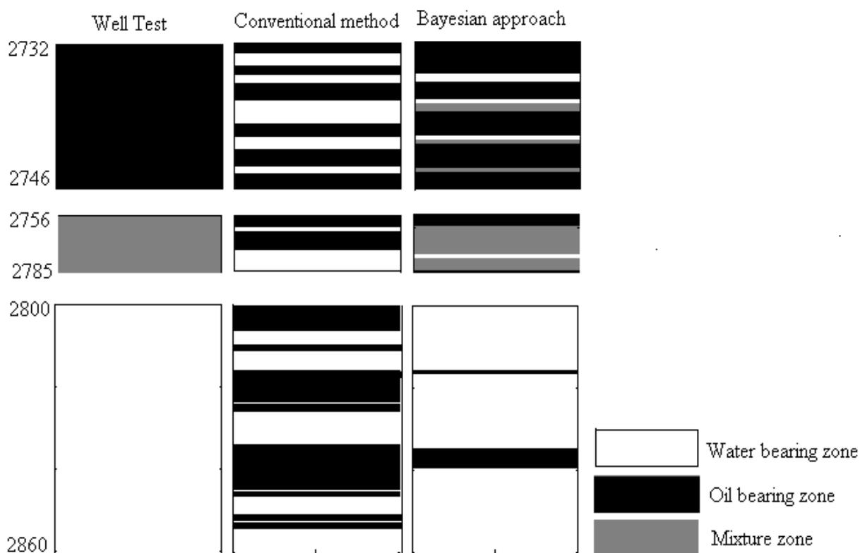
**Figure 5. Results of detecting OWC through two different approaches in well No.3.**
