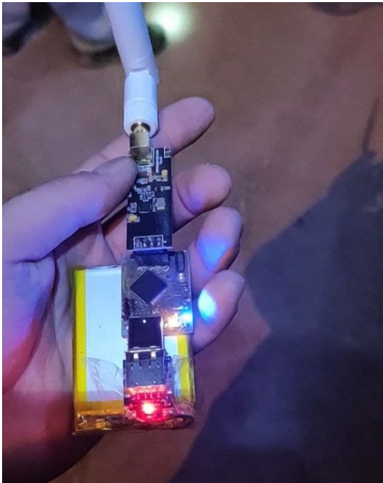
Figure 9. Designed radio module for testing data transmission in the tunnels of underground mines
