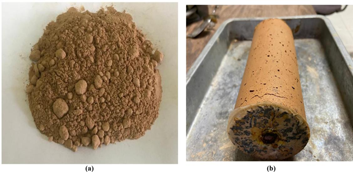
Figure 2. Images depicting (a) the soil sample before treatment and (b) the soil sample after molding and electrokinetic (EK) treatment.
