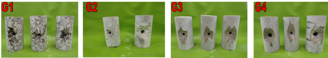
Figure 7. Fracture pits were formed in the granitic rock core specimens
