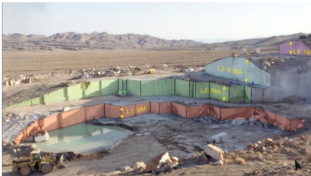
Figure 2. Leveling and segmentation of the quarry based on production steps to remove joints and fractures.
