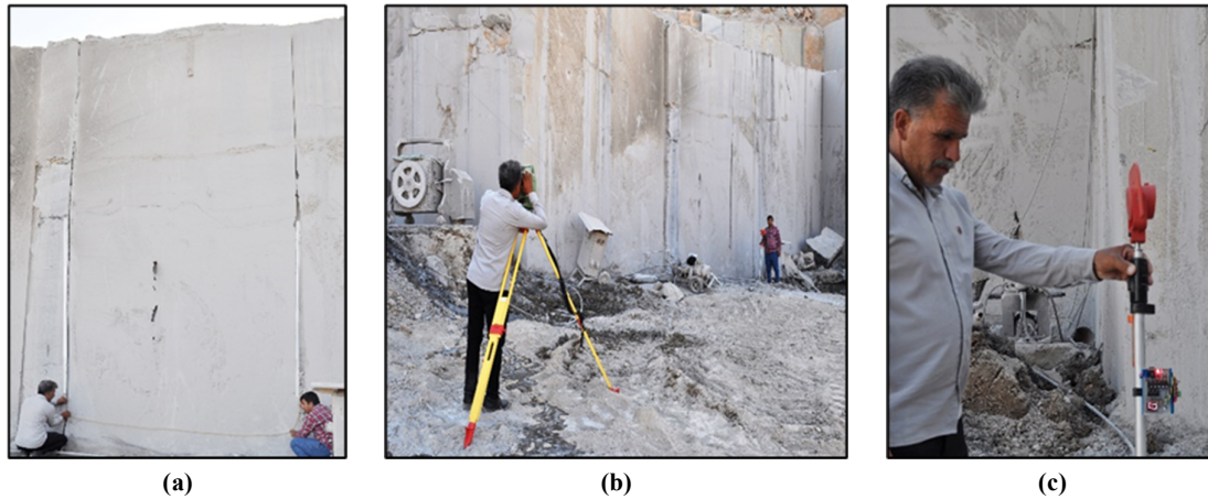
Figure 7. (a) leveling hose, (b) theodolite, and (c) using LTS for spot-finding.
