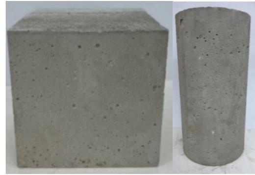
Figure 4. Cubic (10×10×10 cm) and cylindrical (15×30 cm) samples
