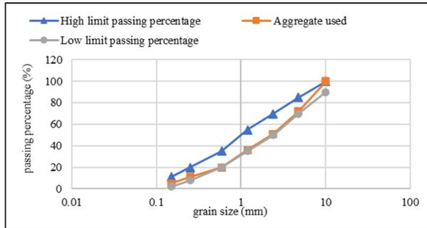
Figure 1. Granulation diagram of the used sand
