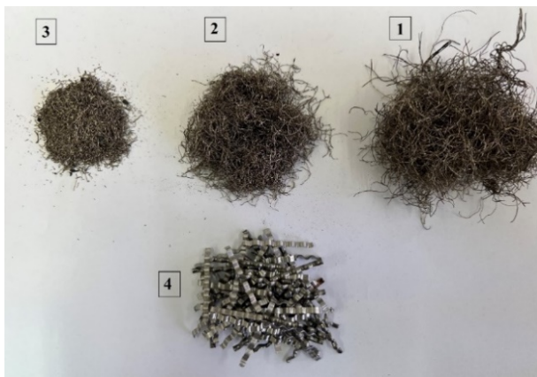
Figure 2. Types of fibers used in tests: 1- Coarse recycled steel fibers, 2- Medium recycled steel fibers, 3- Fine recycled steel fibers, and 4- Industrial steel fibers
