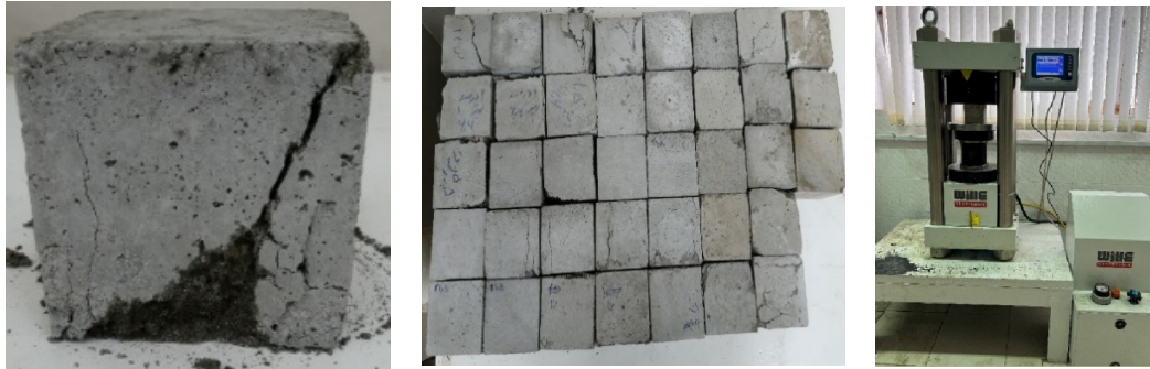
Figure 5. Several samples tested for compressive strength and uniaxial compressive testing machine.
