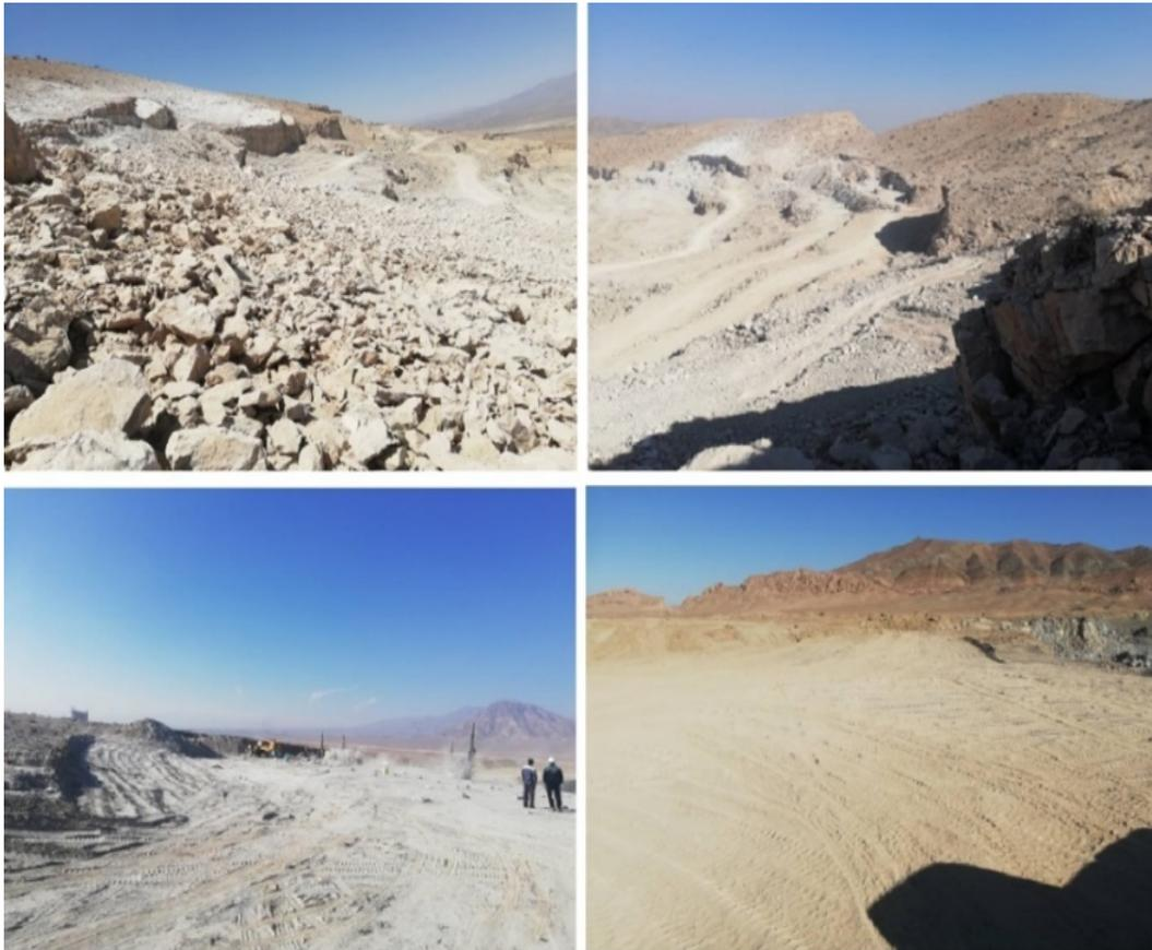
**Figure 5. Post-Blast Condition Using the Power Deck Method in Nizar Mine, Qom, Iran**
