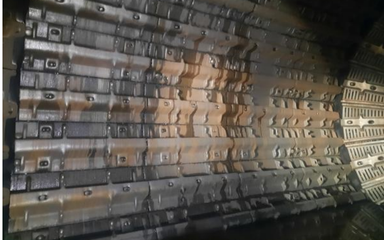
Figure 10. A view of the new liners after 500 hours of operation
