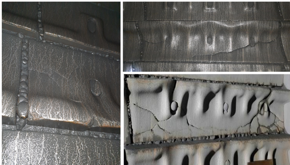
Figure 1. Broken liners in the SAG mill
