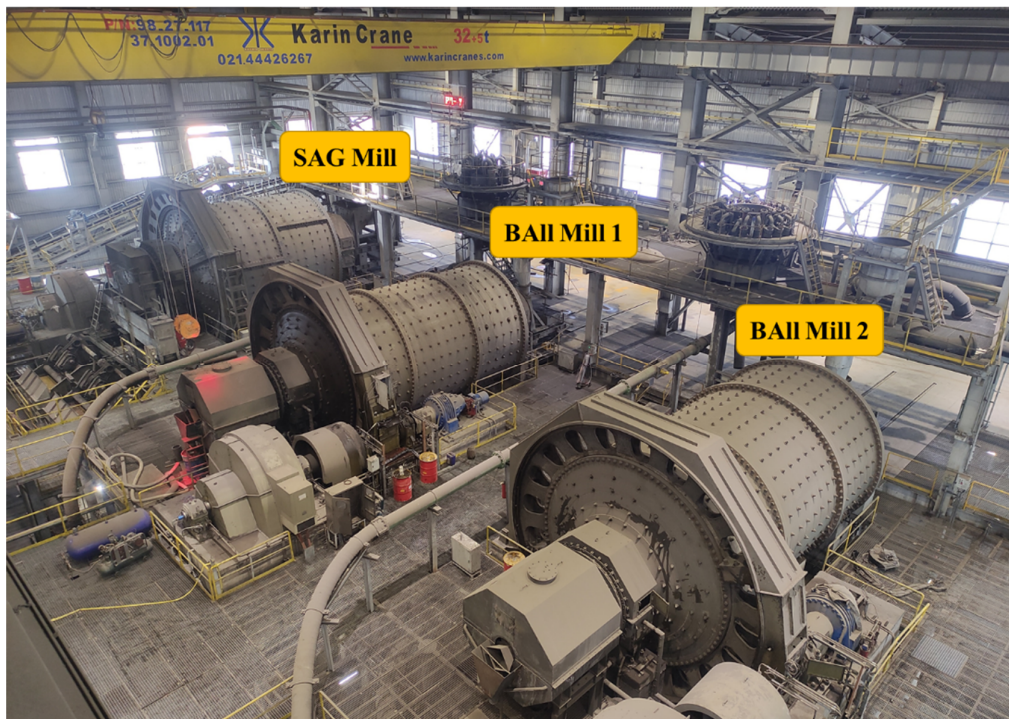
Figure 1. Grinding circuit of the slag flotation plant at the Sarcheshmeh copper complex
