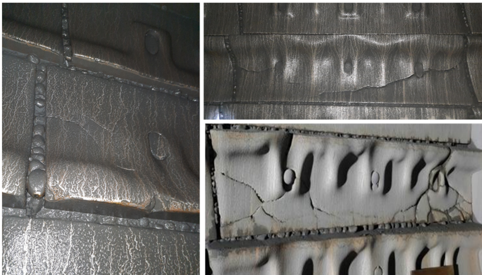
Figure 1. Broken liners in the SAG mill
