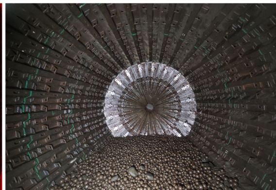
Figure 9. The layout of the proposed liners in SolidWorks software (a) and installed liners in the SAG mill (b).
