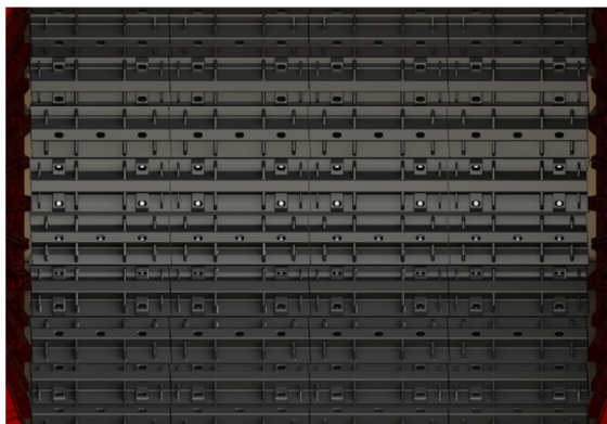
Figure 9. The layout of the proposed liners in SolidWorks software (a) and installed liners in the SAG mill (b).
