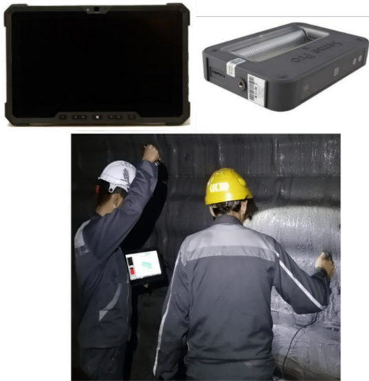
Figure 4. Scanning using the Sence Pro scanner connected to the Latitude 12 Rugged handheld computer.
