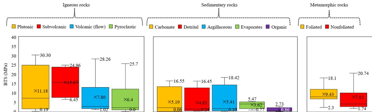
Figure 3. Average and range of BTS values for rock types (According to rock classification given in Table 7)
