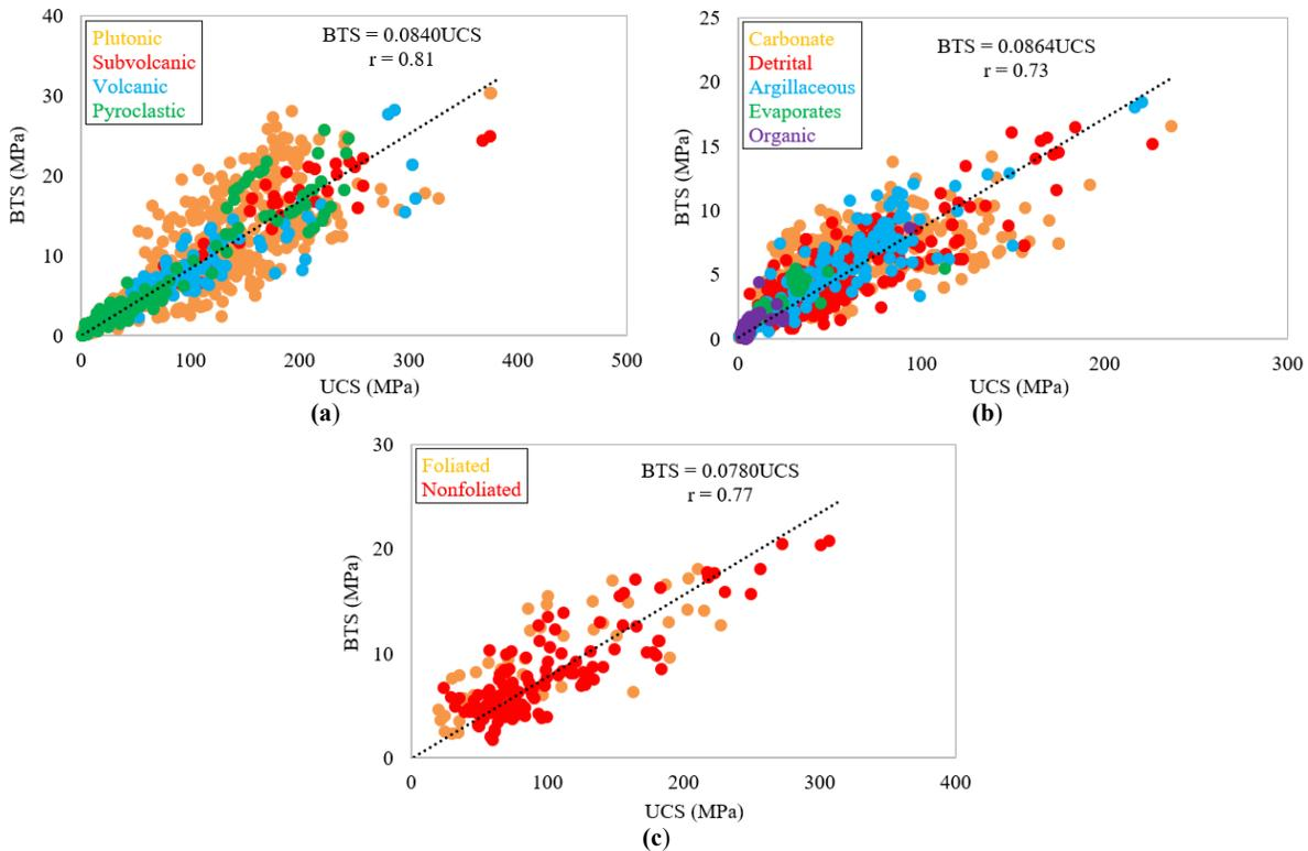
**Figure 5. Relationship between BTS and UCS for (a) igneous rocks, (b) sedimentary rocks, and (c) metamorphic rock**
