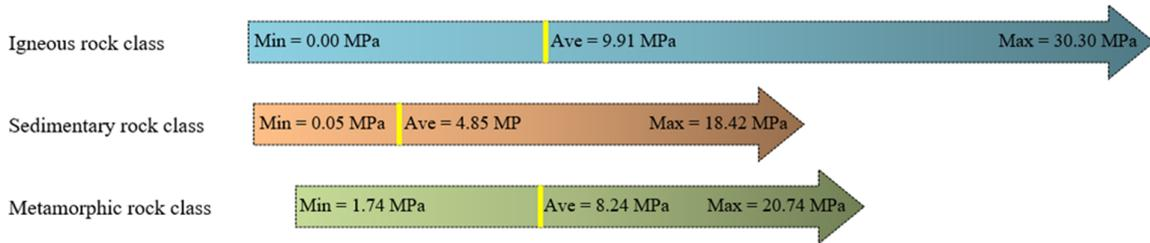
**Figure 4. Comparison of BTS values (minimum, maximum, average) of the igneous, sedimentary, and metamorphic rocks**
