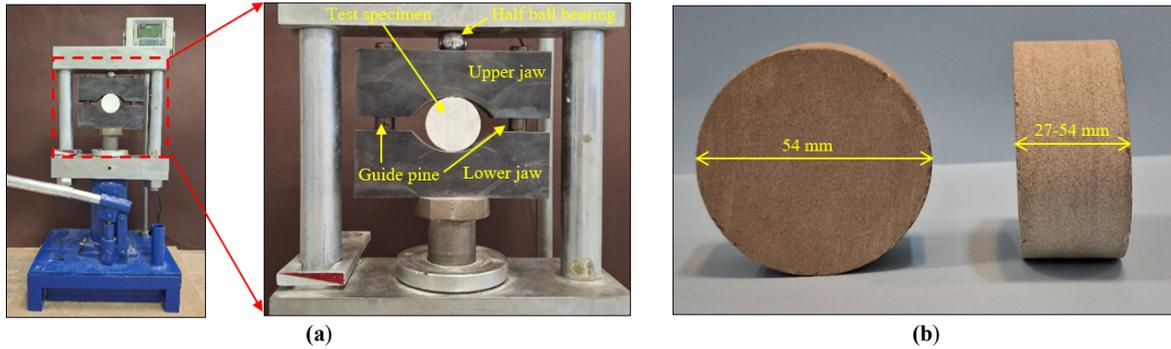
Figure 1. a) The ISRM [24] suggested apparatus for BTS test, and b) disk-shaped rock specimen
