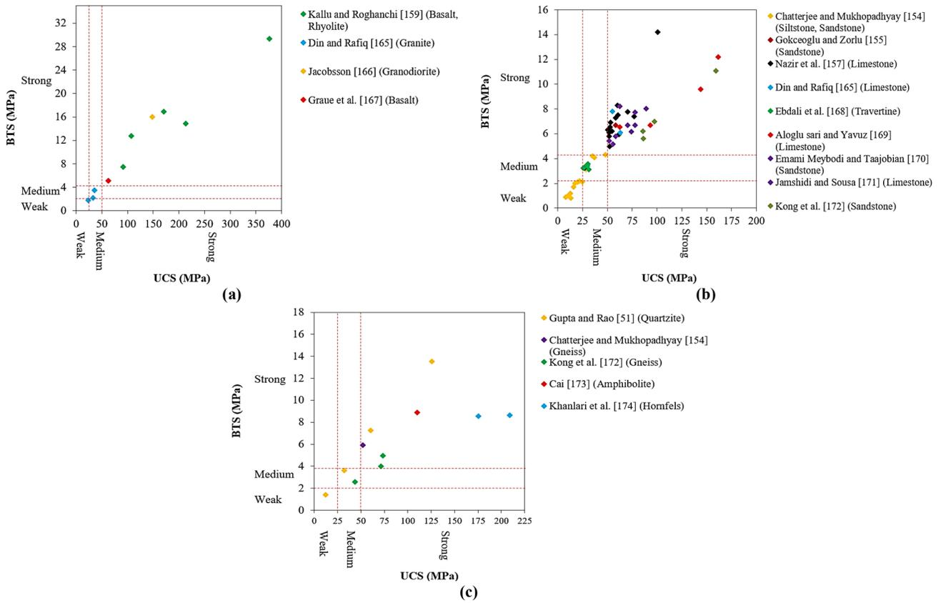
Figure 8. The validity of BTS classification by data published by various researchers a) Igneous rocks b) sedimentary rocks, and c) metamorphic rocks
