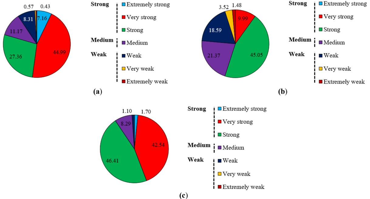
Figure 9. The frequency of BTS classes (a) igneous rocks, (b) sedimentary rocks, and (c) metamorphic rocks
