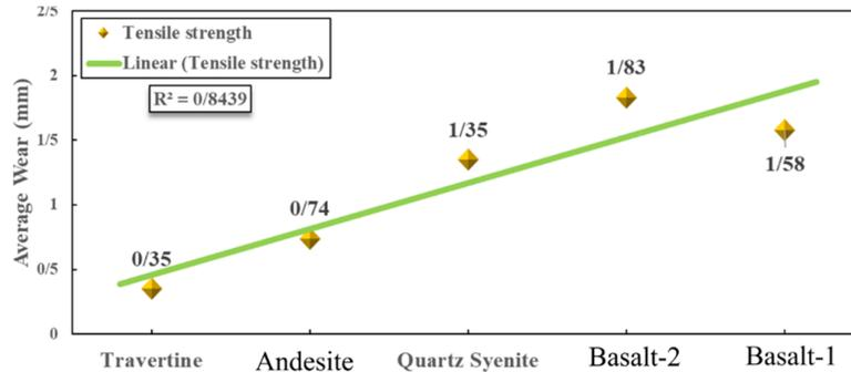
Figure 9. Changes in disc cutter wear according to Brazilian tensile strength in 5 different rock samples.
