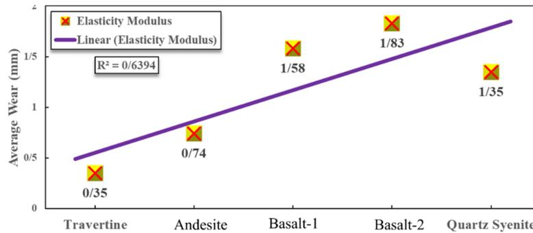
Figure 11. Changes in the wear of the disc cutter according to the values of the modulus of elasticity in 5 different rock samples.
