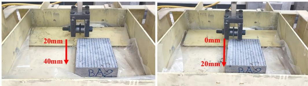
Figure 6. The steps of performing the LCM test.
