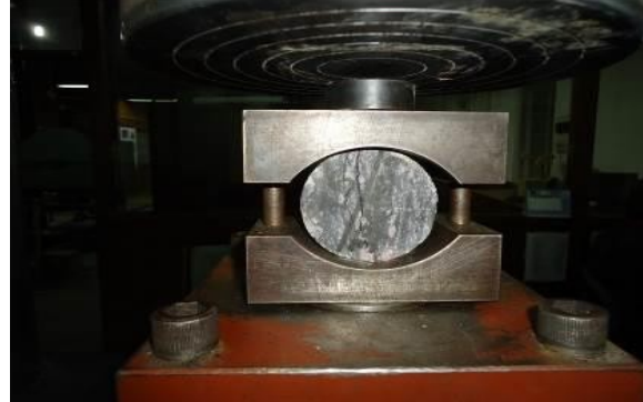
Figure 4. Tensile strength testing using Brazilian test
