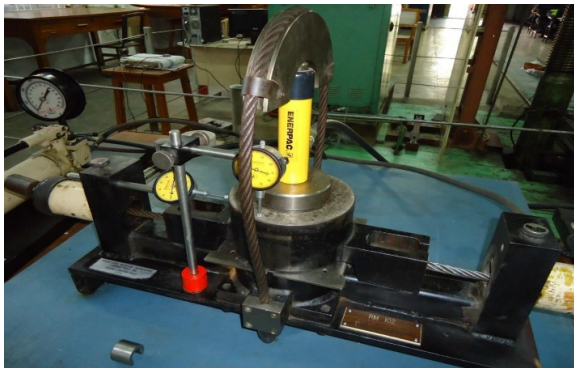
Figure 5. Test setup for laboratory determination of direct shear strength of rock specimens
