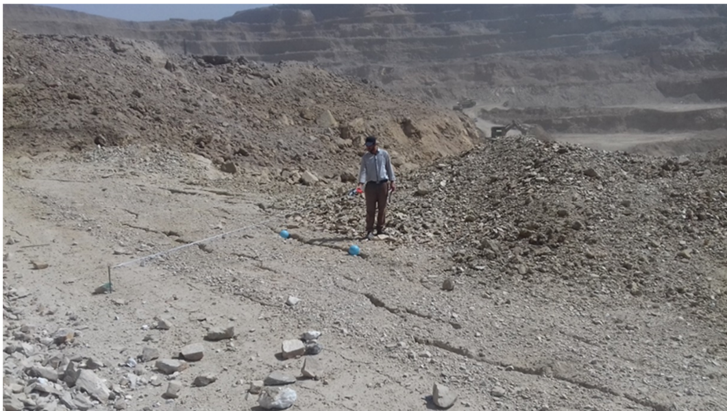
Figure 1. Back-break that resulted from blasting operations at Gol-e-Gohar Mine No. 1
